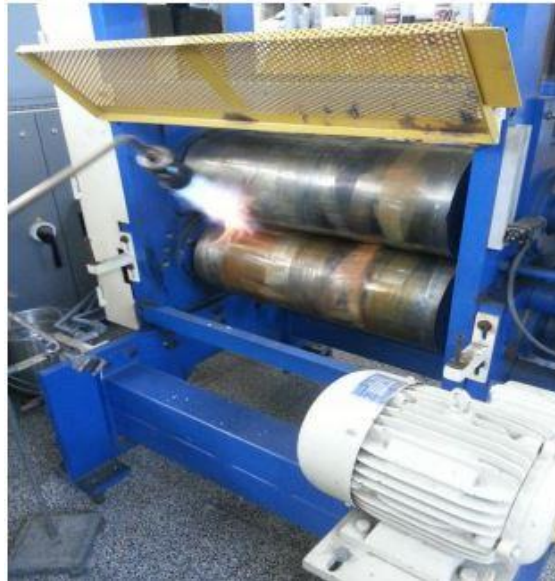
Figure 22. Rolling device used to reduce section thickness of slabs
