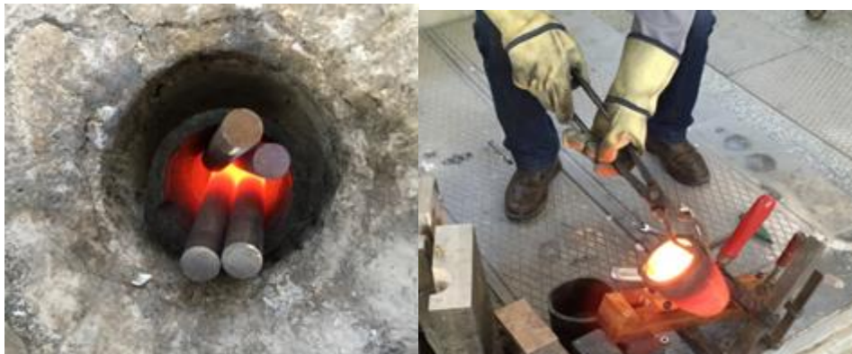
Figure 19. Melting with induction furnace and Casting into mold
