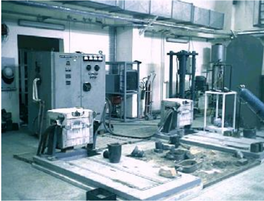
Figure 18. Induction furnaces used in this study
