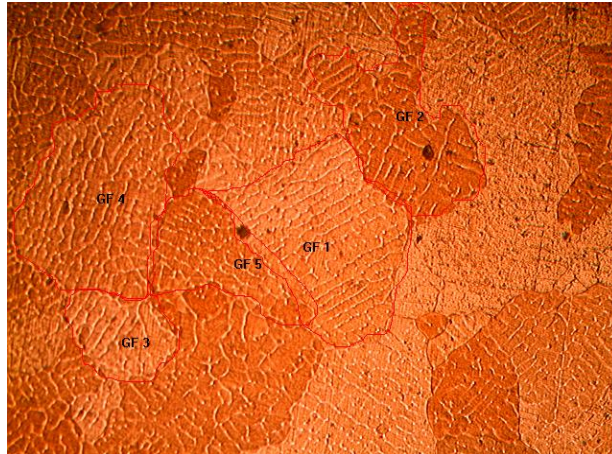
Figure 29. Cast microstructure of CuNiSi alloy
