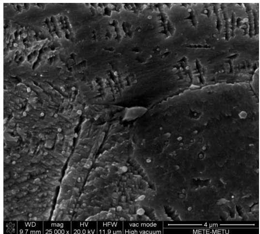
Figure 92. SEM images of 100min annealed, 30min aged sample
