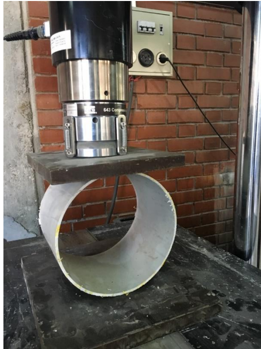
Figure 3.3. Parallel Plate Test Setup
