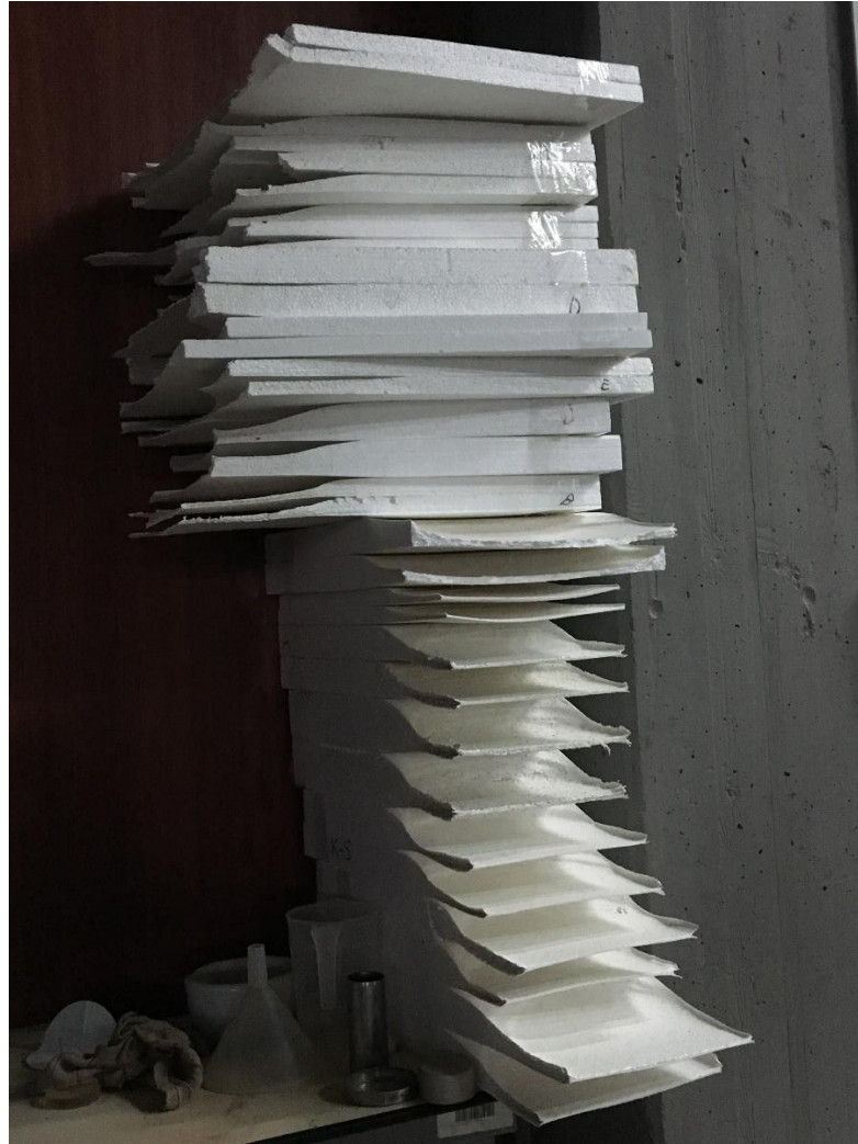
Figure 6.1. Geofoms are cut to measure final strain %
