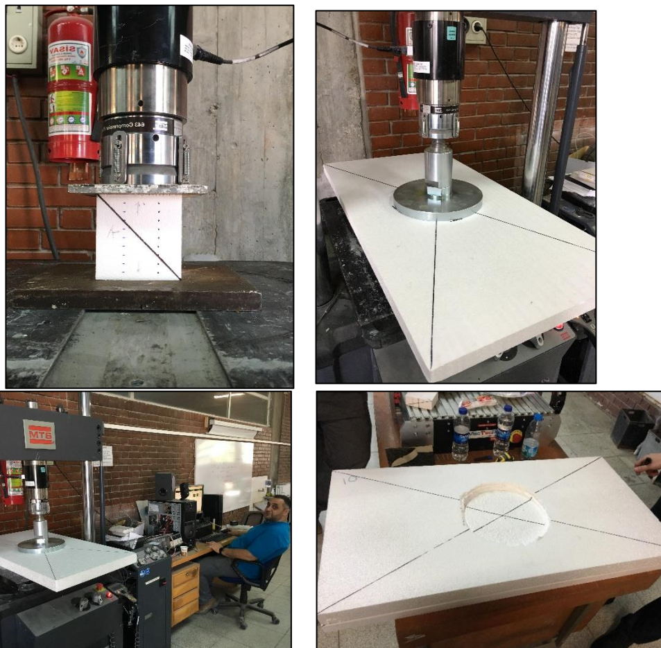
Figure 3.9. Geoforce Loading Experiments in Material Lab
