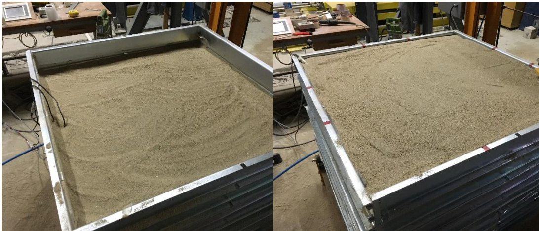
Figure 4.9. Last two compressed soil layers after geofoam placement
