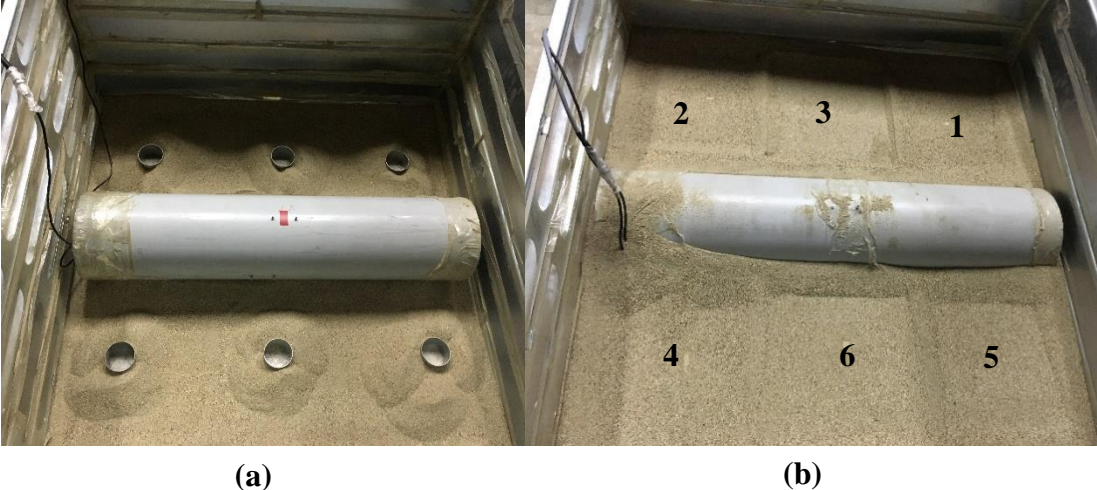
Figure 4.7. Installation of density boxes (a) & compaction order in pipe layer (b)
