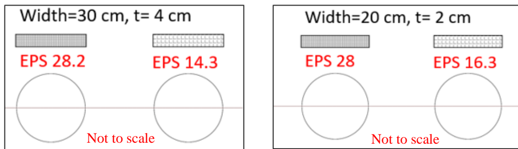
Figure 5.6. Four tests conducted to investigate the effect of geofom density
