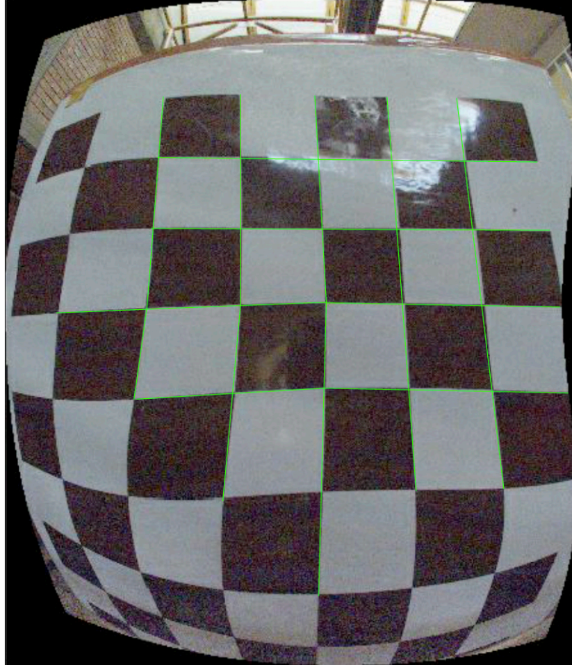
Figure 3-8 Undistorted image obtained by using equations (2.28), (2.29) and (2.30) with the parameters estimated by PSO
