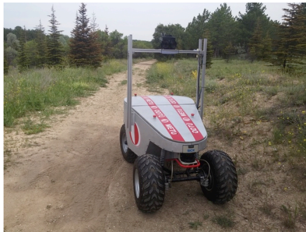
Figure 2-1 Picture of UGV platform, GOAT
