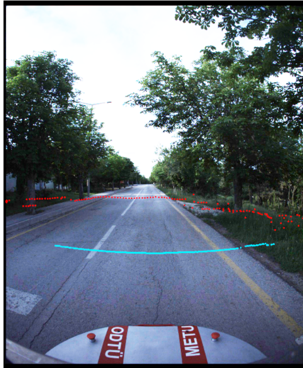
Figure 2-4 Example LIDAR readings taken by the sensors mounted to the front surface, red points measured by SICK and blue points measured by Hokuyo
