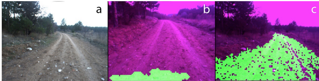
Figure 1-4 Steps of road detection algorithm proposed in [18], a) raw image of the environment, b) training image for the long range road detection algorithm, where green pixels shows the close range road area found by using surface roughness, c) output of the long range road detection algorithm, where green pixels shows the road region
