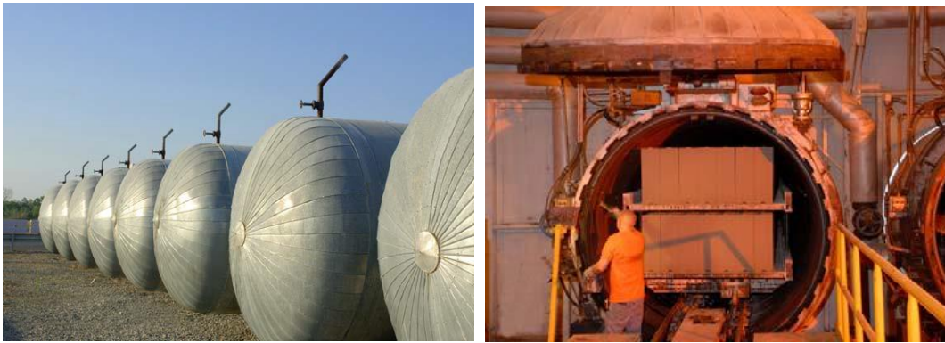
Figure 1.6: Exterior and Interior Views of Autoclaves (Xella, 2010)
