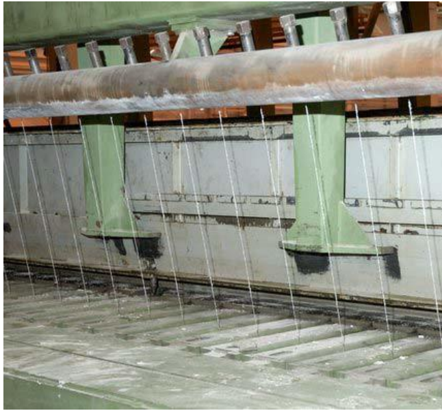
Figure 1.5: Cutting Machine with Steel Wires (Xella, 2010)
