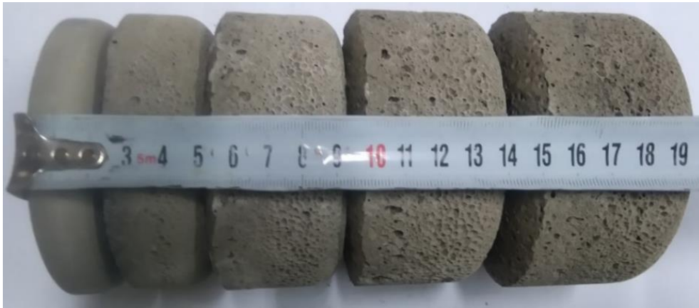
Figure 4.4 Effect of hydrogen peroxide content on expansion of pastes with identical mass (~240 g) and W/S=0.425 (from left to right, hydrogen peroxide contents 0 %, 0.25 %, 0.50 %, 0.75 %, 1.50 %, the scale bar shows cm units).
