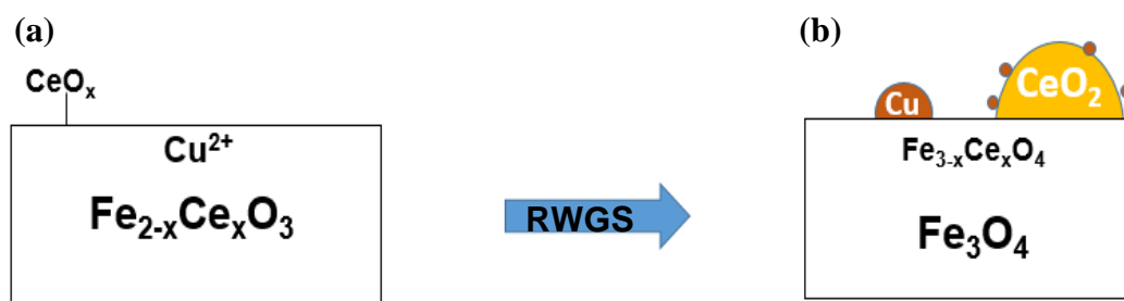
Figure 6.17. Schematic of the 3Cu/8CeFe catalyst (a) calcined and (b) during HT-WGSR
