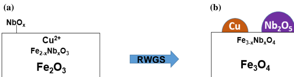
Figure 6.12. Schematic of the supported 3Cu/8NbFe catalyst (a) calcined and (b) during HT-WGS
