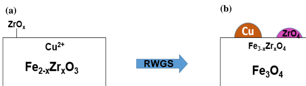
Figure 6.7. Schematic of the supported 3Cu/8ZrFe catalyst (a) calcined and (b) during HT-WGS
