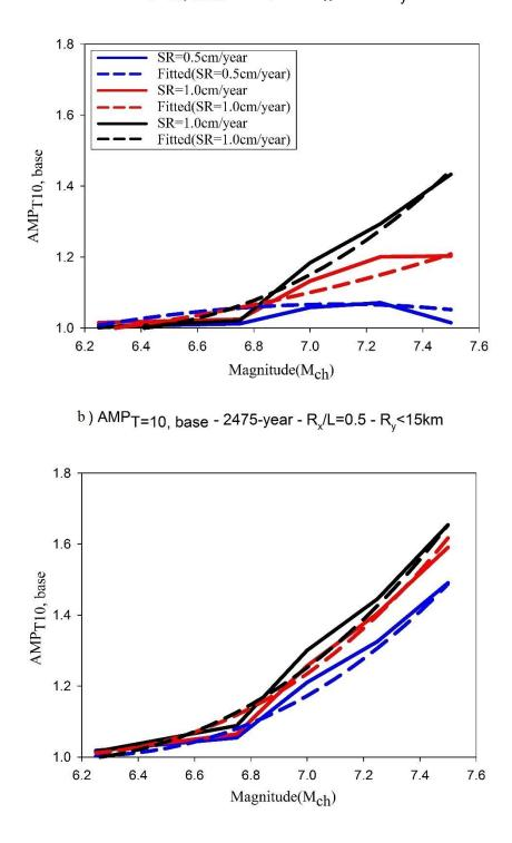
Figure 5.15 SHB11-based directivity amplification vs  $M_{ch}$  relationship together with cubic fits calculated for the sites 3, 9, 15 and 21 at T = 10s a) 475-year return period b) 2475-year return period
