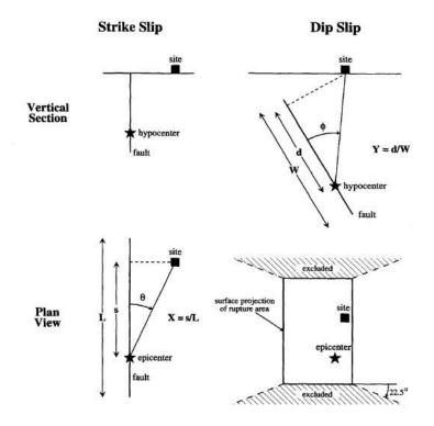
Figure 2.5 Geometric parameters used in Somerville (1997) directivity model.
