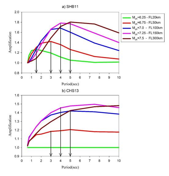
Figure 5.11 Median SHB11 and CHS13 directivity amplifications in terms of M<sub>ch</sub>
