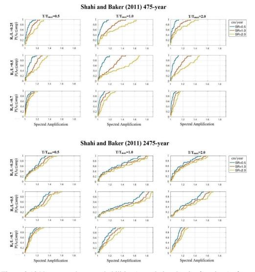
Figure 3.10 Non-exceedance probabilities (cumulative density functions) of directivity spectral amplifications according to Shahi and Baker (2011) directivity model given a range of  $R_x/L$ ,  $T/T_{max}$  and average slip rate. First three rows show the probabilities for the 475-year return period. The last three rows pertain to the 2475-year return period probabilities
