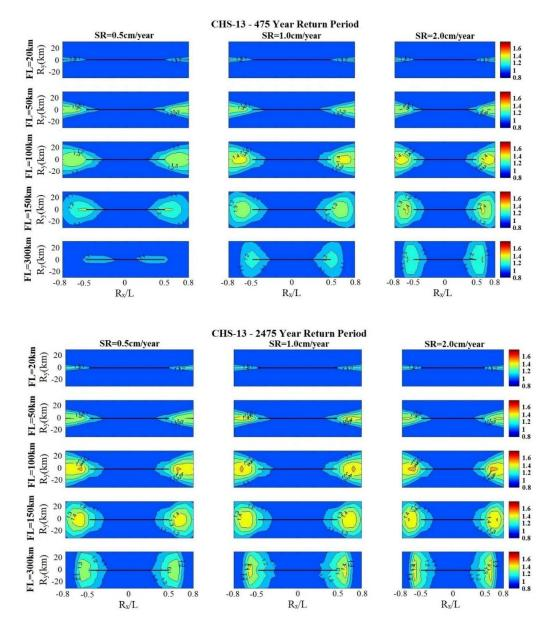
Figure 3.14 The spatial distribution of the forward-directivity spectral amplifications by CHS13 in terms of the return period, slip rate and the fault length (thus the characteristic earthquake magnitude)
