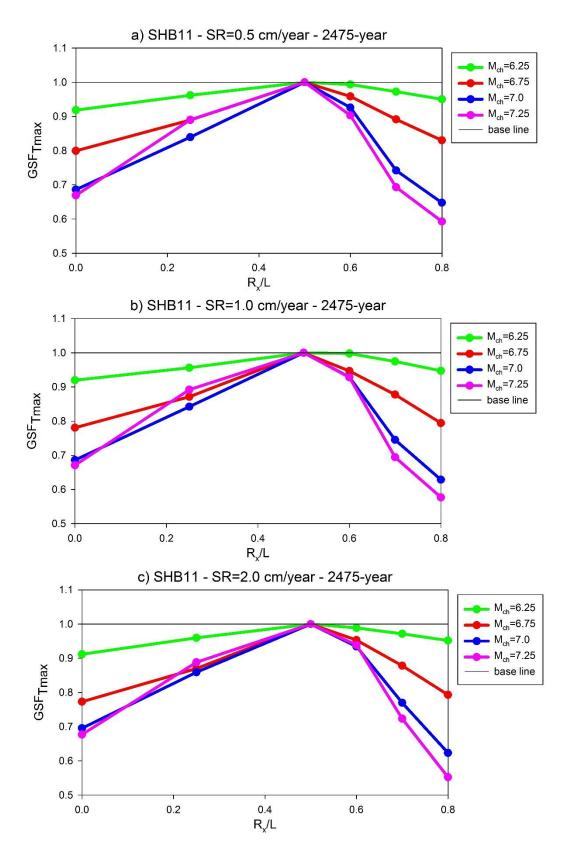
Figure 5.17 Observed geometric scale factors for AMP<sub>Tmax</sub> - 2475-year return period and  $\dot{s} = 0.5$  cm/year,  $\dot{s} = 1.0$  cm/year and  $\dot{s} = 2.0$  cm/year (SHB11)
