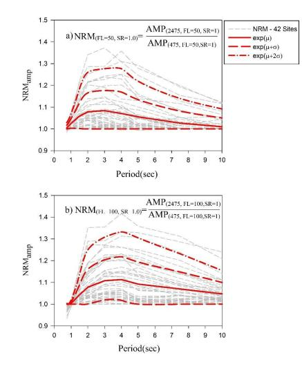
Figure 5.6 Normalized period-dependent 2475-year to 475-year directivity dominant spectral amplification ratios of 42 sites (grey curves) and corresponding logarithmic mean,  $\pm$ sigma as well as 2sigma over logarithmic mean a) fictitious fault with 50km length and  $\dot{s} = 1$  cm/year b) fictitious fault with 100km length and  $\dot{s} = 1$  cm/year
