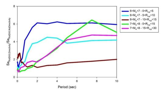
Figure 4.13 Median Sa<sub>RotD50directivity</sub> to Sa<sub>RotD50nodirectivity</sub> ratios computed by normalizing the median Sa<sub>RotD50directivity</sub> spectrum of each pulse-like groundmotion bin in Table 4.2 with the corresponding median Sa<sub>RotD50nodirectivity</sub> spectrum of non-pulse ground-motion bin
