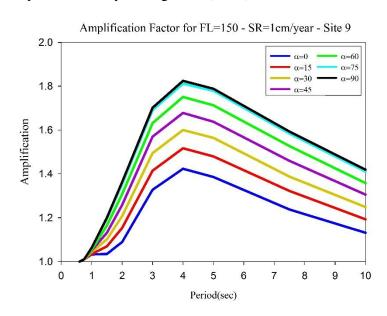
Figure 3.8 Variation of forward-directivity spectral amplifications as a function of  $\alpha$  (alpha) at Site 9 for the fictitious PSHA scenario considered in Figure 3.6.
