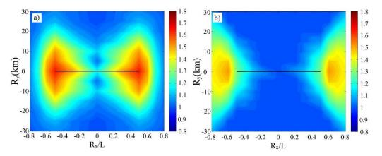
Figure 3.9 475-year probabilistic spectral amplifications for forward-directivity computed by (a) SHB11 and (b) CHS13 (via CY14) for a fault length of L = 100km and  $\dot{s} = 2$ cm/year
