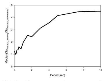
Figure 4.14 Median of Sa<sub>RotD100directivity</sub> to Sa<sub>RotD100nodirectivity</sub> ratios presented in Figure 4.10
