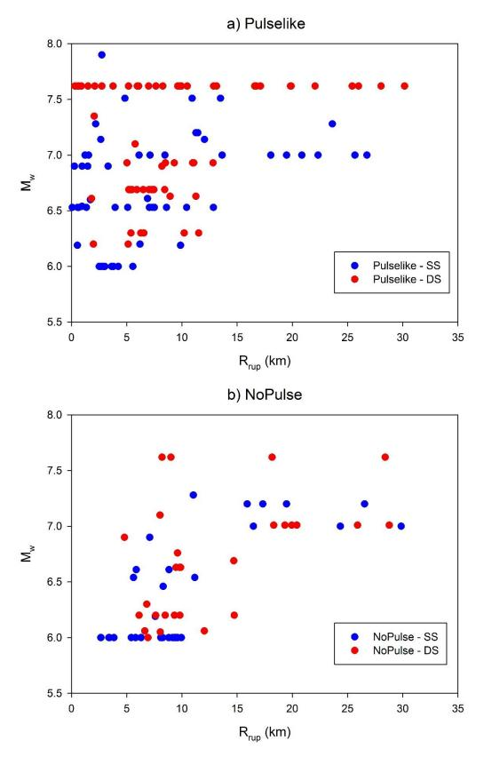
Figure 4.2 Magnitude versus distance distribution of (a) pulselike and (b) non-pulse ground motions for different styles of faults (dip-slip and strike-slip) 72
