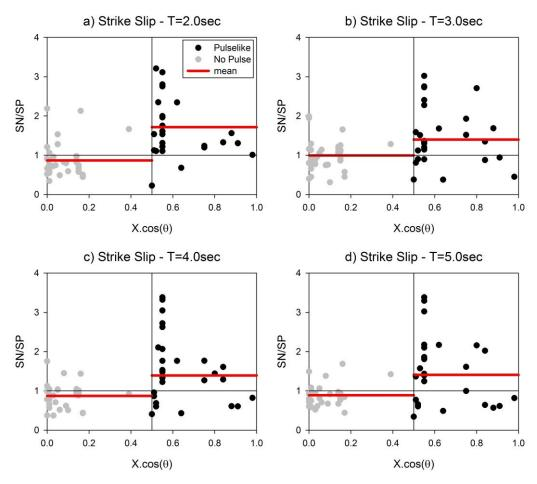
Figure 4.5 Comparisons of SN/SP spectral ratios at T = 2s, 3s, 4s and 5s by considering the  $Xcos(\theta) = 0.5$  criterion as the boundary between pulselike and non-pulse strike-slip recordings. The red solid lines show the average of pulselike and non-pulse SN/SP ratios.
