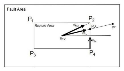
Figure A.4 Calculation of direct point for the case that closest point is located outside the rupture area
