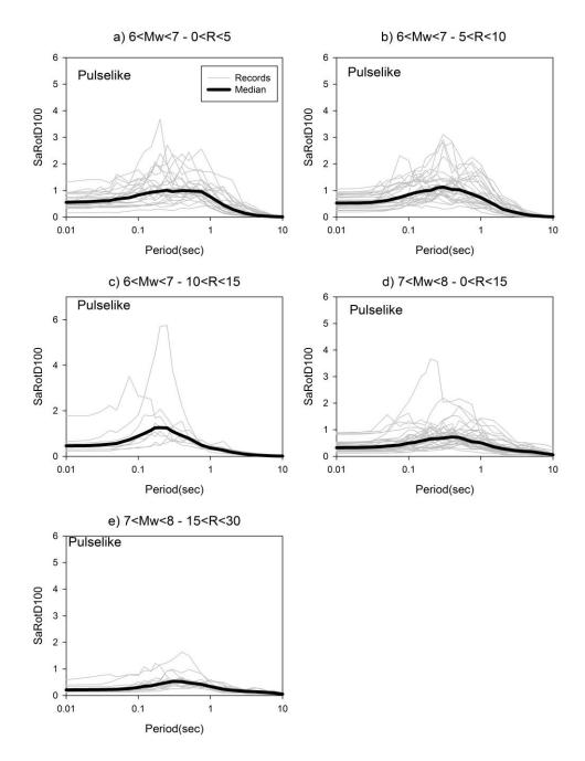
Figure 4.8 Sa<sub>RotD100directivity</sub> (from pulselike records) spectral amplitudes of individual ground motions of the bins given in Table 4.2
