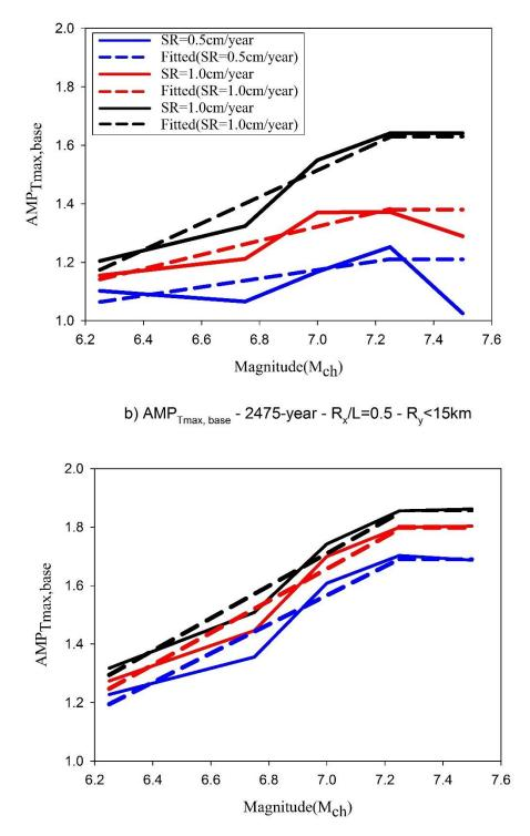
Figure 5.13 SHB11-based directivity amplification vs  $M_{ch}$  relationship together with linear fits calculated for the sites 3, 9, 15 and 21 at spectral period  $T_{max}$  a) 475-year return period b) 2475-year return period
