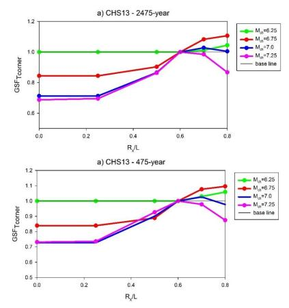
Figure 5.23 Calculation of Geometric Scale Factor for AMP<sub>Tcorner</sub> - 475-year CHS13
