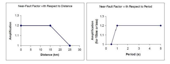
Figure 2.7 Near-Fault adjustment factor as a function of distance and spectral period (CALTRANS 2013).
