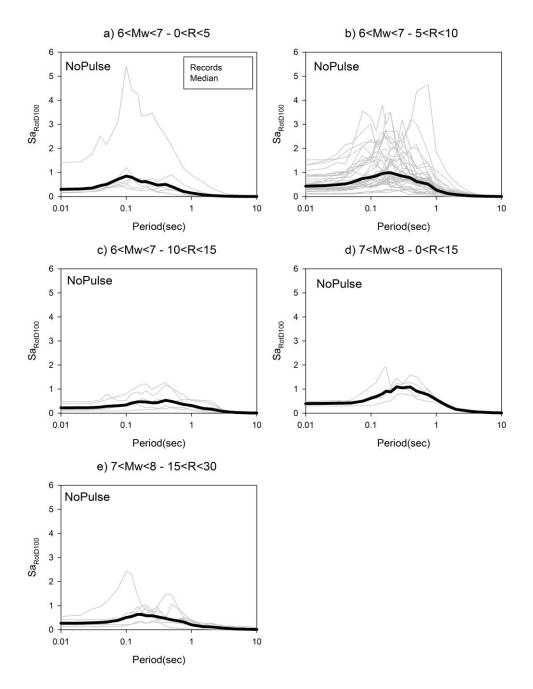
Figure 4.9 Sa<sub>RotD100nodirectiviy</sub> (from non-pulse records) spectral amplitudes of individual ground motions of the bins given in Table 4.2
