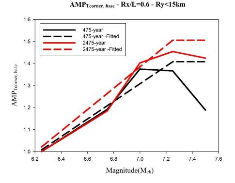
Figure 5.22 Base amplification factors and magnitude relationships together with linear line fits calculated for sites 4, 10, 16 and 22 at spectral period T<sub>corner</sub> - CHS13 model, 475- and 2475-year return period
