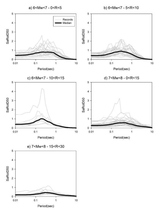
Figure 4.11 Sa<sub>RotD50directivity</sub> (from pulselike records) spectral amplitudes of individual ground motions of the bins given in Table 4.2. The solid black lines are the log-mean (median) spectral curves of each bin.
