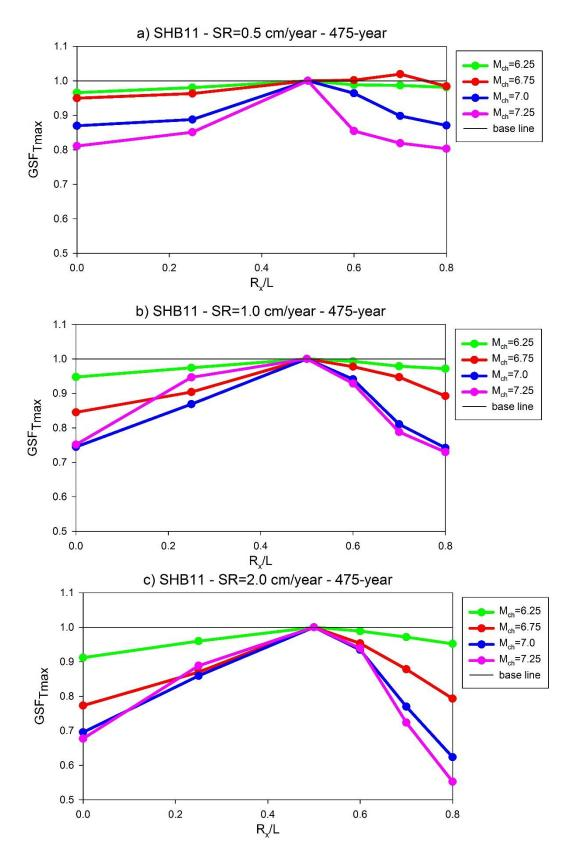
Figure 5.16 Observed geometric scale factors for AMP<sub>Tmax</sub> - 475-year return period and  $\dot{s} = 0.5$  cm/year,  $\dot{s} = 1.0$  cm/year and  $\dot{s} = 2.0$  cm/year (SHB11)
