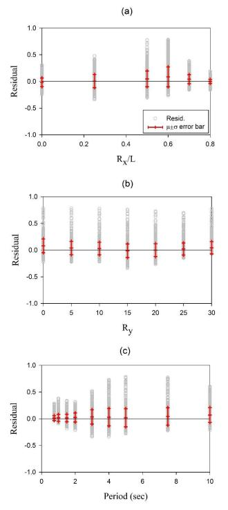
Figure 5.29 Residuals computed from PSHA (observed) and estimated directivity amplifications for SHB11 narrow-band directivity model for the 2475-year return period
