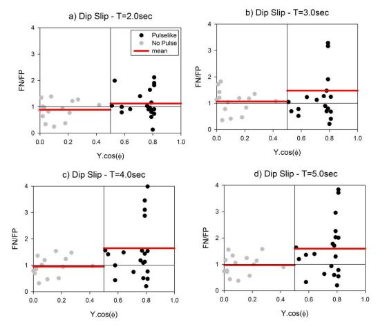
Figure 4.6 Comparisons of SN/SP spectral ratios at T = 2s, 3s, 4s and 5s by considering the  $Ycos(\phi) = 0.5$  criterion as the boundary between pulselike and non-pulse dip-slip recordings. The red solid lines show the average of pulselike and non-pulse SN/SP ratios.
