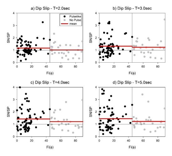
Figure 4.4 Comparisons of SN/SP spectral ratios at T = 2s, 3s, 4s and 5s by considering the  $\phi = 45^{\circ}$  criterion as the boundary between pulselike and non-pulse dip-slip recordings. The red solid lines show the average of pulselike and non-pulse SN/SP ratios.
