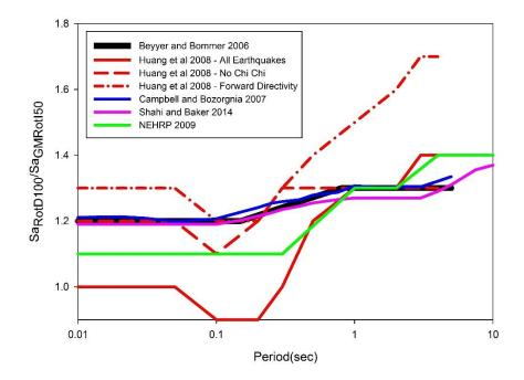
Figure 4.7 Comparison of different scaling (conversion) models proposed for Sa<sub>RotD100</sub>/Sa<sub>GMRotI50</sub> ratio
