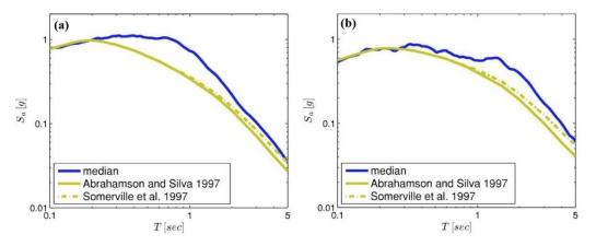
Figure 2.3 Response spectrum of pulse-type records with a)  $0.6 \le T_p < 1.5$  (mean  $T_p=1.0s$ ) and b)  $1.5 \le T_p < 2.5$  (mean  $T_p=1.9s$ ). The plots also show the response spectrum computed from conventional Abrahamson and Silva (1997) GMPE and the braod-band model by Somerville et al. (1997) (Tothong et al. 2007)
