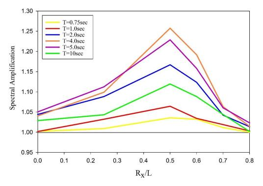
Figure 5.2 Bilinear trend for directivity-dominated spectral amplifications along fault strike,  $R_x/L$ , direction for a suit of spectral periods (FL = 100km,  $\dot{s}$  = 1.0cm/year,  $R_y$ =15km)
