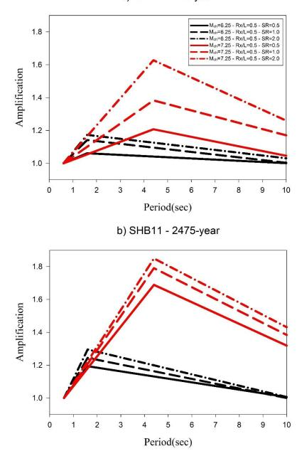
Figure 5.20 Effect of characteristic magnitude and slip rate on the directivity amplifications for SHB11 model computed from proposed simplified expressions a) 475-year return period b) 2475-year return period
