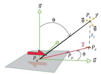
Figure A.5 Geometrical information for the calculation of average scalar radiation pattern ( $\overline{FS}$ ) parameter (Spudich et al. 2013)
