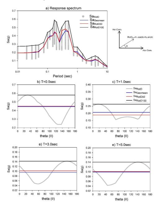
Figure 2.8 Response spectrum of Gebze station-1999 Kocaeli earthquake calculated for different rotated orientations of two horizontal components, together with geometric mean, RotD50 and RotD100 components illustrated for different spectral periods
