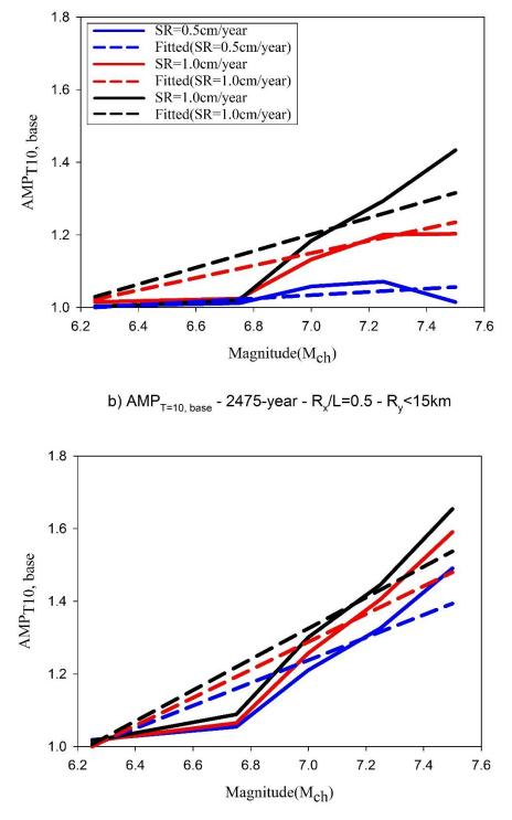
Figure 5.14 SHB11-based directivity amplification vs  $M_{ch}$  relationship together with linear fits calculated for the sites 3, 9, 15 and 21 at T = 10s a) 475-year return period b) 2475-year return period
