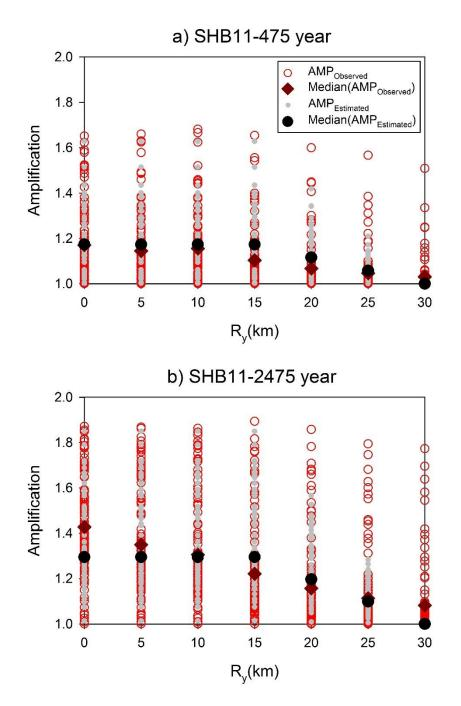
Figure 5.26 Observed ad estimated directivity amplifications as a function of R<sub>y</sub> for simplified SHB11 model
