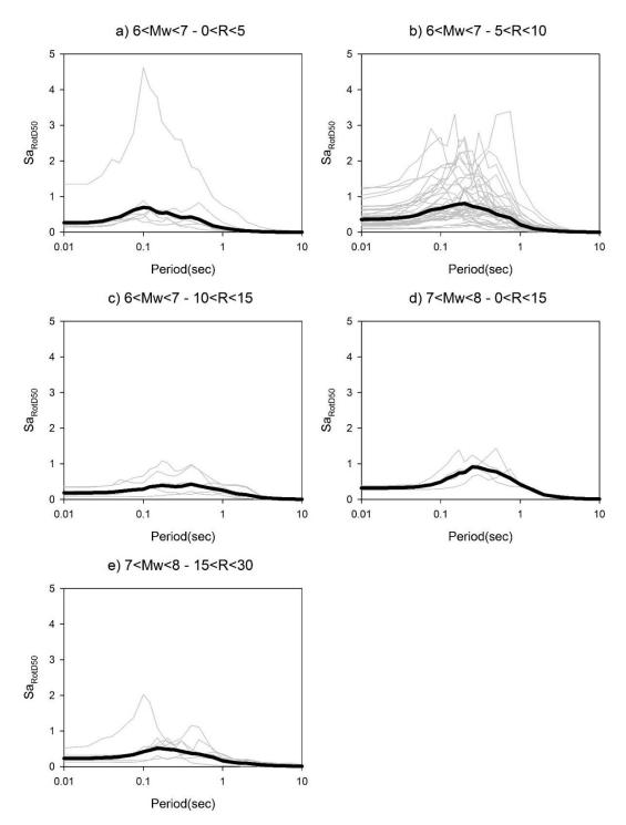
Figure 4.12 Sa<sub>RotD50nodirectiviy</sub> (from non-pulse records) spectral amplitudes of individual ground motions of the bins given in Table 4.2. The solid black lines are the log-mean (median) spectral curves of each bin
