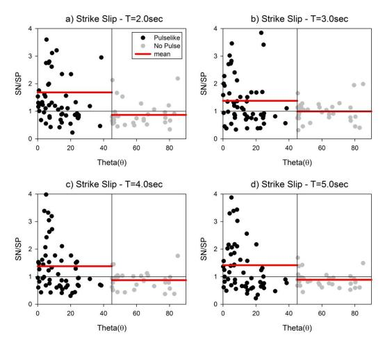
Figure 4.3 Comparisons of SN/SP spectral ratios at T = 2s, 3s, 4s and 5s by considering the  $\theta = 45^{\circ}$  criterion as the boundary between pulselike and non-pulse strike-slip recordings. The red solid lines show the average of pulselike and non-pulse SN/SP ratios.
