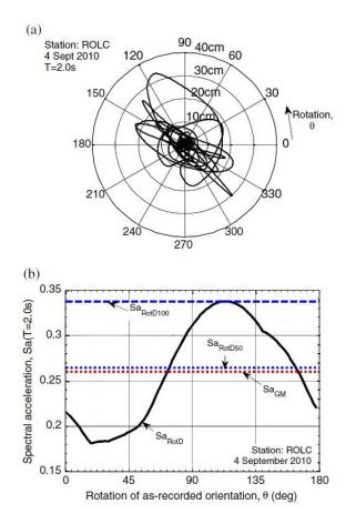
Figure 4.1 (a) Illustration of polarization by plotting the displacement response of horizontal components at T = 2s for at the Rolleston station from the 24 September 2010 M<sub>w</sub>7.1 Darfield earthquake), (b) Sa values at T = 2.0s obtained by rotating the horizontal ground-motion components at  $0^{\circ} \le \theta \le 179^{\circ}$  (Bradley and Baker 2015)
