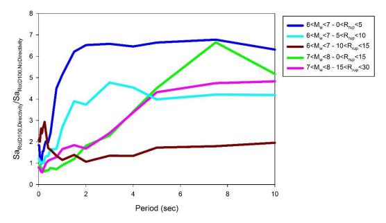
Figure 4.10  $AF_{directivity}$  curves computed from median  $Sa_{RotD100directivity}$  to  $Sa_{RotD100nodirectivity}$  ratios of the ground-motion bins presented in Table 4.2
