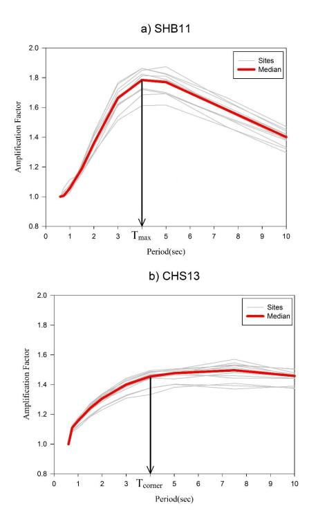
Figure 5.10  $T_{max}$  and  $T_{corner}$  values for directivity amplifications. The earthquake scenario is FL=150km (M<sub>ch</sub>=7.25),  $\dot{s} = 0.5$ cm/year, 1cm/year, 2 cm/year a) SHB11 model b) CHS13 model
