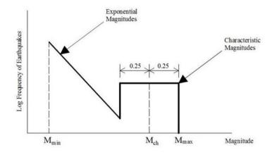
Figure 3.7 The Youngs and Coppersmith (1985) stochastic model to describe the earthquake recurrence in PSHA runs. The minimum magnitude, M<sub>min</sub>, is always considered as M<sub>w</sub> 5 in the probabilistic earthquake scenarios. The characteristic magnitude, M<sub>ch</sub>, is determined from the mean M<sub>w</sub> estimated from the empirical M<sub>w</sub> vs. RA relationship in (Wells and Coppersmith 1994).
