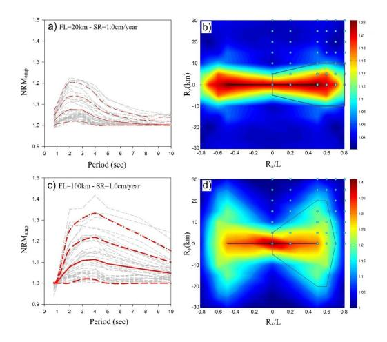
Figure 5.7 Comparison of NRM<sub>amp</sub> and the related contour maps for classification of the sites a) NRM<sub>amp</sub> vs T(sec) for FL=20km, S=1cm/year b) contour map of NRM<sub>amp</sub> for T=2.0sec FL=20km, S=1cm/year c) NRM<sub>amp</sub> vs T(sec) for FL=100km, S=1cm/year d) contour map of NRM<sub>amp</sub> for T=4.0sec FL=100km, S=1cm/year
