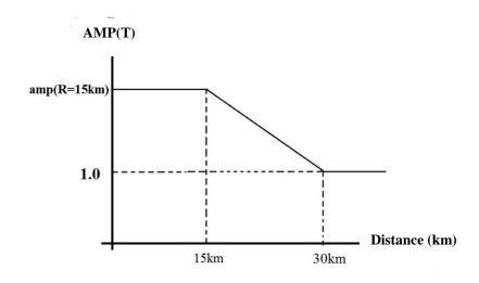
Figure 5.25 Distance Tapering of Directivity Amplification Factor
