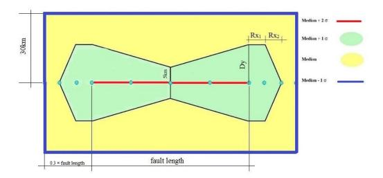
Figure 5.8 Classification of the area around the fault into four regions with respect to NRM<sub>amp</sub>(T) intensities
