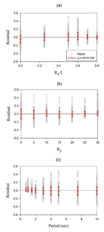
Figure 5.28 Residuals computed from PSHA (observed) and estimated directivity amplifications for SHB11 narrow-band directivity model, for the 475-year return period
