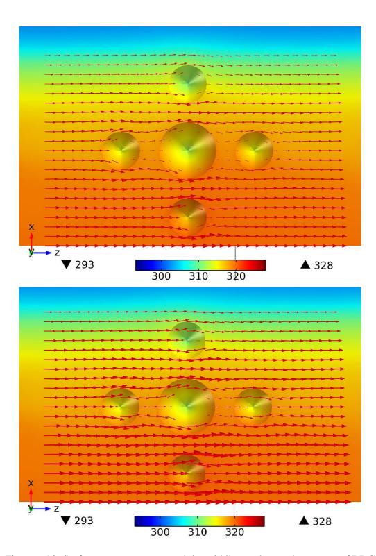
Figure 6.93: Surface temperature around the middle roughness element set of RDC configuration and convective het flux in the fluid at  $y = 5 \mu m$  plane (top) and  $y = 7.5 \mu m$  plane (bottom) for  $G = 1016 \text{ kg/(m^2s)}$ .
