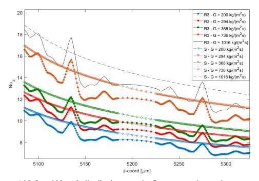
Figure 6.95: Local Nusselt distribution over the first two roughness element sets of RDC configuration.
