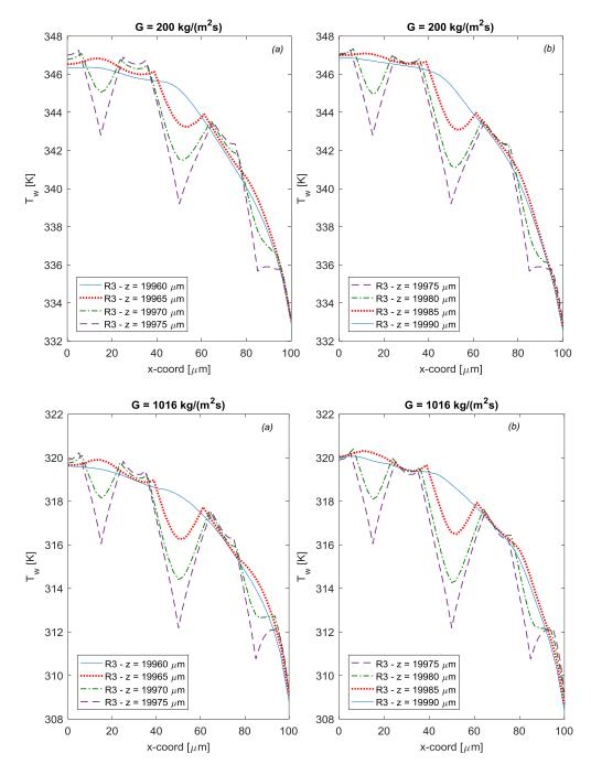
Figure 6.86: Wall temperature distribution around the bigger cone of middle roughness element set of RDC configuration for inlet mass fluxes of 200 kg/( $m^2s$ ) and 1016 kg/( $m^2s$ ) for (a) flow facing side of the cone, (b) back side of the cone.
