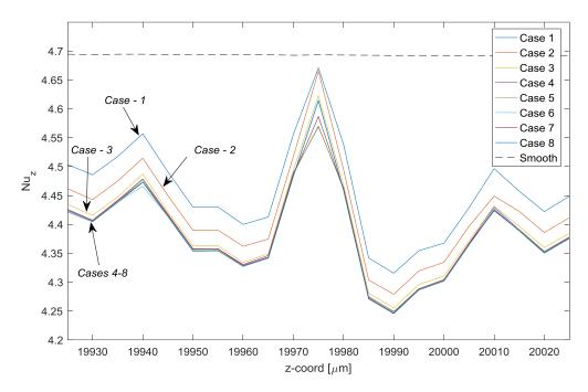
Figure 6.78: Local Nusselt distribution for mesh independence test cases of RDC configuration around the middle roughness element set.
