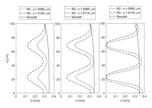
Figure 6.52: Velocity magnitude profiles along *x*-direction at  $y = 5 \mu m$  and various *z* locations for the first conical element of R2LC configuration.
