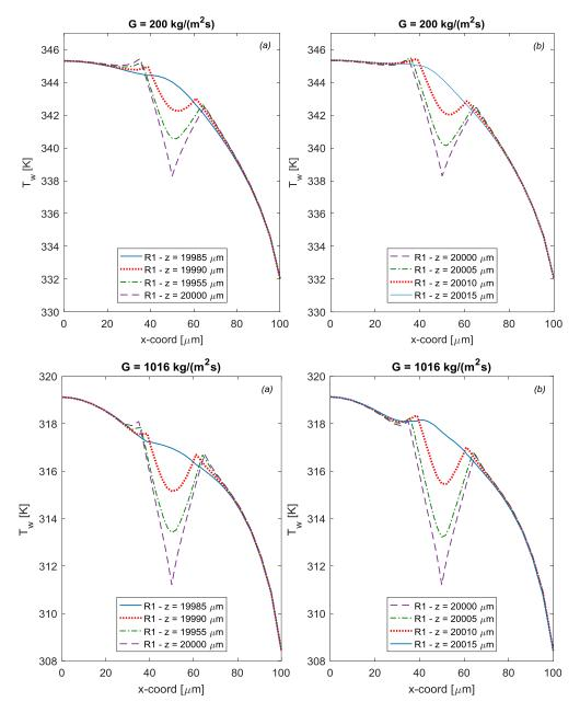
Figure 6.27: Wall temperature distribution around the middle cone of R1LC configuration for inlet mass fluxes of 200 kg/( $m^2s$ ) and 1016 kg/( $m^2s$ ) for (a) flow facing side of the cone, (b) back side of the cone.
