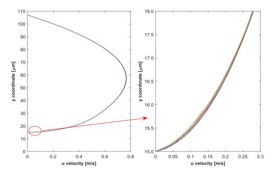
Figure A.3: Velocity distributions over the tip point of middle roughness element (along the R2-L3 line) and close-up view near the tip point.
