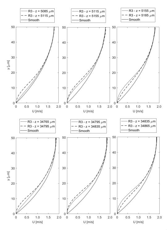
Figure 6.81: Velocity magnitude profiles along the *y*-direction at  $x = 50 \mu m$  and various *z* locations for the first and last roughness element set of RDC configuration.
