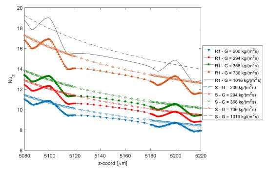
Figure 6.38: Local Nusselt distribution over the first two roughness elements of R1LC configuration.
