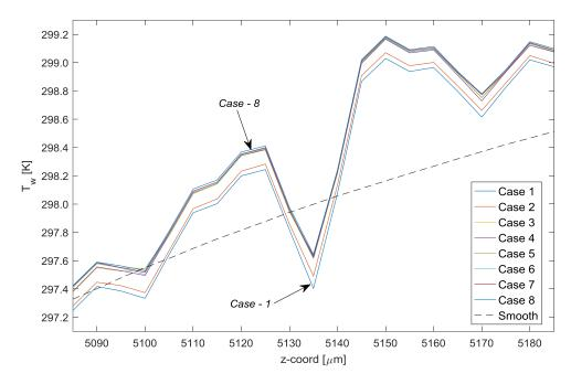
Figure 6.75: Wall mean temperature distribution for mesh independence test cases of RDC configuration around the first roughness element set.
