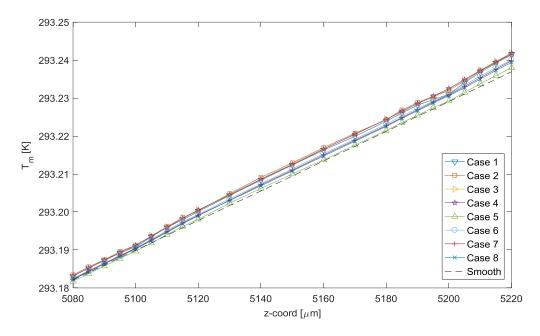
Figure 6.12: Fluid bulk mean temperature distribution for mesh independence test cases of R1LC configuration around the first two roughness elements.
