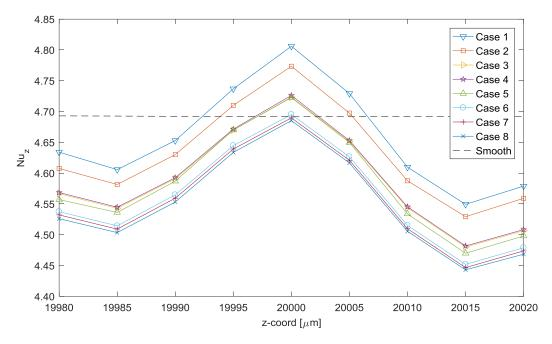
Figure 6.18: Local Nusselt distribution for mesh independence test cases of R1LC configuration around the middle roughness elements.
