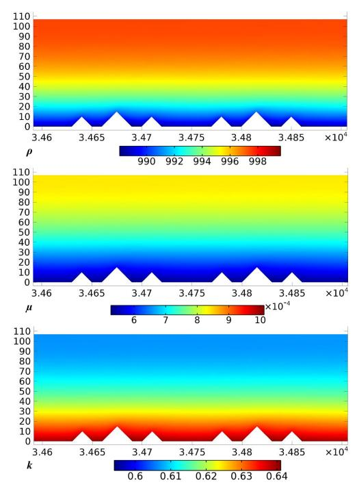
Figure 6.94: Variation of  $\rho$ ,  $\mu$ , and k over the last two roughness element set of RDC configuration at  $x = 50 \ \mu\text{m}$  plane for  $G = 1016 \ \text{kg/(m^2s)}$ .
