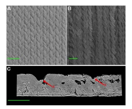
Figure 2.14: Images of Speedo shark skin-like swimsuit fabric (Fastskin FS II) (Scale bars =  $500 \ \mu m$ ). (A) Underside surface image (non-biomimetic), (B) Outside surface image (biomimetic), (C) Cross-section image showing the dents on the biomimetic side (red arrows) [81].
