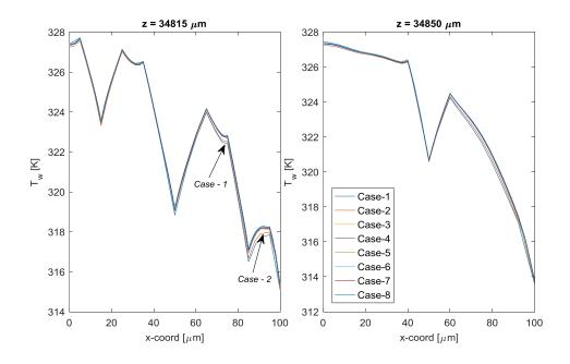
Figure 6.74: Wall temperature distributions for mesh independence test cases of RDC configuration along the *x*-direction at  $z = 34815 \ \mu m$  and  $z = 34850 \ \mu m$  locations.
