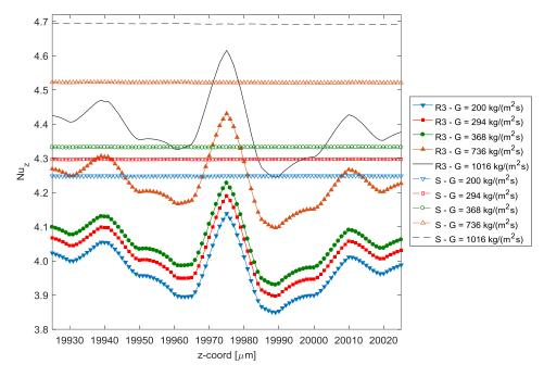
Figure 6.96: Local Nusselt distribution over the middle roughness element set of RDC configuration
