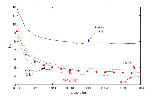
Figure B.2: Local Nu values for test cases of stabilization methods.
