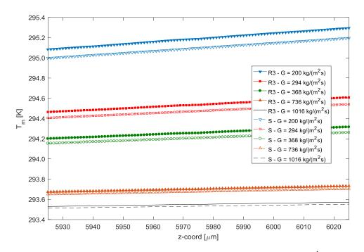
Figure 6.88: Fluid bulk mean temperature distribution over the 7<sup>th</sup> roughness element set of RDC configuration.
