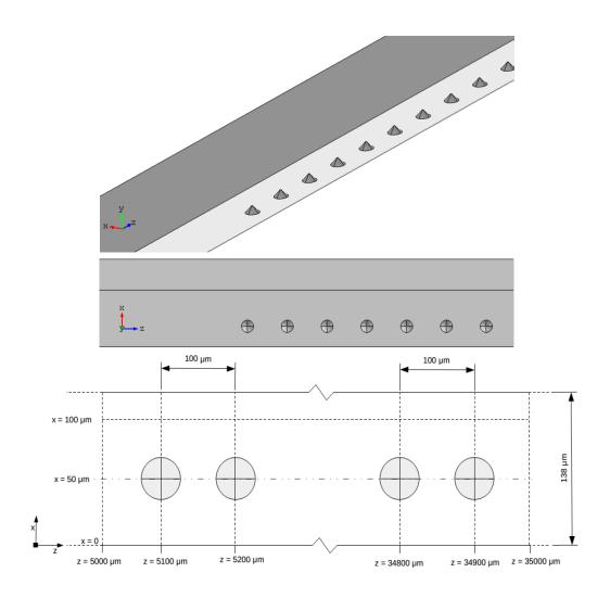
Figure 5.5: Model of *Micro\_G06 (1LineCone)* case and geometrical properties of its roughness elements.
