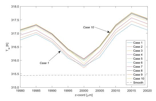
Figure 6.46: Wall mean temperature distribution for mesh independence test cases of R2LC configuration around the middle roughness element.
