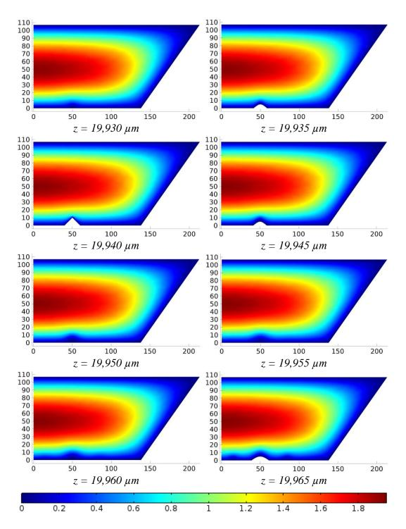
Figure 6.83: Velocity distribution at various cross-sections through the middle roughness element set of RDC configuration in the flow direction (G = 1016 [kg/(m<sup>2</sup>s)]).
