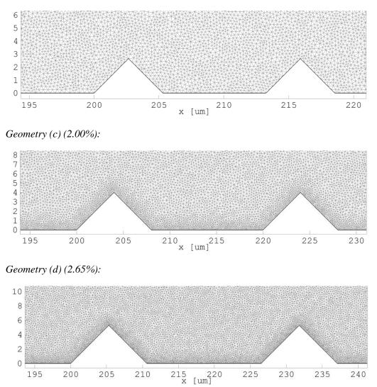
Figure 4.5: Distribution of chosen meshes around the first two roughness elements of 2D parallel plate channels.
