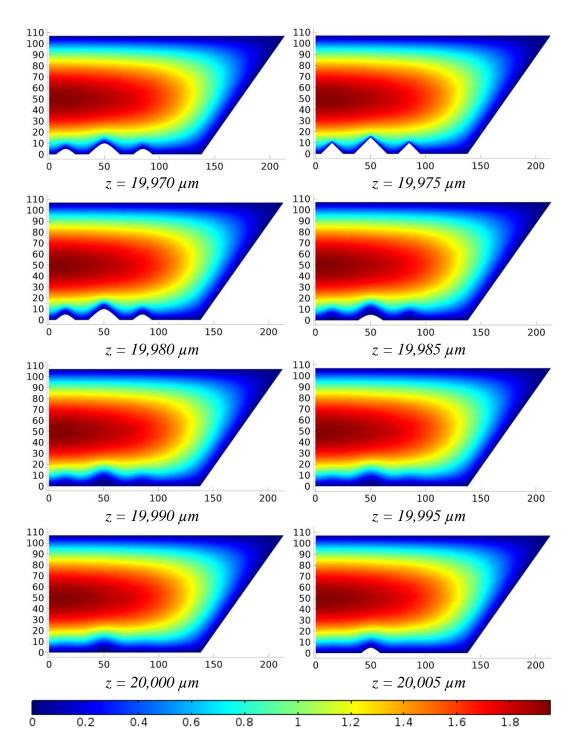
Figure 6.83: Velocity distribution at various cross-sections through the middle roughness element set of RDC configuration in the flow direction (G = 1016 [kg/(m<sup>2</sup>s)]) (*Continued*).
