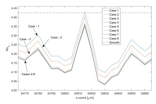
Figure 6.79: Local Nusselt distribution for mesh independence test cases of RDC configuration around the last roughness element set.
