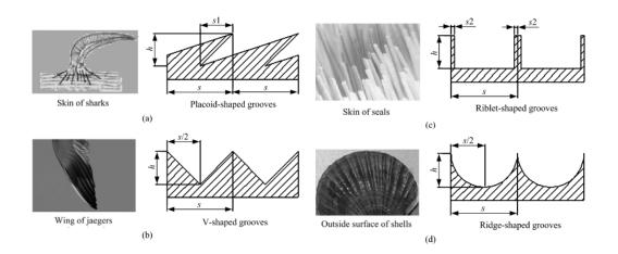
Figure 2.4: Bionic surface geometries considered in [70] (a) placoid-shaped grooves,(b) V-shaped grooves, (c) riblet-shaped grooves, and (d) ridge-shaped grooves.
