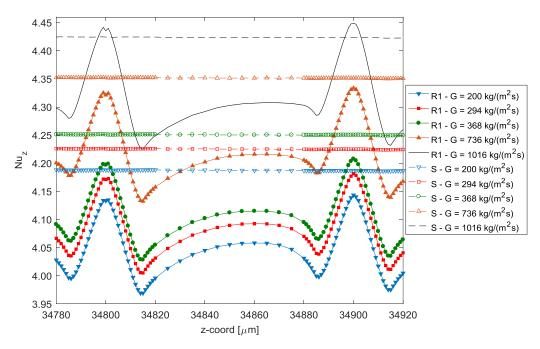
Figure 6.40: Local Nusselt distribution over the last two roughness elements of R1LC configuration.
