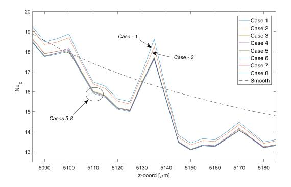
Figure 6.77: Local Nusselt distribution for mesh independence test cases of RDC configuration around the first roughness element set.
