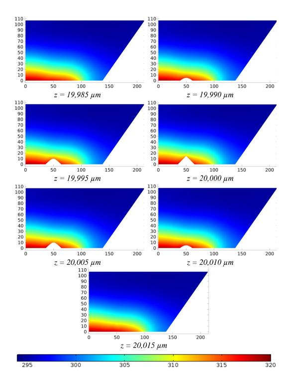
Figure 6.28: Temperature distribution at various cross-sections around the middle cone of R1LC configuration in the flow direction ( $G = 1016 [kg/(m^2s)]$ ).
