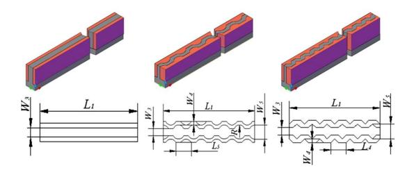
Figure 2.9: Schematics of simulated channels in [77], regular rectangular (left), with offset fan-shaped reentrant cavities (middle), and with triangular reentrant cavities (right).
