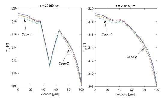
Figure 6.14: Wall temperature distributions for mesh independence test cases of R1LC configuration along the *x*-direction at  $z = 20000 \ \mu m$  and  $z = 20015 \ \mu m$  locations.
