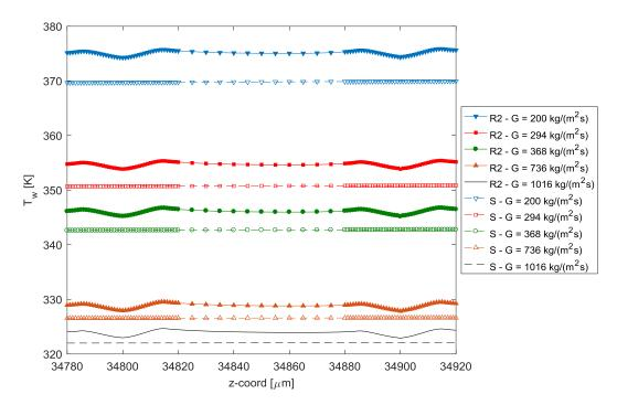
Figure 6.63: Wall mean temperature distribution over the last two roughness elements of R2LC configuration.
