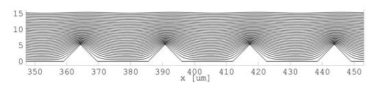
Figure 4.6: Streamlines around the middle roughness elements for *Case-03* of 2D rough channel geometries for Re = 100.
