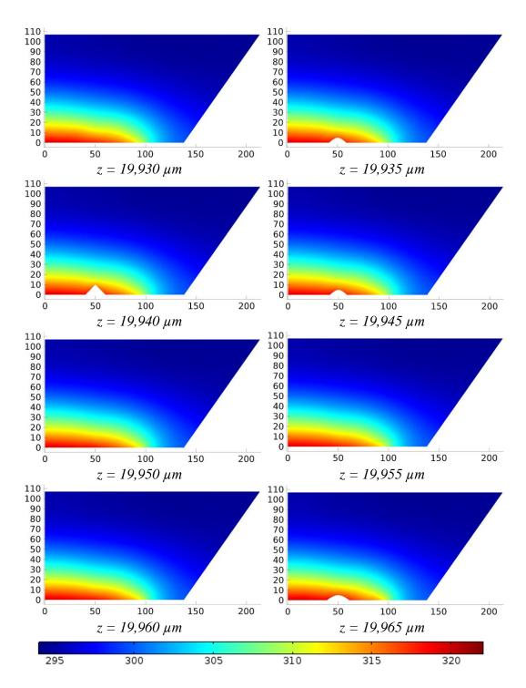
Figure 6.87: Temperature distribution at various cross-sections through the middle roughness element set of RDC configuration in the flow direction (G = 1016 [kg/(m<sup>2</sup>s)]).
