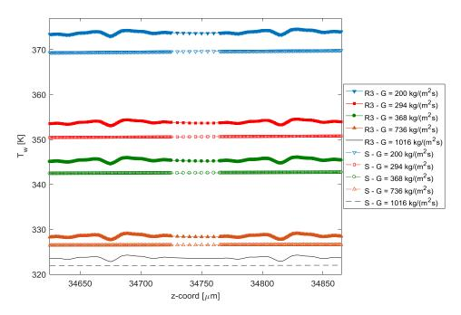
Figure 6.92: Wall mean temperature distribution over the last two roughness element sets of RDC configuration.
