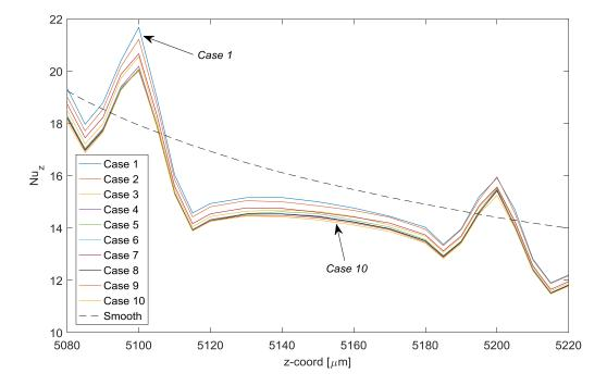
Figure 6.47: Local Nusselt distribution for mesh independence test cases of R2LC configuration around the first two roughness elements.
