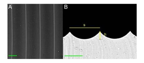
Figure 2.13: Images of the biomimetic riblet silicone material (Scale bars =  $200 \ \mu m$ ). (A) Front side. (B) Cross-section view, h =  $87 \ \mu m$ , s =  $340 \ \mu m$  [81].
