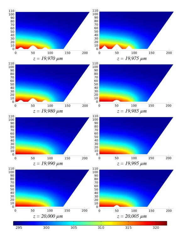
Figure 6.87: Temperature distribution at various cross-sections through the middle roughness element set of RDC configuration in the flow direction (G = 1016 [kg/(m<sup>2</sup>s)]) (*Continued*).
