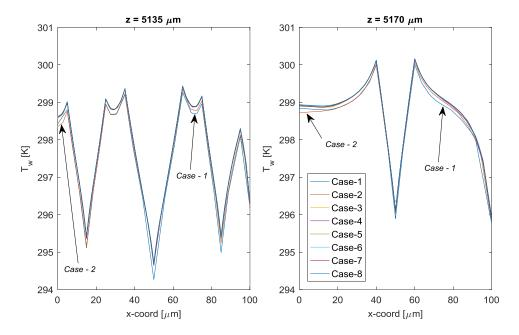
Figure 6.72: Wall temperature distributions for mesh independence test cases of RDC configuration along the *x*-direction at  $z = 5135 \mu m$  and  $z = 5170 \mu m$  locations.
