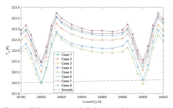
Figure 6.16: Wall mean temperature distribution for mesh independence test cases of R1LC configuration around the last two roughness elements.
