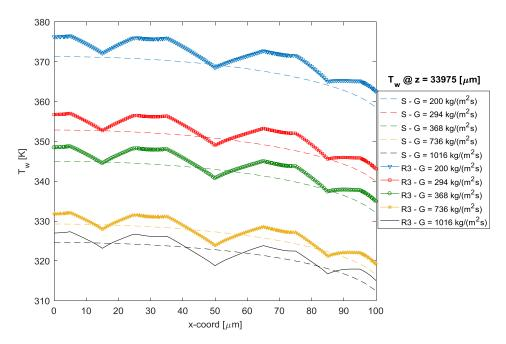
Figure 6.85: Wall temperature distribution at  $z = 33975 \ \mu m$  location for various inlet mass fluxes for RDC configuration with corresponding smooth values.
