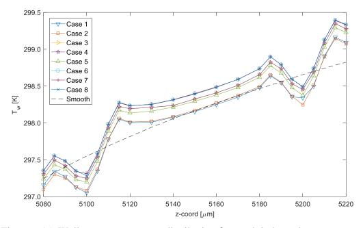
Figure 6.15: Wall mean temperature distribution for mesh independence test cases of R1LC configuration around the first two roughness elements.
