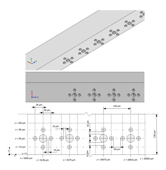
Figure 5.7: Model of *Micro\_G08 (DaisyCone)* case and geometrical properties of its roughness elements.
