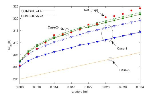
Figure B.1: Wall mean temperatures calculated with COMSOL v4.4 and v5.2a for test cases of stabilization methods.
