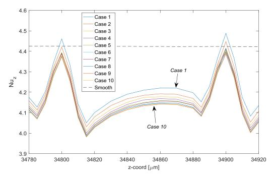
Figure 6.49: Local Nusselt distribution for mesh independence test cases of R2LC configuration around the last two roughness elements.
