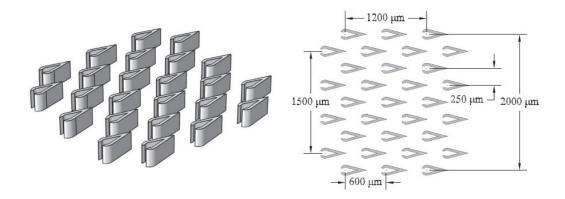
Figure 2.16: Piranha Pin Fin (PPF) array used in [91].
