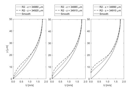
Figure 6.51: Velocity magnitude profiles along *y*-direction at  $x = 69 \mu m$  and various *z* locations for the last conical element of R2LC configuration.
