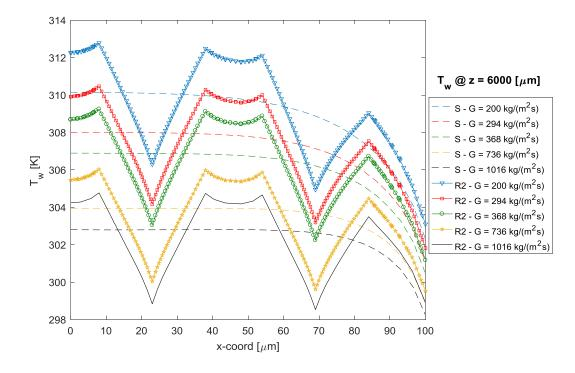
Figure 6.55: Wall temperature distribution at  $z = 6000 \mu m$  location for various inlet mass fluxes for R2LC configuration with corresponding smooth values.
