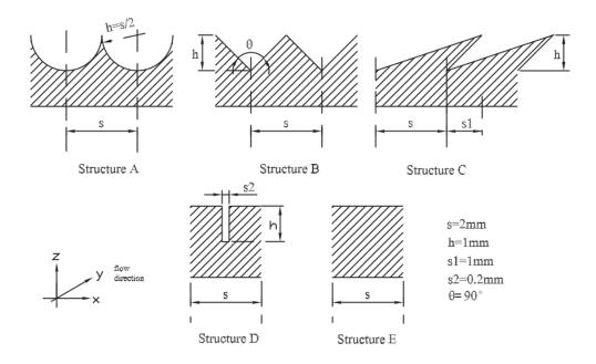
Figure 2.3: Representative channel geometries used in [69] (A) ridge-shaped grooves, (B) V-shaped grooves, (C) shield-shaped grooves, (D) straight slot grooves, and (E) smooth surface.
