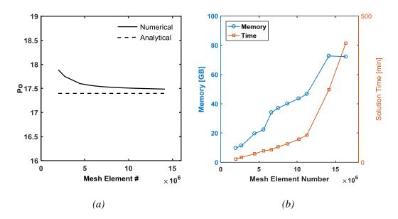
Figure 5.2: (a) Change of *Po* values with respect to element number for mesh independence runs of *Macro\_G01* case, (b) Solution time and memory use with respect to element numbers.
