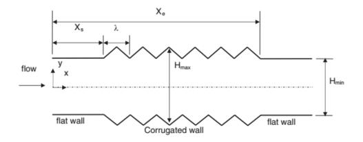
Figure 2.5: Schematics of the corrugated channel used in [72].
