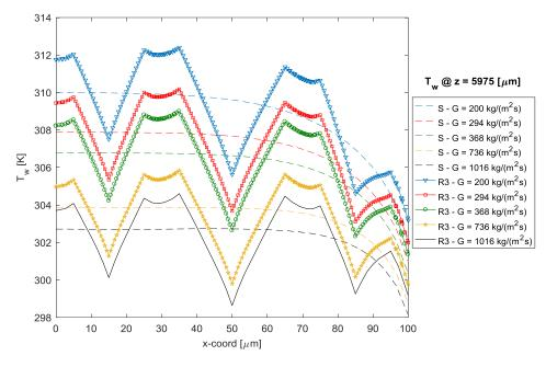
Figure 6.84: Wall temperature distribution at  $z = 5975 \mu m$  location for various inlet mass fluxes for RDC configuration with corresponding smooth values.
