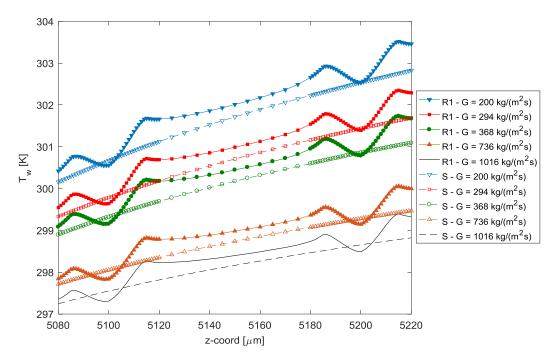
Figure 6.31: Wall mean temperature distribution over the first two roughness elements of R1LC configuration.
