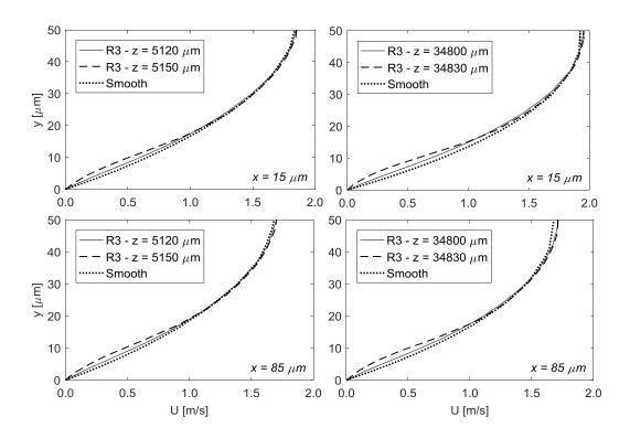
Figure 6.80: Velocity magnitude profiles around the small side cones of first and last roughness element set of RDC configuration along the *y*-direction at  $x = 15 \mu m$  and  $x = 85 \mu m$  for various *z* locations.
