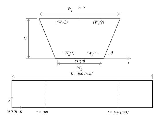
Figure 5.1: Schematics of the cross-sections of trapezoidal channel used in macroscale flow simulations.
