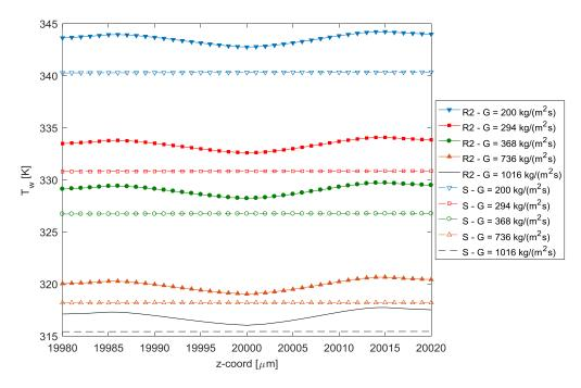
Figure 6.62: Wall mean temperature distribution near the middle roughness elements of R2LC configuration.
