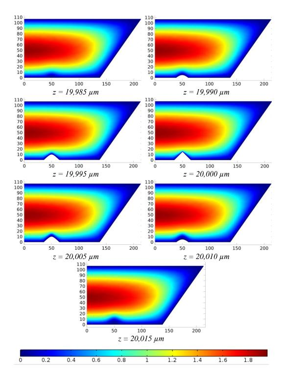
Figure 6.24: Velocity distribution at various cross-sections around the middle cone of R1LC configuration in the flow direction ( $G = 1016 [kg/(m^2s)]$ ).
