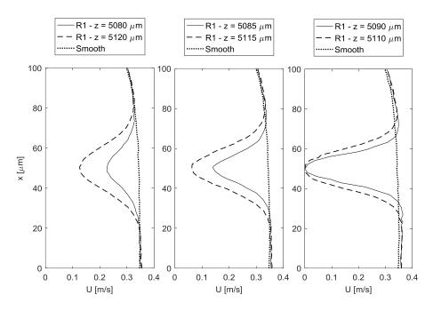
Figure 6.22: Velocity magnitude profiles along *x*-direction at  $y = 5 \mu m$  and various *z* locations for the first conical element of R1LC configuration.
