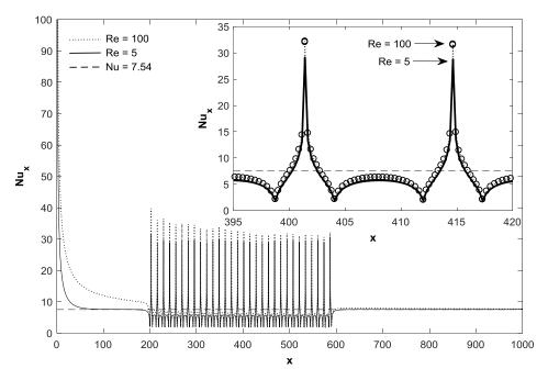
Figure 4.9: Local *Nu* distribution along the 2D *Geometry* (*b*) ( $\varepsilon = 1.325\%$ ) and closeup view between the two consecutive roughness elements.
