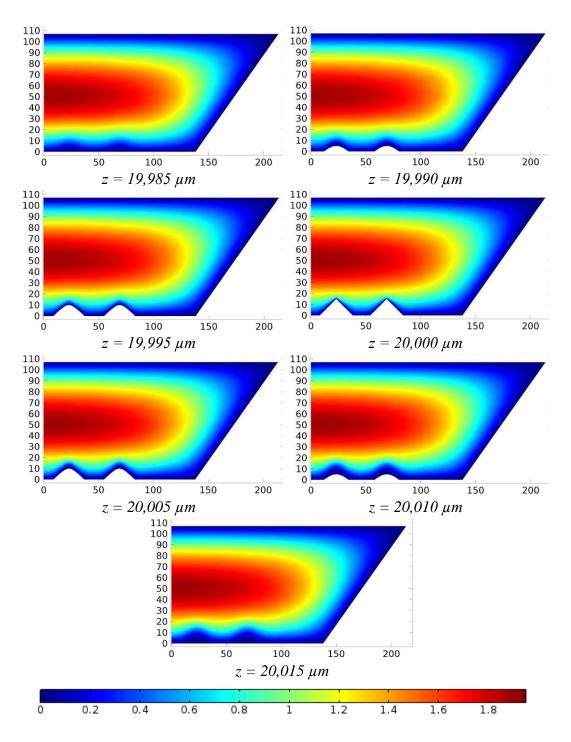
Figure 6.54: Velocity distribution at various cross-sections around the middle cone of R2LC configuration in the flow direction ( $G = 1016 [kg/(m^2s)]$ ).
