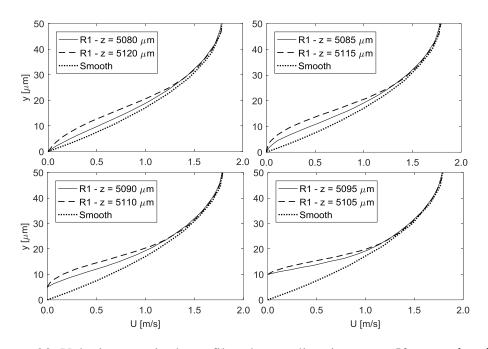
Figure 6.20: Velocity magnitude profiles along *y*-direction at  $x = 50 \mu m$  and various *z* locations for the first conical element of R1LC configuration.
