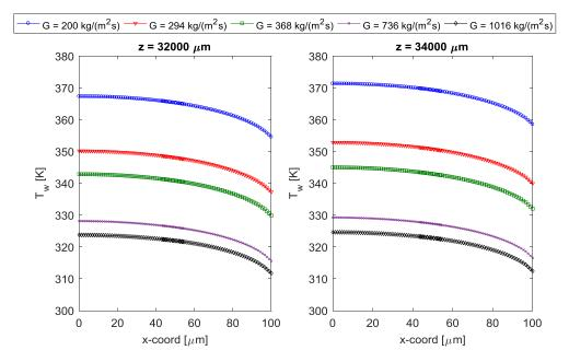
Figure 6.5: Wall temperatures over the last two microheaters (at  $z = 32000 \ \mu\text{m}$  and  $z = 34000 \ \mu\text{m}$ ) along x-direction for various inlet mass fluxes.
