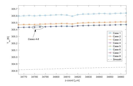
Figure 6.71: Fluid bulk mean temperature distribution for mesh independence test cases of RDC configuration over the last roughness element set.
