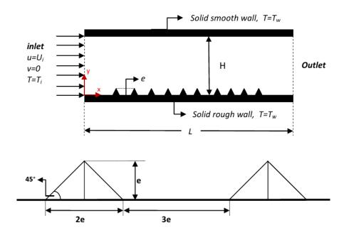
Figure 4.1: Schematics of the rough parallel-plate channels and geometrical properties of roughness elements [106].
