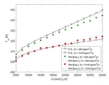
Figure 6.7: Wall mean temperatures for inlet mass fluxes of 294 kg/(m<sup>2</sup>s) and 1016 kg/(m<sup>2</sup>s) with reference results (*P.S.*: Present Study, *Ref.*: Reference Work, *Exp.*: Experimental, *Num.*: Numerical).
