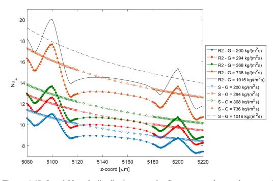
Figure 6.65: Local Nusselt distribution over the first two roughness elements of R2LC configuration.
