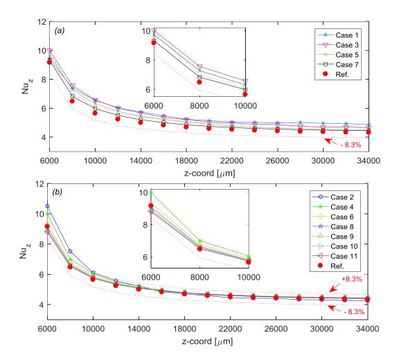
Figure 6.3: Local Nusselt numbers over the microheaters for the mesh independence test cases (a) Cases with predefined meshes, (b) Cases with manually adjusted meshes ( $q_{eff} = 300 \text{ kW/m}^2$ ,  $G = 1016 \text{ kg/(m}^2\text{s})$ ).
