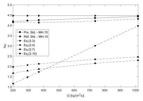
Figure 6.10: Comparison of *Nu* values obtained from the equations proposed in literature (*Prs. Std.*: Present Study, *Ref. Std.*: Reference Study [26], *MH.15*: 15<sup>th</sup> microheater).
