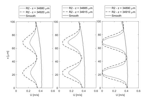
Figure 6.53: Velocity magnitude profiles along *x*-direction at  $y = 5 \mu m$  and various *z* locations for the last conical element of R2LC configuration.
