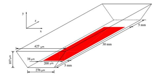
Figure 6.1: Schematic of trapezoidal microchannel and placement of heated section in the reference work [26].
