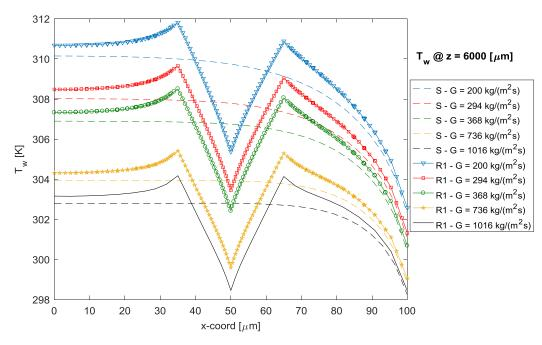
Figure 6.25: Wall temperature distribution at  $z = 6000 \mu m$  location for various inlet mass fluxes for R1LC configuration with corresponding smooth values.
