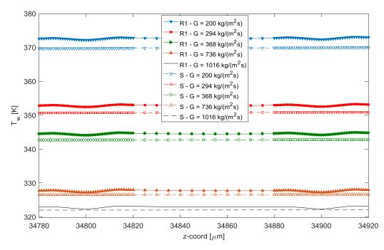
Figure 6.33: Wall mean temperature distribution over the last two roughness elements of R1LC configuration.
