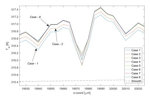
Figure 6.76: Wall mean temperature distribution for mesh independence test cases of RDC configuration around the middle roughness element set.
