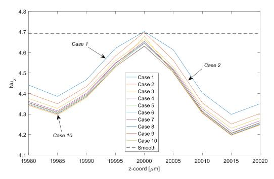
Figure 6.48: Local Nusselt distribution for mesh independence test cases of R2LC configuration around the middle roughness elements.
