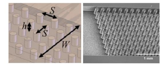
Figure 2.7: Schematic view of the channel with micro cylinders (left), and SEM image of a silicon micro cylinder array [74].
