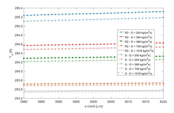
Figure 6.59: Fluid bulk mean temperature distribution over the 10<sup>th</sup> roughness elements of R2LC configuration.
