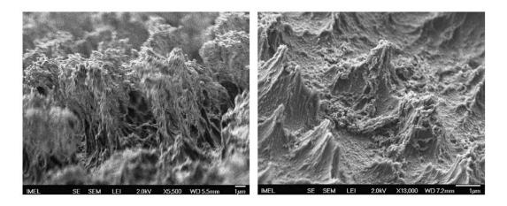
Figure 2.11: SEM images of PMMA surfaces at the bottom of microchannels formed by means of etching in O<sub>2</sub> plasma prior to (left) and after (right) immersion in water and drying [80].
