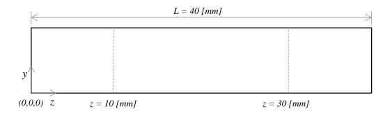
Figure 5.3: Schematics of the side view of microchannel geometry along the flow direction used in smooth microscale flow simulations.
