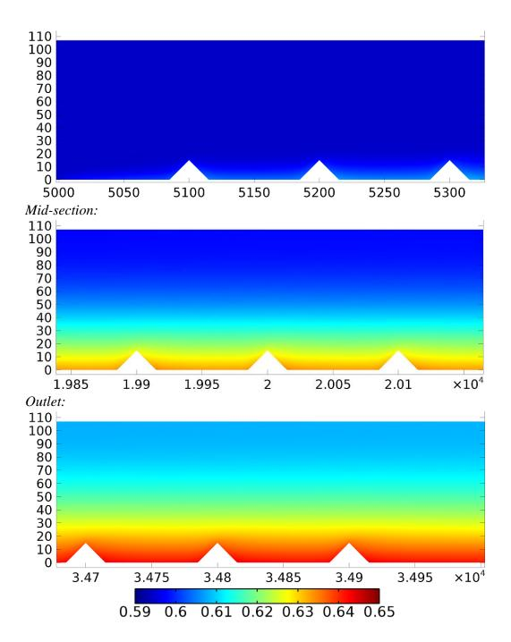
Figure 6.68: Change of thermal conductivity at  $x = 23 \mu m$  plane through the inlet to the outlet of the rough section of R2LC configuration ( $G = 1016 [kg/(m^2s)]$ ).
