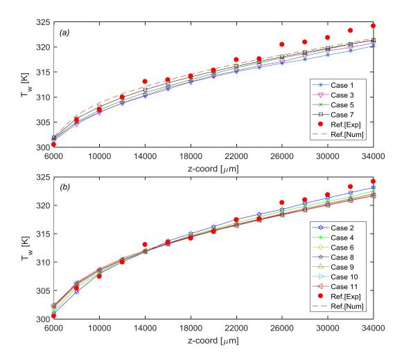
Figure 6.2: Wall mean temperatures over the microheaters for the mesh independence tests cases (a) Cases with predefined meshes, (b) Cases with manually adjusted meshes ( $q_{eff} = 300 \text{ kW/m}^2$ ,  $G = 1016 \text{ kg/(m}^2\text{s})$ ).
