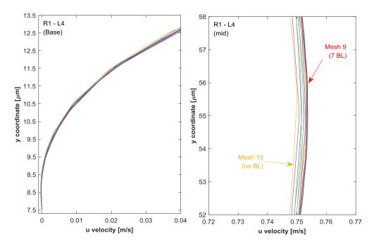
Figure A.2: Close-up views of velocity distributions near the base and around the middle of the *R1-L4* line.
