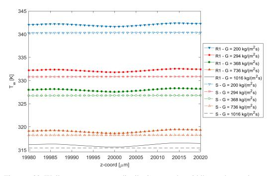
Figure 6.32: Wall mean temperature distribution near the middle roughness element of R1LC configuration.
