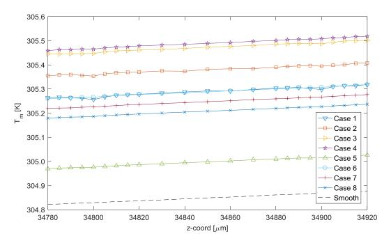
Figure 6.13: Fluid bulk mean temperature distribution for mesh independence test cases of R1LC configuration around the last two roughness elements.
