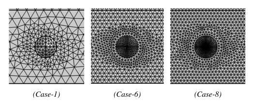
Figure 6.11: Surface meshes around the conical elements of R1LC configuration for *Case-1* (coarsest), *Case-6*, and *Case-8* (densest).
