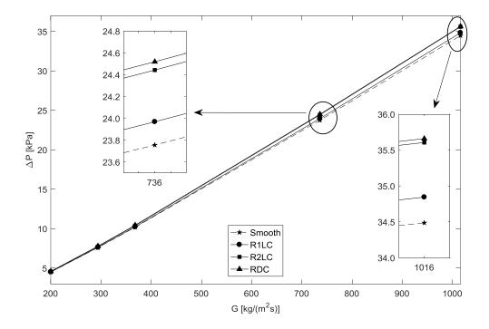
Figure 6.98: Pressure drop between the inlet and exit of heated section of smooth and rough channels for various inlet mass fluxes.
