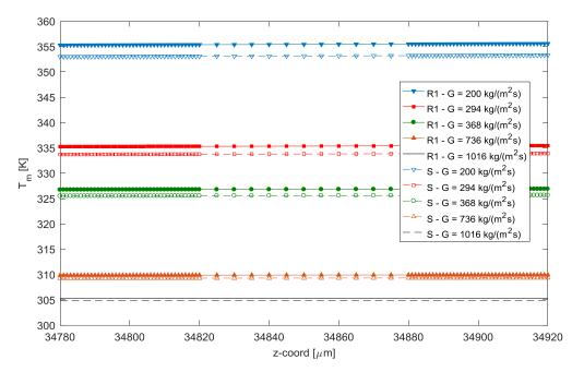
Figure 6.30: Fluid bulk mean temperature distribution over the last two roughness elements of R1LC configuration.
