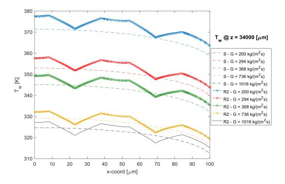
Figure 6.56: Wall temperature distribution at  $z = 34000 \ \mu m$  location for various inlet mass fluxes for R2LC configuration with corresponding smooth values.
