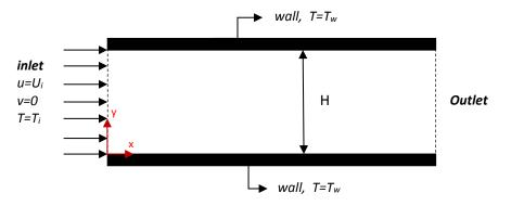
Figure 3.1: Schematics of 2D parallel plate microchannel and boundary conditions.
