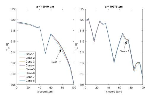
Figure 6.73: Wall temperature distributions for mesh independence test cases of RDC configuration along the *x*-direction at  $z = 19940 \ \mu m$  and  $z = 19975 \ \mu m$  locations.
