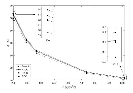
Figure 6.99: Temperature difference between the inlet and outlet of heated section of smooth and rough channels for various inlet mass fluxes.
