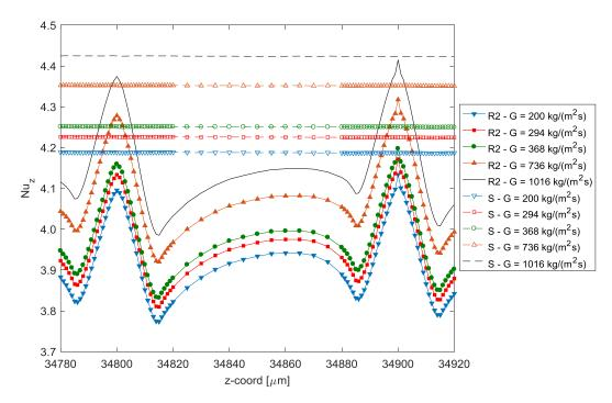
Figure 6.67: Local Nusselt distribution over the last two roughness elements of R2LC configuration.
