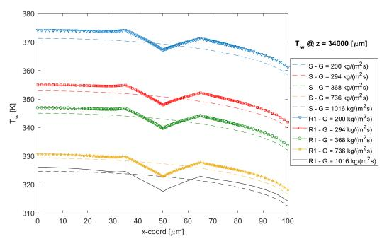
Figure 6.26: Wall temperature distribution at  $z = 34000 \ \mu m$  location for various inlet mass fluxes for R1LC configuration with corresponding smooth values.
