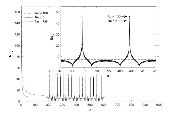
Figure 4.10: Local *Nu* distribution along the 2D *Geometry* (*c*) ( $\varepsilon = 2.00\%$ ) and closeup view between the two consecutive roughness elements.
