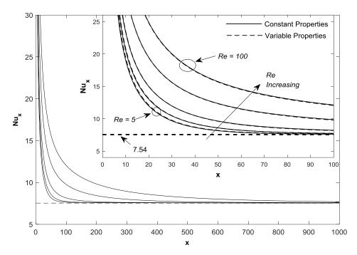
Figure 4.8: Local *Nu* distribution along the 2D *Geometry* (*a*) (*smooth*) and close-up view of entrance section.
