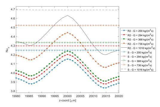
Figure 6.66: Local Nusselt distribution near the middle roughness element of R2LC configuration.
