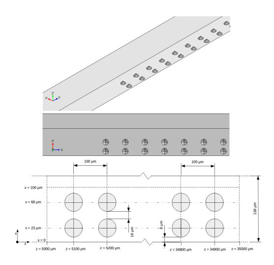
Figure 5.6: Model of *Micro\_G07 (2LineCone)* case and geometrical properties of its roughness elements.
