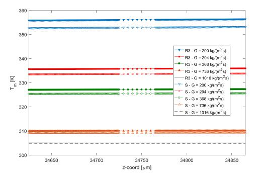
Figure 6.89: Fluid bulk mean temperature distribution over the last two roughness element sets of RDC configuration.
