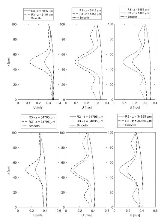
Figure 6.82: Velocity magnitude profiles along the *x*-direction at  $y = 5 \mu m$  and various *z* locations for the first and last roughness element set of RDC configuration.
