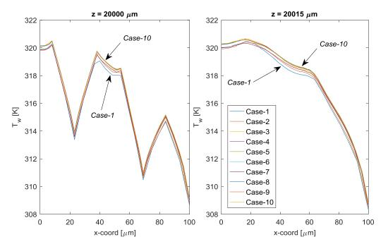
Figure 6.43: Wall temperature distributions for mesh independence test cases of R2LC configuration along the *x*-direction at  $z = 20000 \ \mu m$  and  $z = 20015 \ \mu m$  locations.
