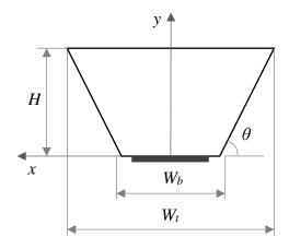
Figure 3.2: Representative schematic for channels having trapezoidal cross-section.
