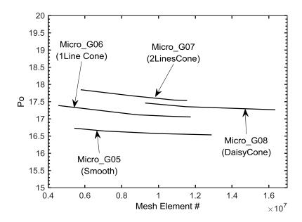
Figure 5.8: Calculated *Po* values with respect to mesh element numbers for mesh independence studies of micro smooth and rough geometries.
