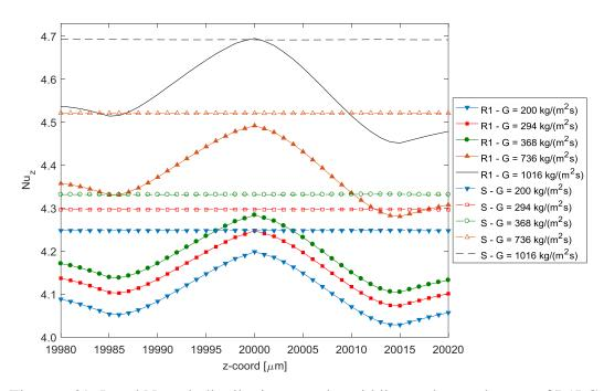
Figure 6.39: Local Nusselt distribution near the middle roughness element of R1LC configuration.
