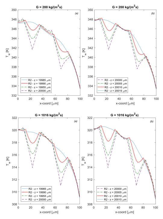
Figure 6.57: Wall temperature distribution around the middle cone of R2LC configuration for inlet mass fluxes of 200 kg/( $m^2s$ ) and 1016 kg/( $m^2s$ ) for (a) flow facing side of the cone, (b) back side of the cone.
