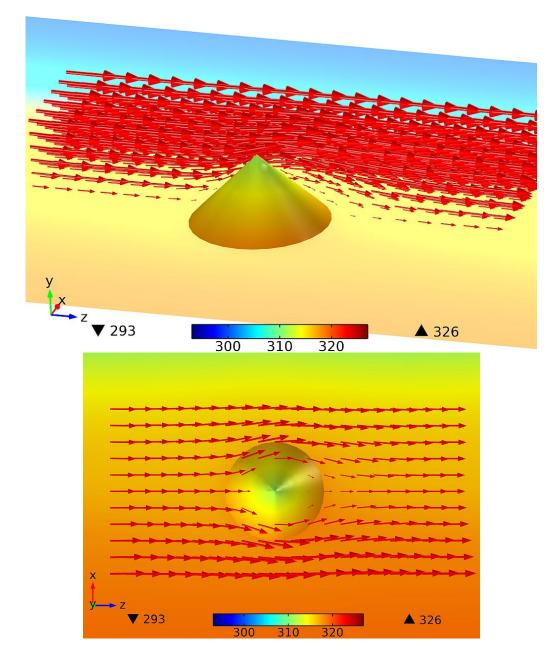
Figure 6.34: Surface temperature and convective heat flux around the middle cone of R1LC configuration for  $G = 1016 \text{ [kg/(m^2s)]}$  (*Top:* heat flux around the half of the cone, *Bottom:* heat flux at  $y = 7.5 \mu \text{m}$  plane).
