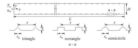
Figure 2.1: Schematic of the rough microchannel and roughness elements used in [62].
