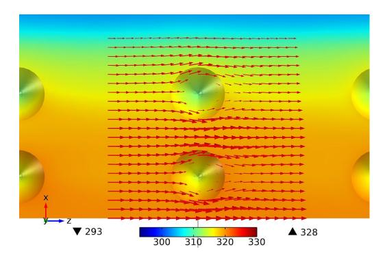
Figure 6.64: Surface temperature around the middle conical elements of R2LC configuration and convective het flux in the fluid at  $y = 7.5 \ \mu m$  plane ( $G = 1016 \ [kg/(m^2s)]$ ).
