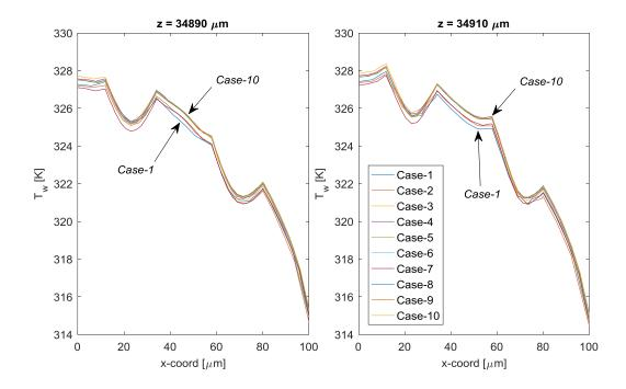
Figure 6.44: Wall temperature distributions for mesh independence test cases of R2LC configuration along the *x*-direction at  $z = 34890 \ \mu m$  and  $z = 34910 \ \mu m$  locations.
