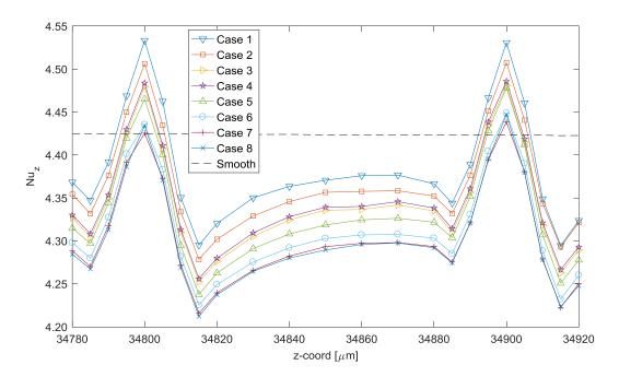
Figure 6.19: Local Nusselt distribution for mesh independence test cases of R1LC configuration around the last two roughness elements.
