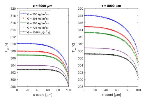
Figure 6.4: Wall temperatures over the first two microheaters (at  $z = 6000 \ \mu\text{m}$  and  $z = 8000 \ \mu\text{m}$ ) along x-direction for various inlet mass fluxes.
