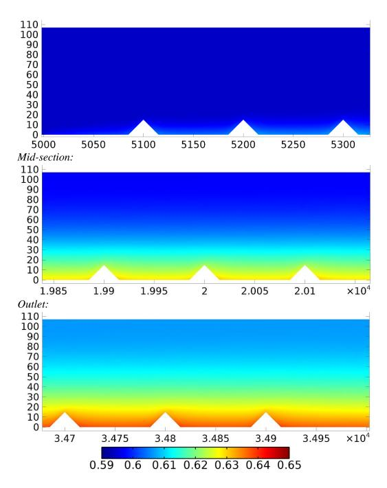
Figure 6.69: Change of thermal conductivity at  $x = 69 \mu m$  plane through the inlet to the outlet of the rough section of R2LC configuration ( $G = 1016 [kg/(m^2s)]$ ).
