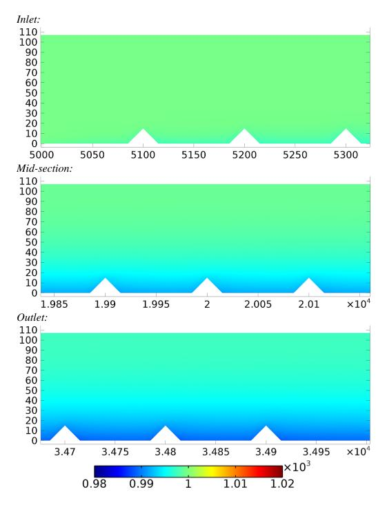
Figure 6.35: Change of density at  $x = 50 \mu m$  plane through the inlet to outlet of the rough section of R1LC configuration ( $G = 1016 [kg/(m^2s)]$ ).
