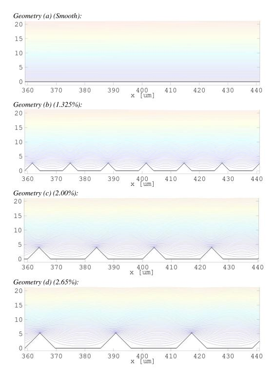
Figure 4.7: Velocity contour plots around the middle roughness elements for *Case-*03 of 2D smooth and rough channel geometries for Re = 100.
