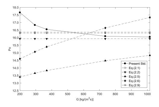
Figure 6.9: Comparison of *Po* values obtained from the equations proposed in literature.
