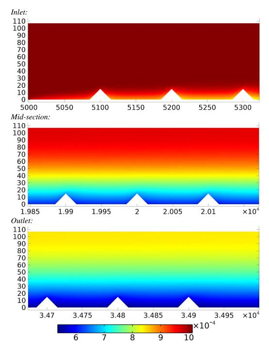
Figure 6.36: Change of viscosity at  $x = 50 \mu m$  plane through the inlet to outlet of the rough section of R1LC configuration ( $G = 1016 [kg/(m^2s)]$ ).
