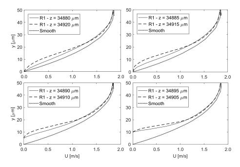
Figure 6.21: Velocity magnitude profiles along *y*-direction at  $x = 50 \mu m$  and various *z* locations for the last conical element of R1LC configuration.
