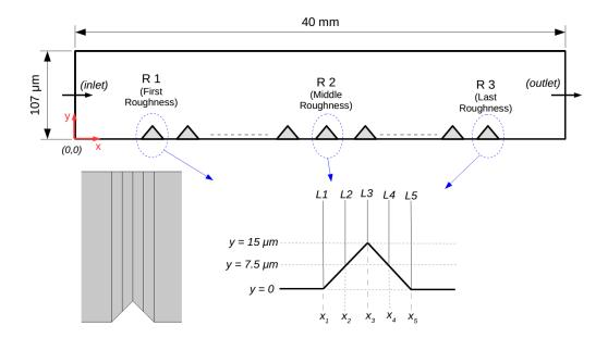
Figure A.1: Schematics of 2D test channel and the locations of data extraction lines.
