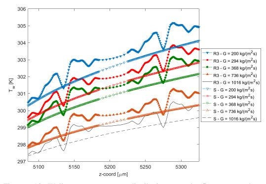
Figure 6.90: Wall mean temperature distribution over the first two roughness element sets of RDC configuration.
