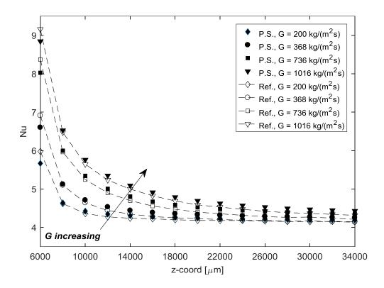
Figure 6.8: Calculated *Nu* values for various inlet mass fluxes along with the reference results (*P.S.*: Present Study, *Ref.*: Reference Work).
