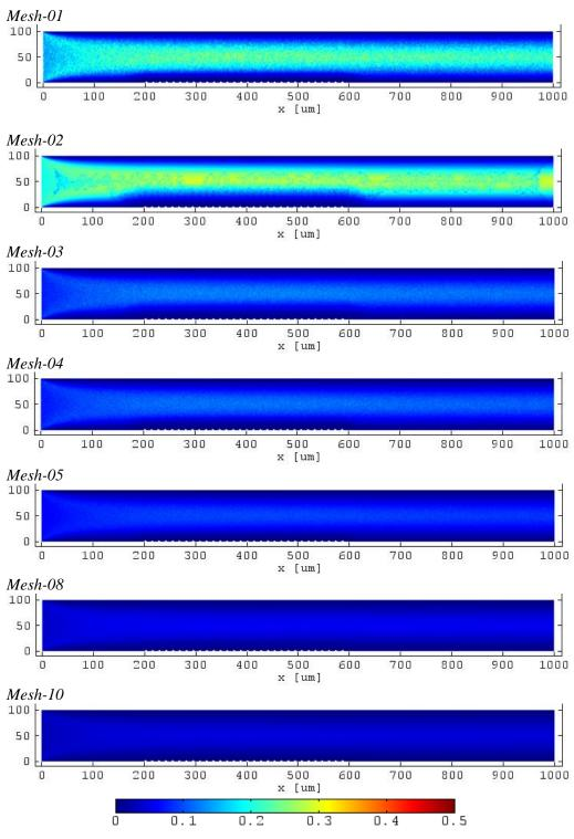
Figure 4.2: Selected cell *Re* plots for mesh independence studies of *Geometry* (*b*) *Case-04* (with 1.325% relative roughness).
