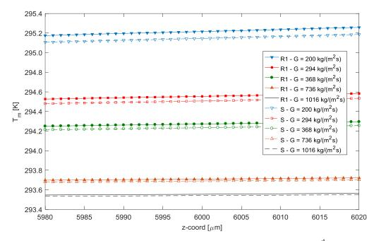
Figure 6.29: Fluid bulk mean temperature distribution over the 10<sup>th</sup> roughness element of R1LC configuration.
