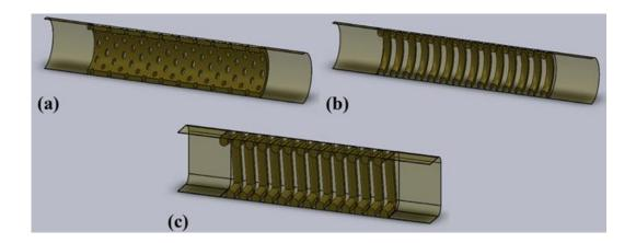
Fig. 2.17: Wall thickening patterns used in the simulations of [96].
