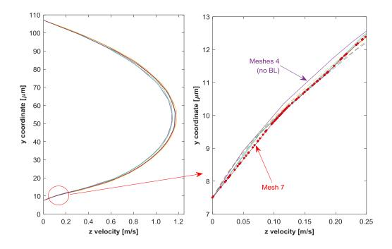
Figure A.5: *w*-velocity distributions along the second line of first roughness element and close-up view of the base section.
