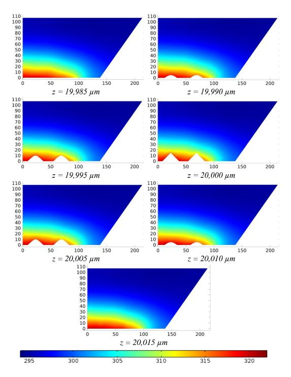
Figure 6.58: Temperature distribution at various cross-sections around the middle cone of R2LC configuration in the flow direction ( $G = 1016 [kg/(m^2s)]$ ).
