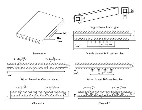
Figure 2.8: Schematic views of the channels considered in [76].
