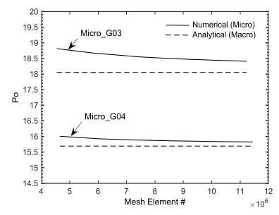
Figure 5.4: Change in *Po* with respect to mesh element number for *Micro\_G03* and *Micro\_G04* cases.
