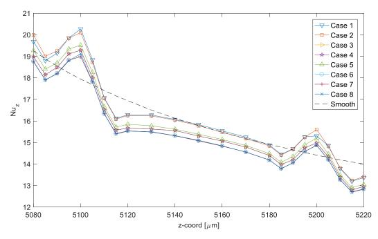
Figure 6.17: Local Nusselt distribution for mesh independence test cases of R1LC configuration around the first two roughness elements.
