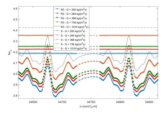
Figure 6.97: Local Nusselt distribution over the last two roughness element sets of RDC configuration.
