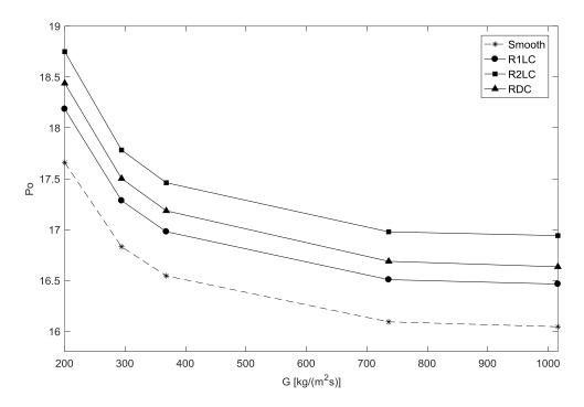
Figure 6.100: Change in *Po* value with inlet mass flux in smooth and rough channels.
