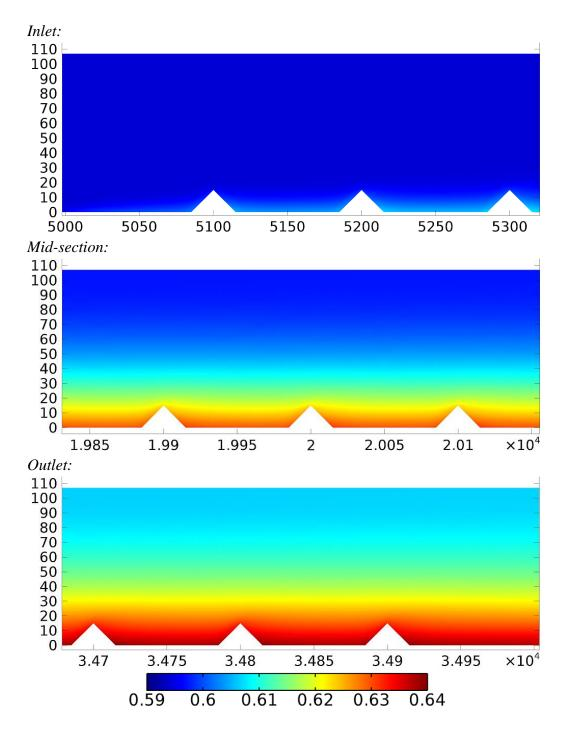
Figure 6.37: Change of thermal conductivity at  $x = 50 \mu m$  plane through the inlet to outlet of the rough section of R1LC configuration ( $G = 1016 [kg/(m^2s)]$ ).
