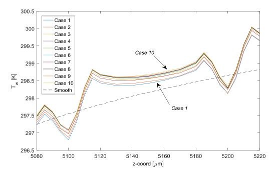
Figure 6.45: Wall mean temperature distribution for mesh independence test cases of R2LC configuration around the first two roughness elements.
