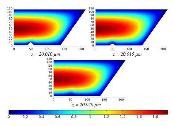
Figure 6.83: Velocity distribution at various cross-sections through the middle roughness element set of RDC configuration in the flow direction (G = 1016 [kg/(m<sup>2</sup>s)]) (*Continued*).
