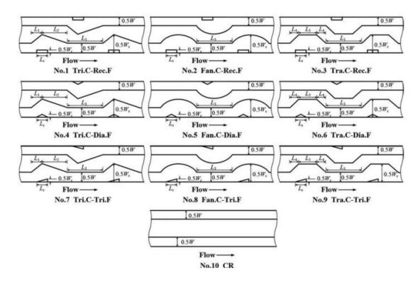
Figure 2.10: Schematics of channels used in [78] (*Rec*: Rectangular, *Tri*: Triangular, *Fan*: Fan shaped, *Tra*: Trapezoidal, *Dia*: Diamond, *C*: Cavity, *F*: Fin, *CR*: Conventional Rectangular).
