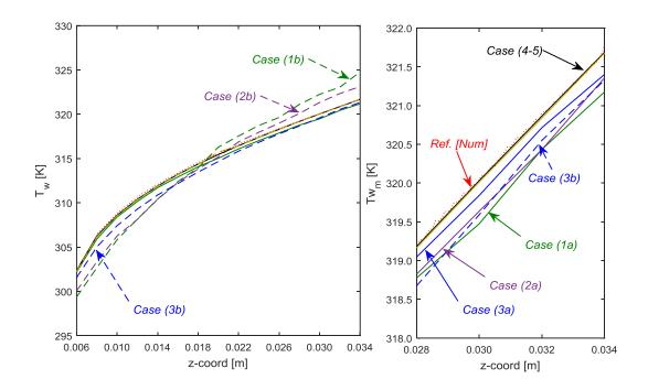
Figure B.3: Wall mean temperature distribution over the heated section for first and second order mesh elements.
