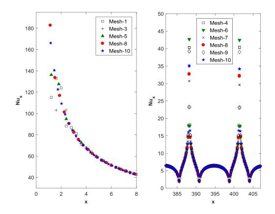
Figure 4.4: Local *Nu* distribution at the inlet of the channel and at the middle of the rough section for *Case-04* of *Geometry* (*b*) and Re = 100.
