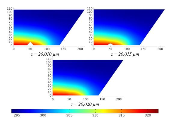
Figure 6.87: Temperature distribution at various cross-sections through the middle roughness element set of RDC configuration in the flow direction (G = 1016 [kg/(m<sup>2</sup>s)]) (*Continued*).
