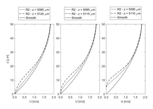
Figure 6.50: Velocity magnitude profiles along *y*-direction at  $x = 23 \mu m$  and various *z* locations for the first conical element of R2LC configuration.
