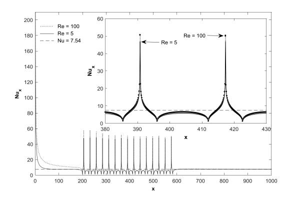
Figure 4.11: Local *Nu* distribution along the 2D *Geometry* (*d*) ( $\varepsilon = 2.65\%$ ) and closeup view between the two consecutive roughness elements.
