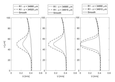
Figure 6.23: Velocity magnitude profiles along *x*-direction at  $y = 5 \mu m$  and various *z* locations for the last conical element of R1LC configuration.
