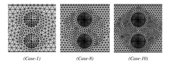
Figure 6.41: Surface meshes around the conical elements of R2LC configuration for *Case-1* (coarsest), *Case-8*, and *Case-10* (densest).
