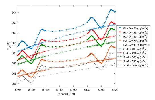
Figure 6.61: Wall mean temperature distribution over the first two roughness elements of R2LC configuration.
