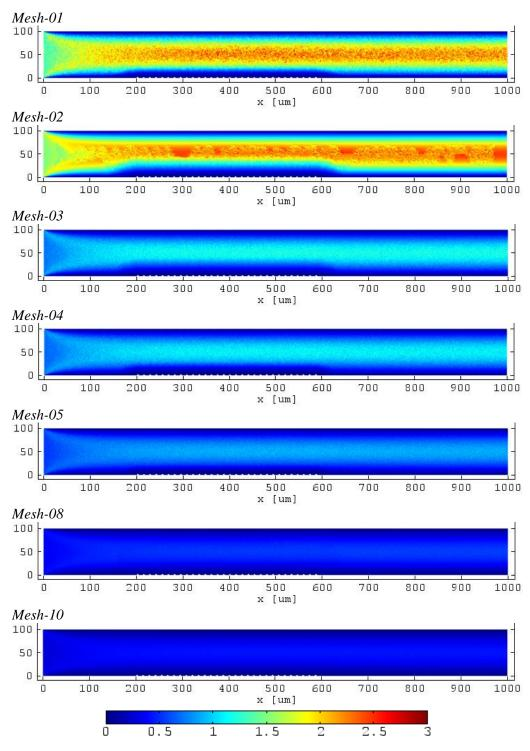
Figure 4.3: Selected cell *Pe* plots for mesh independence studies of *Geometry* (*b*) *Case-04* (with 1.325% relative roughness).
