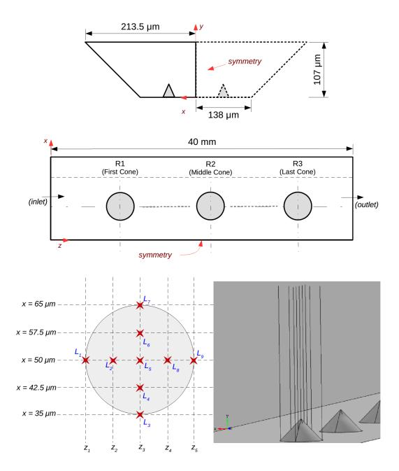
Figure A.4: Schematics of 3D test channel and the locations of data extraction lines.
