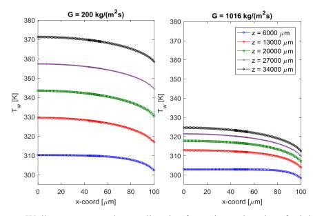
Figure 6.6: Wall temperatures along *x*-direction for various *z*-locations for inlet mass fluxes of 200 kg/(m<sup>2</sup>s) and 1016 kg/(m<sup>2</sup>s).
