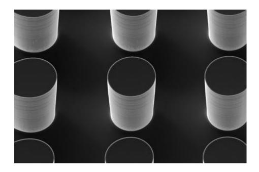
Figure 2.6: Image of the micro pin fins used in [73].
