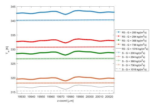
Figure 6.91: Wall mean temperature distribution over the middle roughness element set of RDC configuration.
