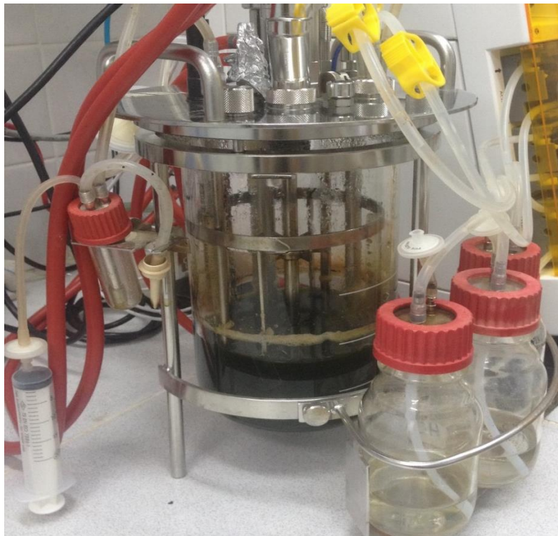
Figure 4.30. Cultivation of Micractinium sp. ME05 cells in 2-L bioreactor with 1-L working volume under heterotrophic conditions.
