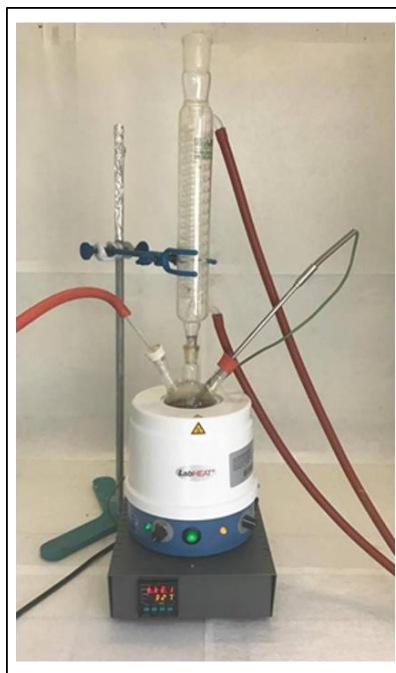
Figure 11. Image of experimental set up of thermal decomposition method
