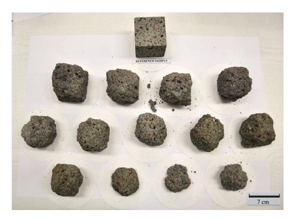
Figure 5.40 Disintegration of some of the vesicular basalt samples after 16<sup>th</sup> cycle of the salt crystallization test
