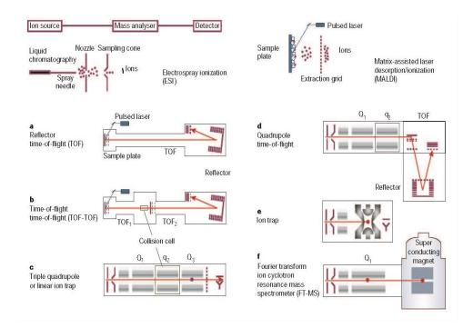
Figure 1.8. Mass spectrometer with different ionization sources and instrumental configurations with different analyzers (a-f) (Aebersold and Mann, 2003)
