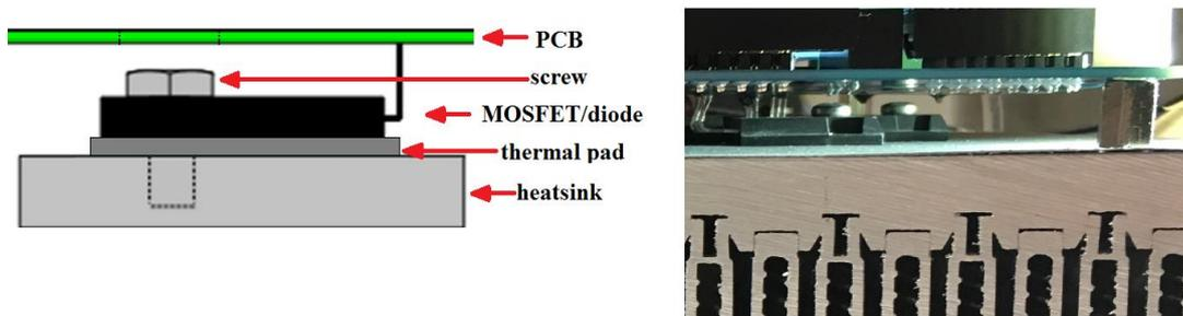
Figure 3.10 Mechanical and electrical connections of the semiconductors
