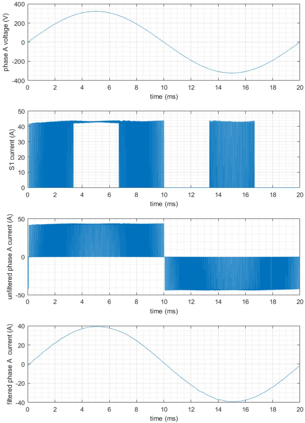
Figure 3.24 Current waveforms of phase-A for one power cycle at unity power factor,  $I_{dc}=42A$  and  $m=0.9$
