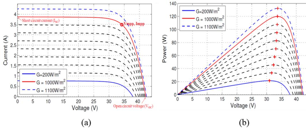
Figure 2.6 (a) I-V Characteristics of a small PV module, (b) MPP vs solar insolation
