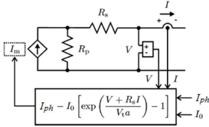
Figure 3.3 PV module equivalent simulation model
