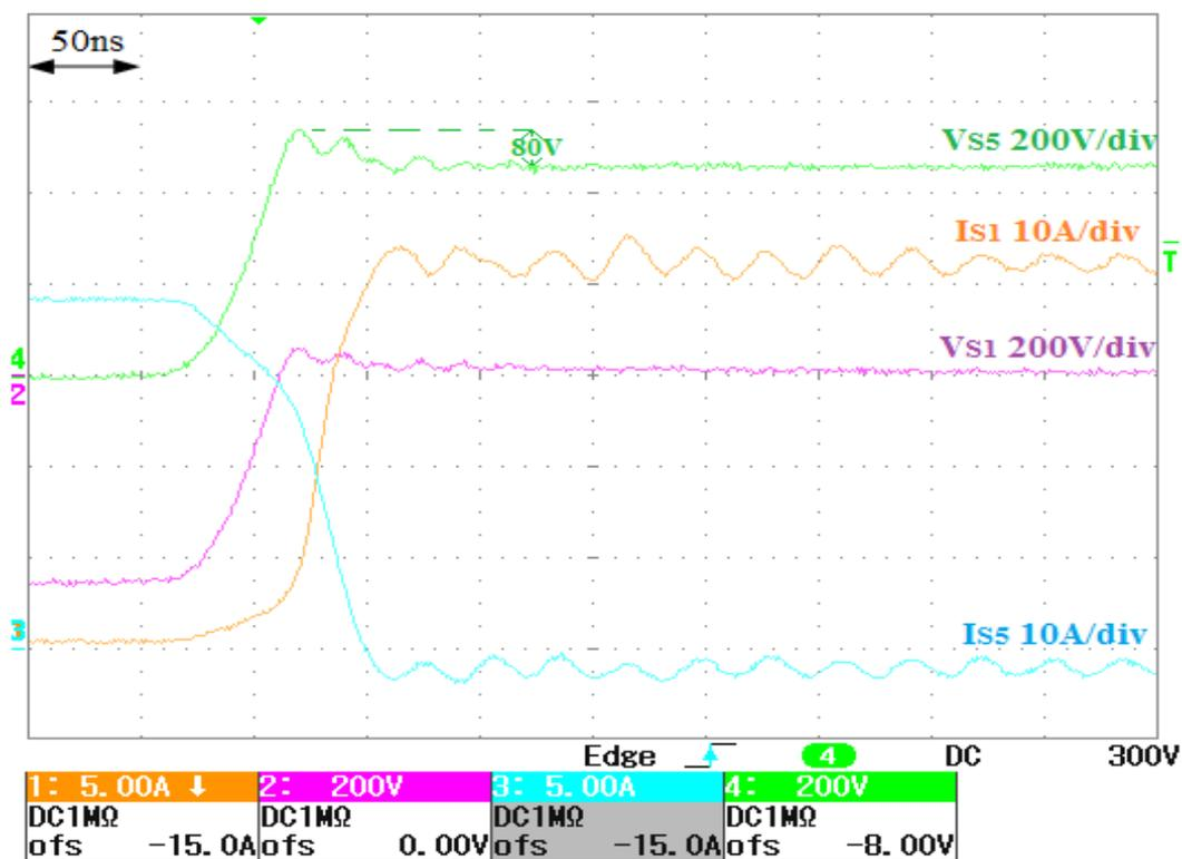
Figure 4.4 Switching waveforms belong to the S5 to S1 commutation event, Ch1: S1 current (orange, 10A/div), Ch2: S1 voltage (pink, 200V/div), Ch3: S5 current (blue, 10A/div), Ch4: S5 voltage (pink, 200V/div), time scale 50ns/div, sampling rate 1 GS/s
