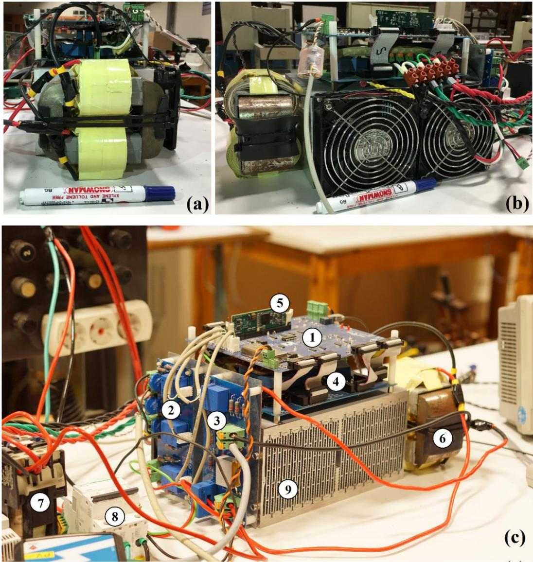
Figure 3.31 20 kVA, three-phase PV-CSI prototype a) side view, b) back view, c) front view
