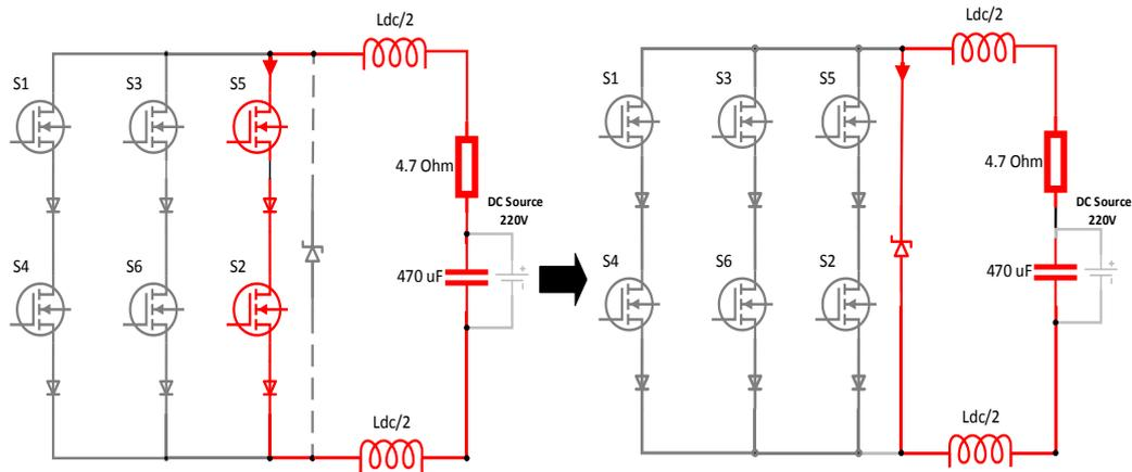
Figure 4.6 Test of overvoltage protection circuit
