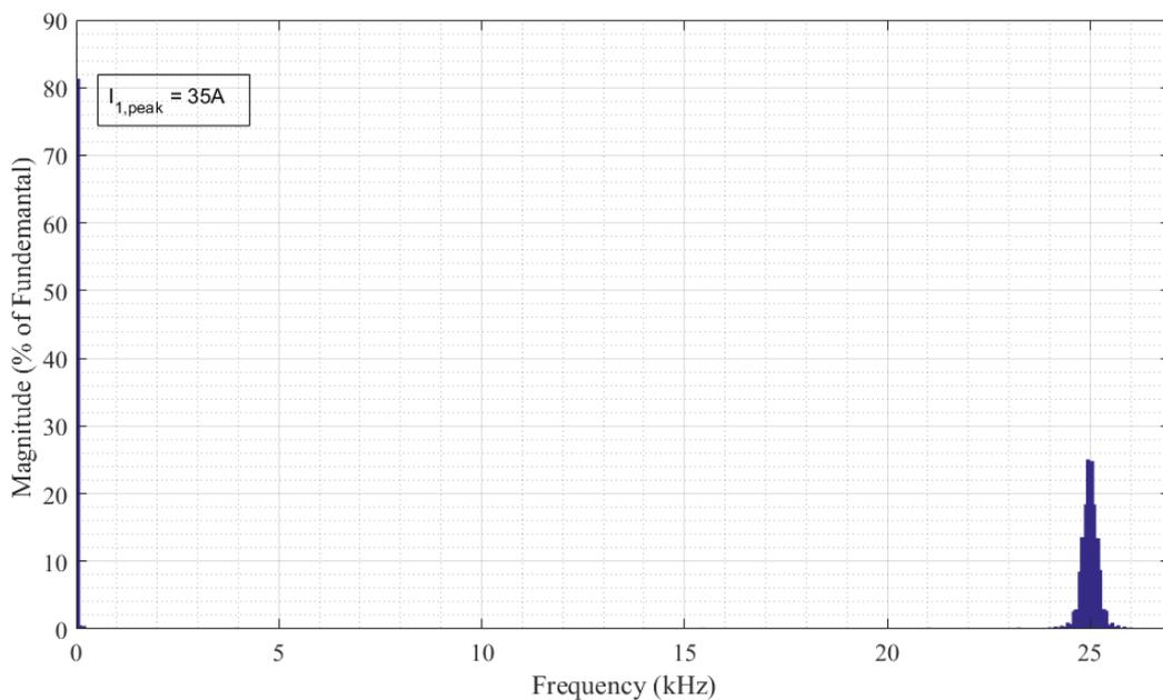
Figure 3.16 Harmonic spectrum of the converter currents ( $I_{cnv}$ ) for  $f_{cr} = 25$  kHz,  $m=0.8$  and  $I_{dc}=42$ A
