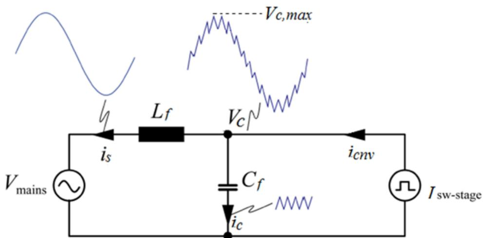
Figure 3.17 Idealized current waveforms for filter elements
