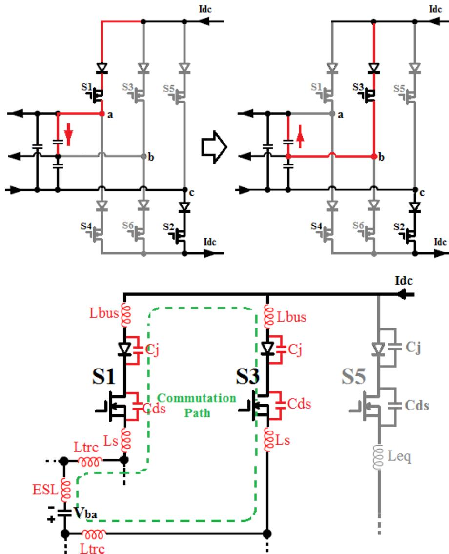
Figure 3.32 (a) Current path before (left) and after (right) S1 to S3 commutation, (b) commutation path for S1-S3 commutation events including parasitic components
