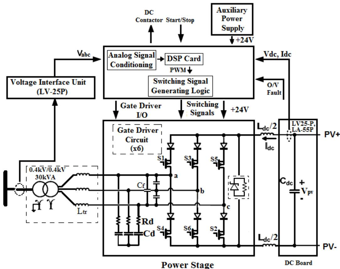
Figure 3.30 Simplified structure of the PV-CSI prototype
