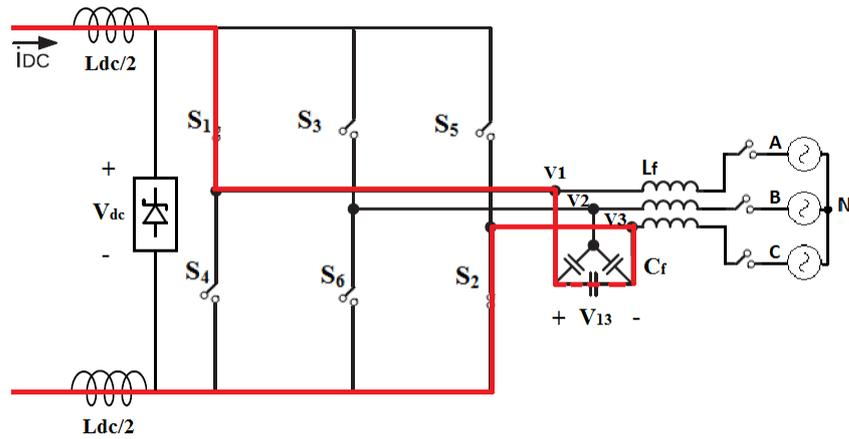
Figure 3.28 Equivalent circuit for mains disconnection
