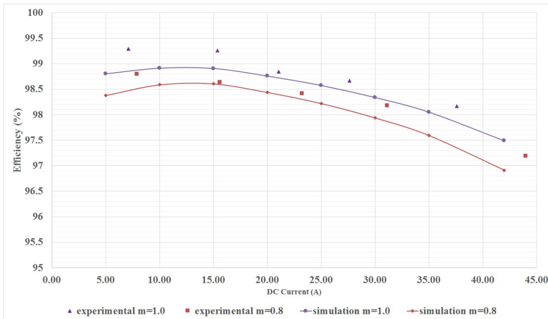
Figure 4.17 Measured and calculated efficiencies of PV-CSI at different DC-link current values for  $m=1.0$  and  $m=0.8$
