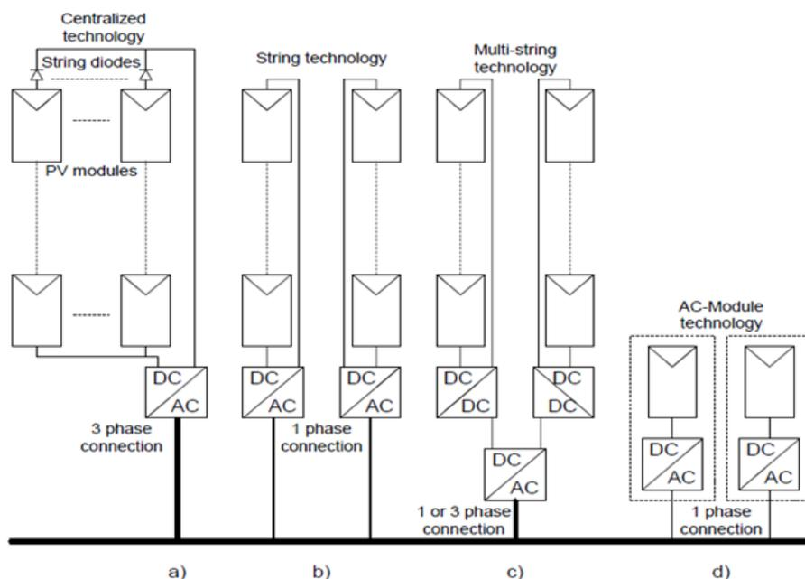
Figure 1.3 Photovoltaic system technologies. a) centralized technology, b) string technology, c) multi-string technology, d) AC-Module technology [7]
