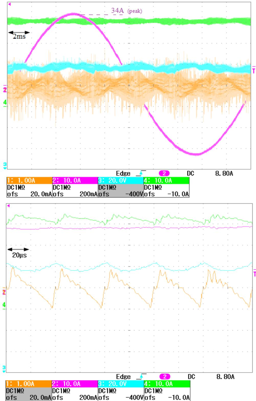
Figure 4.8 DC-link waveforms at  $I_{pv}=42A$  and  $m=0.85$ , Ch1: AC component of  $I_{dc}$  (orange, 1A/div), Ch2: phase A current (pink, 10A/div), Ch3:  $V_{pv}$  (blue, 10V/div, offset=-400V), Ch4:  $I_{dc}$  (DC+AC)(green, 10A/div), (upper: 2ms/div, 25MS/s, lower: 20us/div, 1GS/s)
