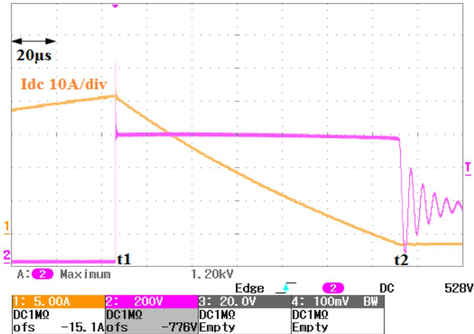
Figure 4.7 Overvoltage protection waveforms in case of an inductor current interruption, inductor current (Ch1:orange, 10A/div), DC-link voltage (Ch:2, pink, 200V/div), time scale  $20\mu\text{s}/\text{div}$
