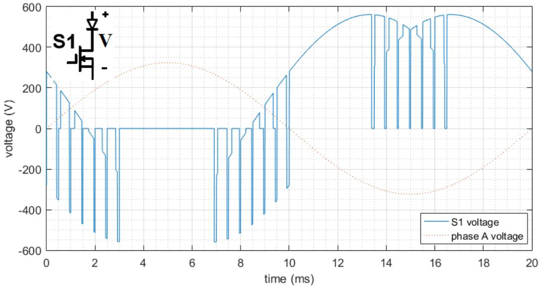
Figure 3.5 Switching voltages of S1 during one grid cycle at unity power factor for  $m=0.9$  and  $f_{cr}=2$  kHz
