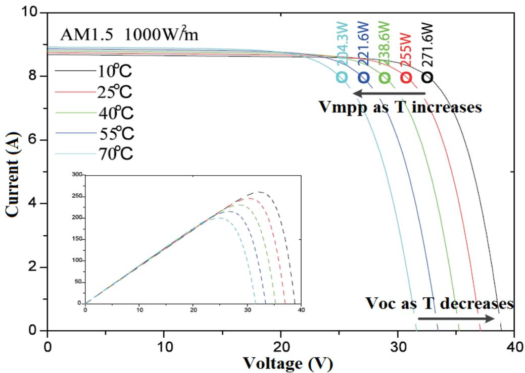
Figure 2.7 I-V characteristics of a PV module at different PV cell temperatures [45]
