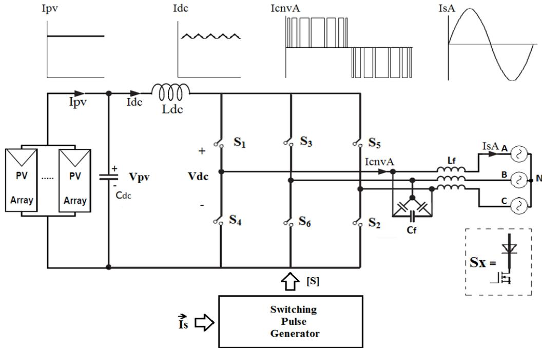
Figure 2.12 Pulse width modulation of output AC currents
