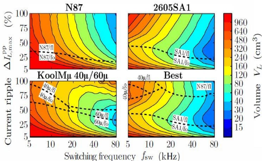
Figure 3.12 Achievable minimum volumes at fixed power loss for powder core (KoolM $\mu$ ), Ferrite (N87) and tape wound (2605SA1) core materials [60]
