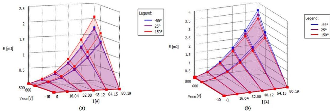
Figure 3.6 Look-up table for switching losses a) turn-off losses b) turn-on losses
