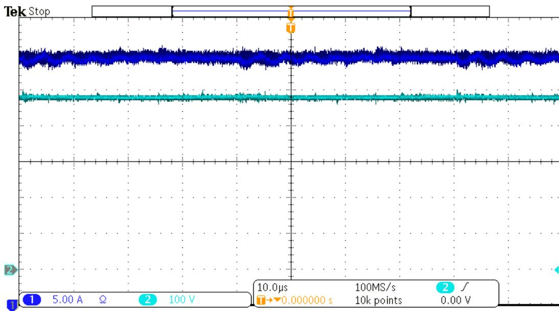
Figure 4.10 PV array voltage and current waveforms at rated DC-link current and for  $m=1.0$
