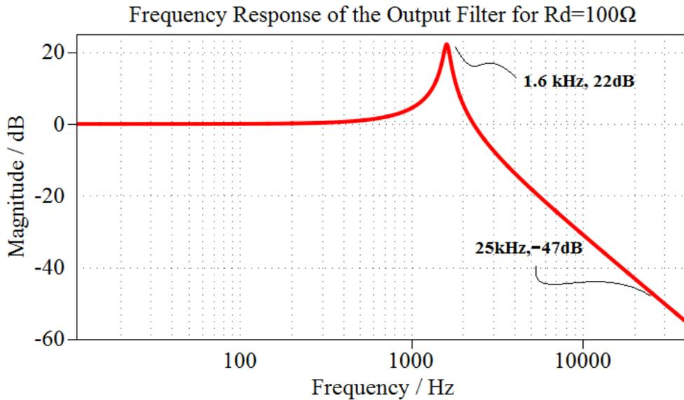
Figure 3.22 Frequency response of output filter for  $R_d = 100 \Omega$
