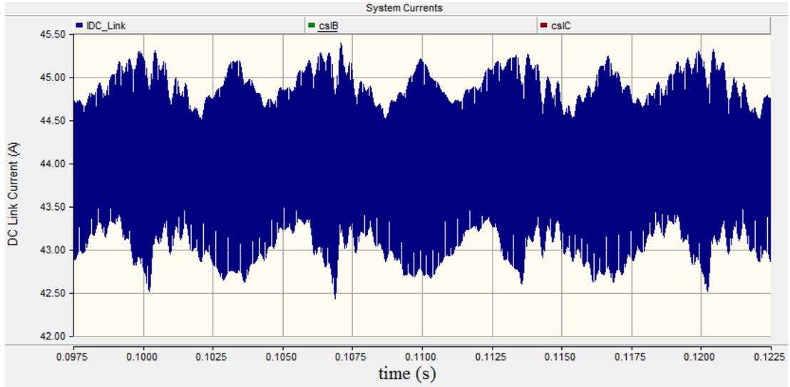
Figure 3.15 DC-link ripple current variation for  $m=0.8$  during one grid period (PSCAD)
