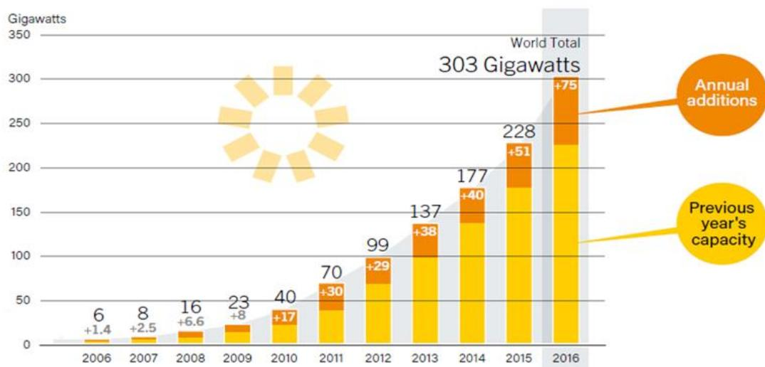
Figure 1.2 Solar PV Global Capacity and Annual Additions, 2006-2016 [3]
