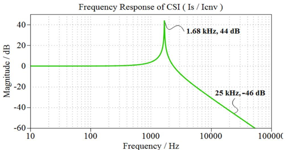
Figure 3.19 Frequency response of undamped output filter
