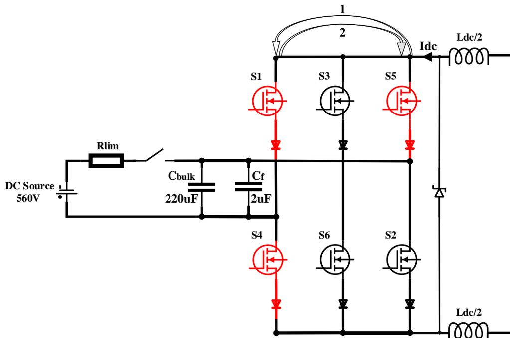
Figure 4.3 Switching test setup
