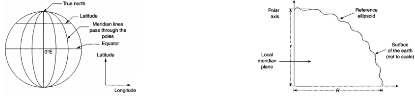
(a) Latitude and Longitude Representations [51] (b) Semi-major and Semi Minor Axes of Earth [51]
