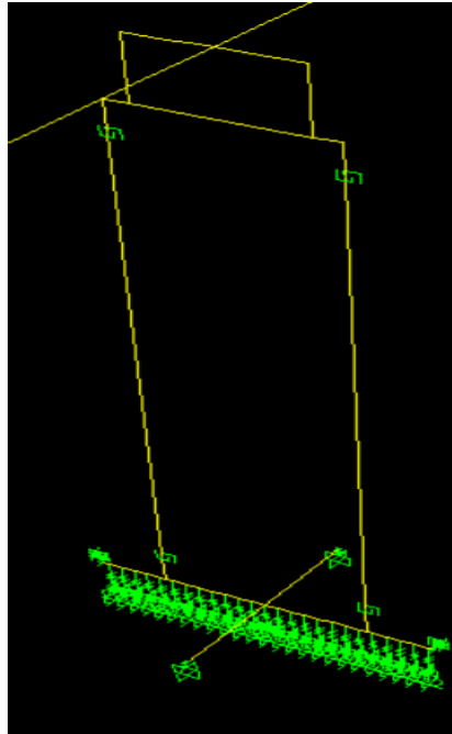
Figure 24. Takeda Link on Multi-Column Pier Bent
