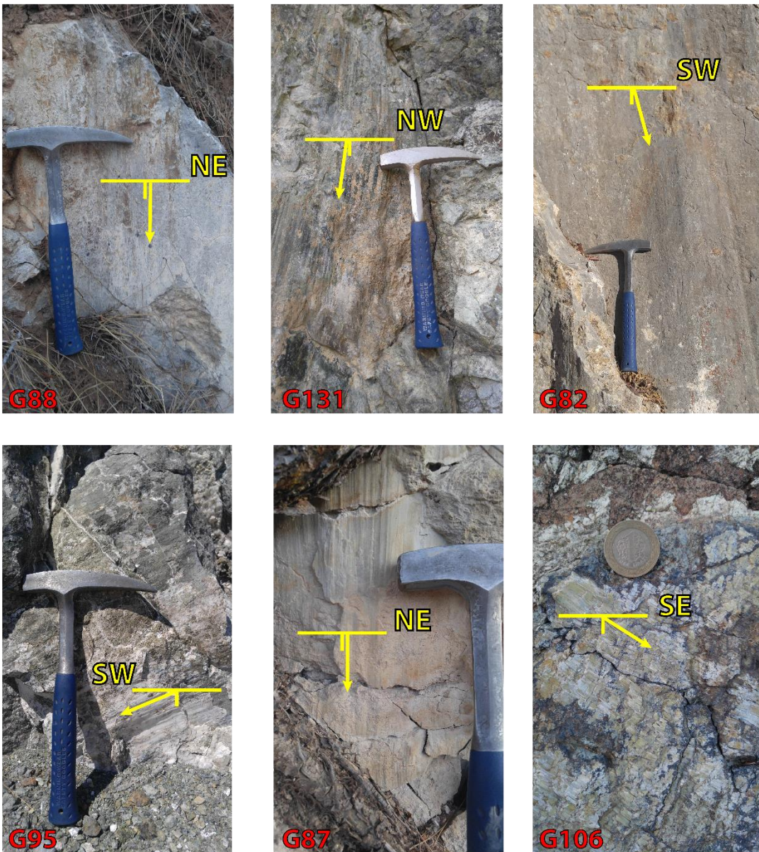
Figure 6 Slickenside lineations on fault planes. Arrows indicate the sense of slip on fault planes.
