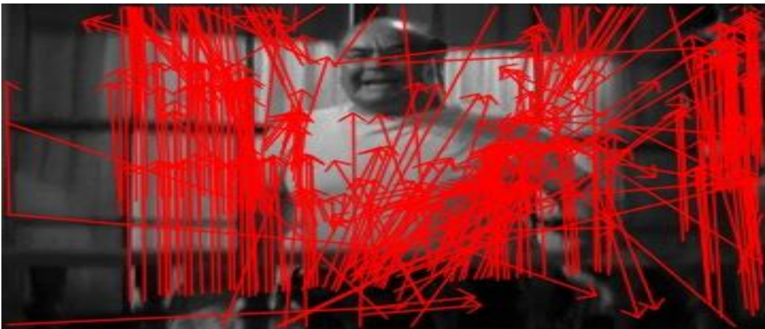
Figure B.2: Optical flow vectors for the sample consecutive frames of the StandUp action
