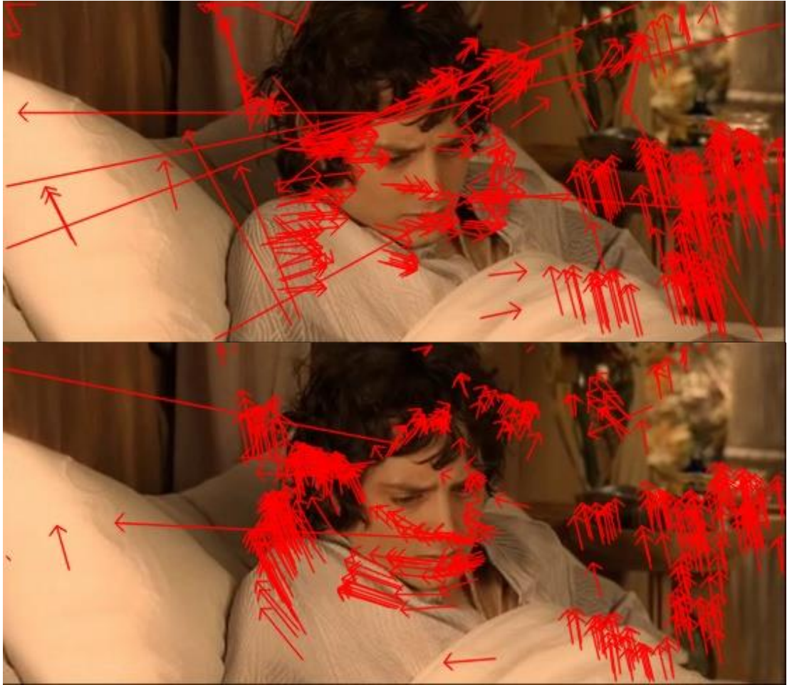
Figure B.10: Optical flow vectors for the sample consecutive - three - frames of the SitUp action
