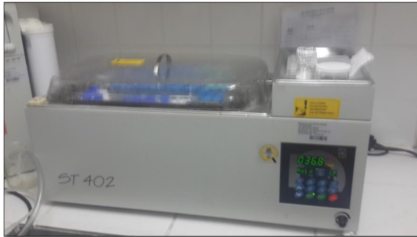
Figure 14 The shaker used for biomimetic coating.
