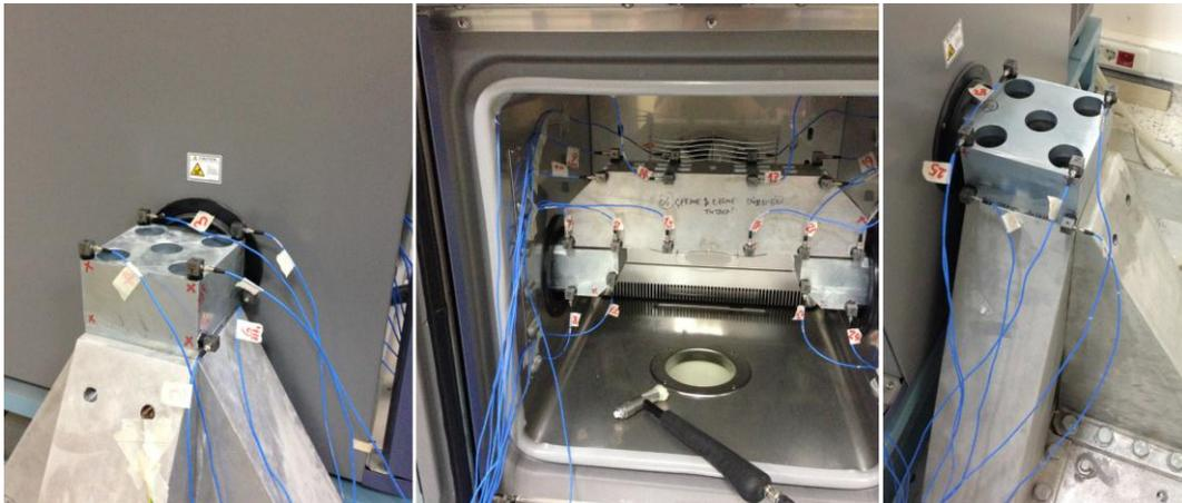
**Figure 62.** Modal test configuration of test fixture
