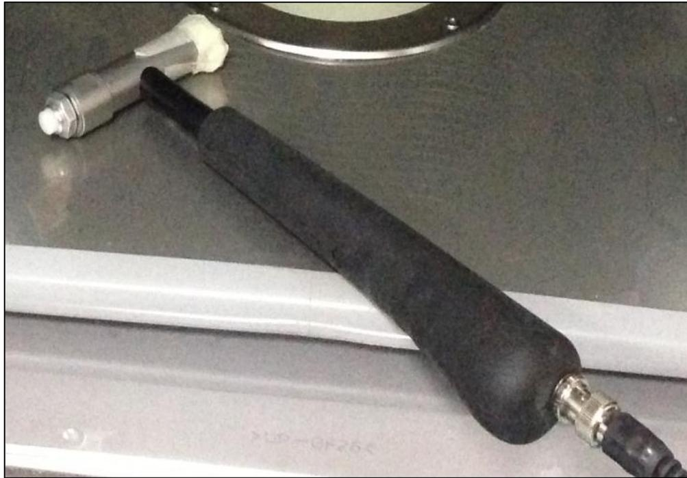
**Figure 61.** Impact hammer with plastic tip
