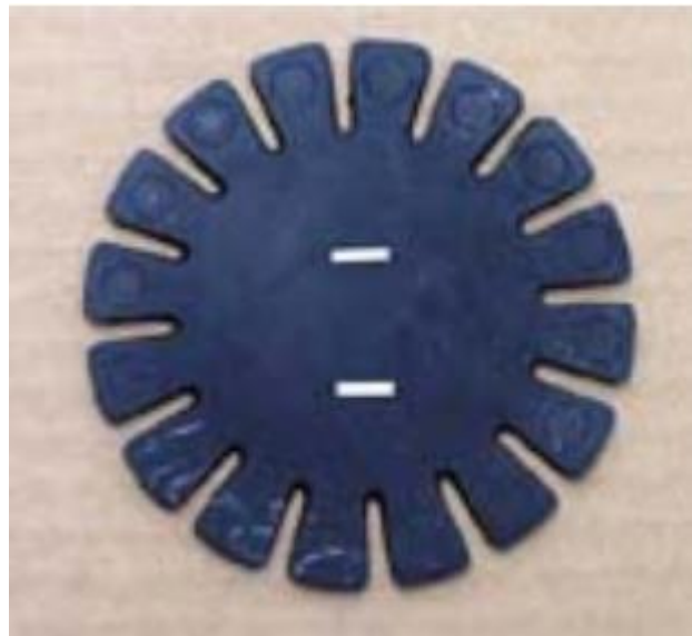
Figure 2.6: Test specimen produced for equibiaxial tension test [8]
