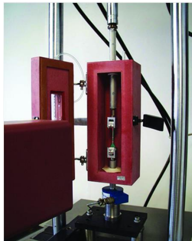
Figure 2.5: Uniaxial experiment test set-up designed for elastomers [8]
