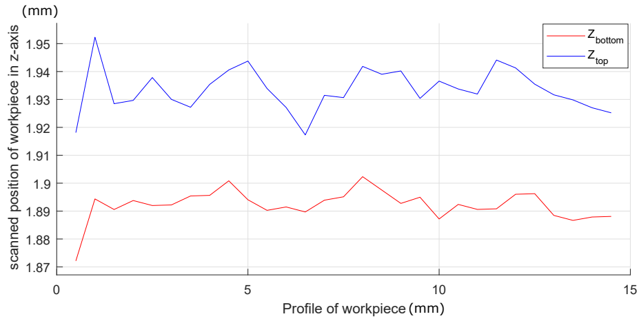
Figure 8.3: Form error due to interaction force of 300 \mu m depth of cut
