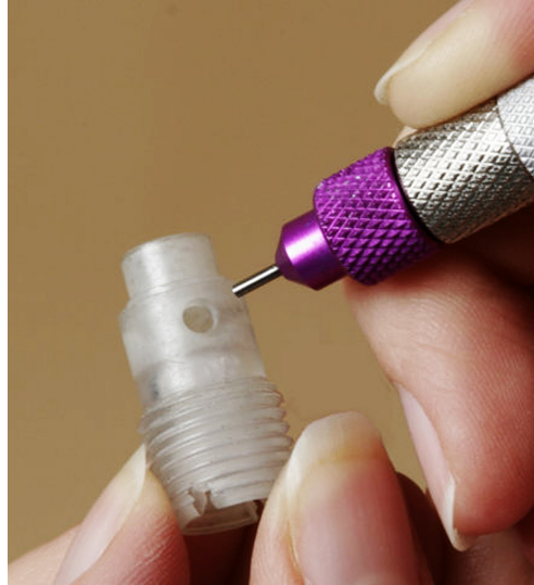
Figure 1.1: Manual deburring process on medical component
