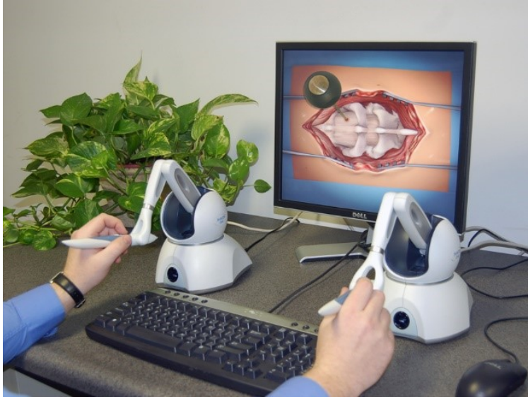
Figure 3.1: Two haptic devices are being used for surgery in virtual environment subject of "General concentrated position DMPs" is related to 6DOF haptic device and "Local DMPs" is related to 1DOF haptic device. These concepts are explained in chapter 5 and chapter 6 respectively.
