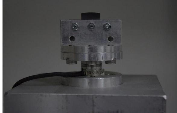
Figure 3.3: A close up of workpiece, F/T sensor, and the heavy metal block
