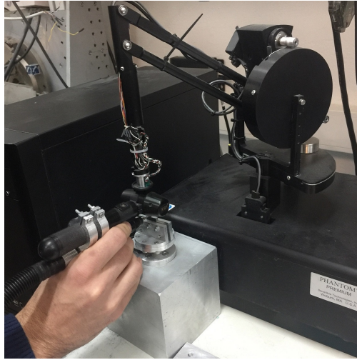
Figure 8.10: Participant holding spindle of 6-DOF haptic device
