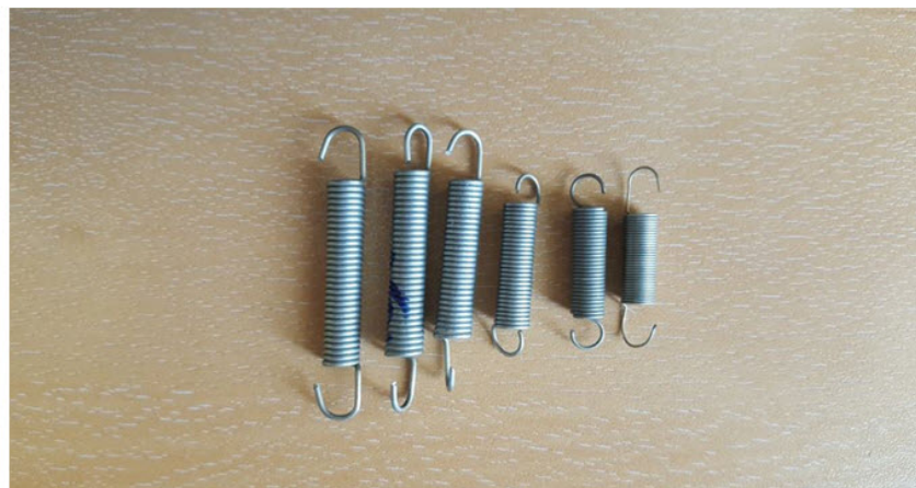
Figure 2.18: Selected Tension Springs
