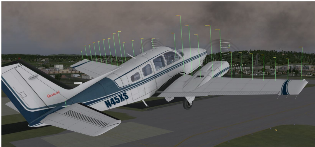
Figure 2.1: Illustrating the forces acting on a Baron 58[20]
