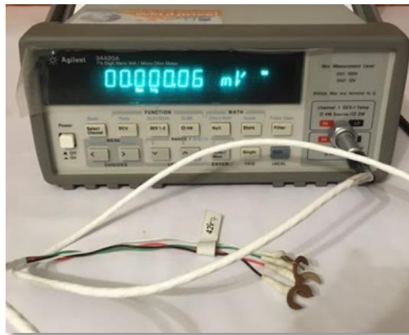
Figure 35 Nanovolt, Micro Ohm Meter (METU Central Lab.)
