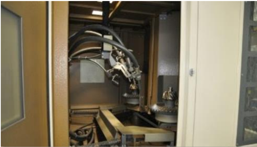
Figure 28 Shot peening equipment (TAI)
