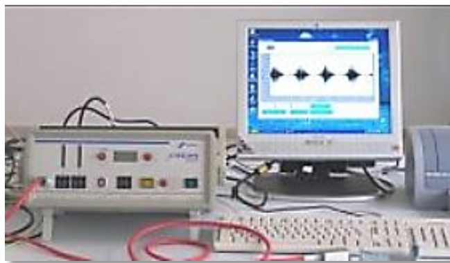
Figure 32 Stresstech MBN System (METU Central Lab.)
