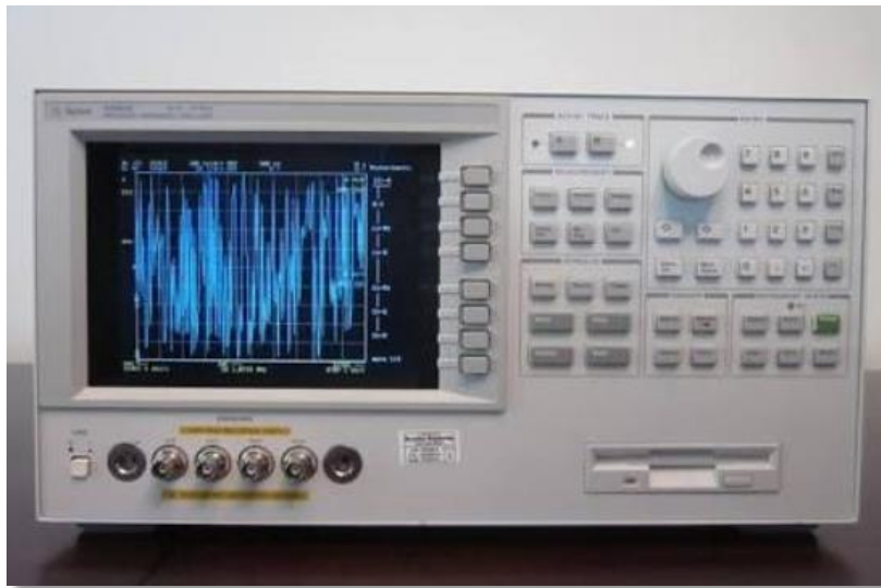
Figure 36 Precision Impedance Analyzer (METU Central Lab.)
