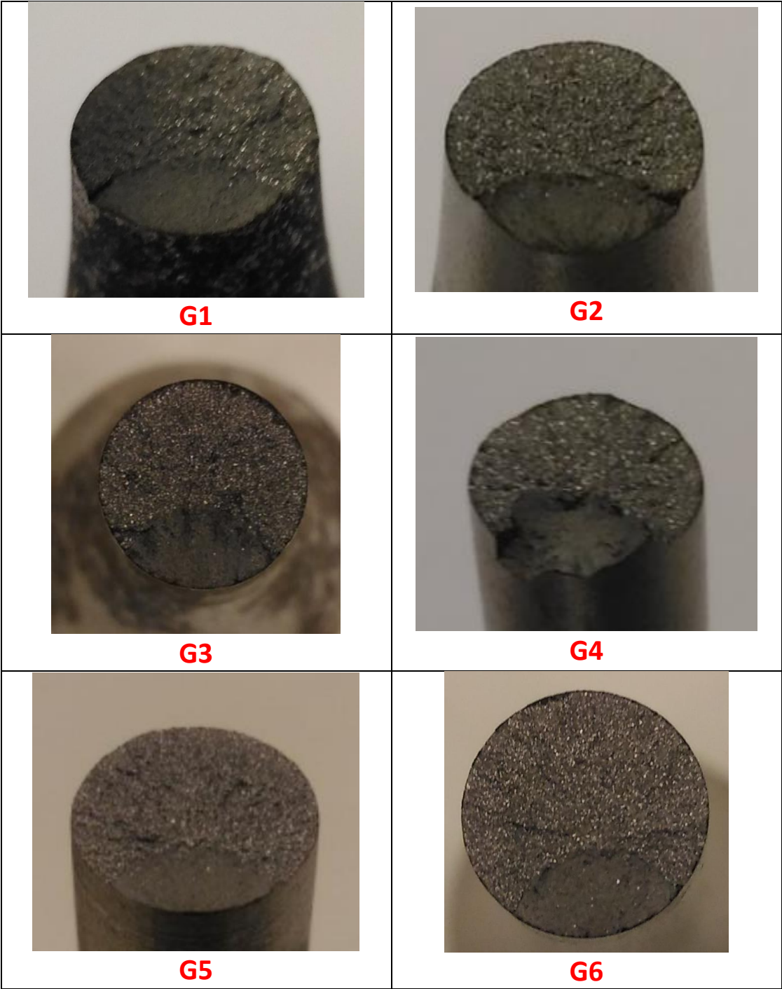
Figure 53 Representative fracture surfaces for each sample group
