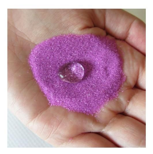
Figure 1.1. Hydrophobic Sand
