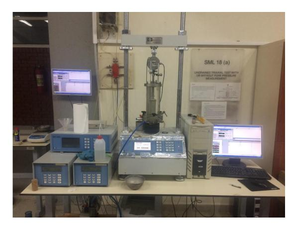
Figure 3.10. Triaxial testing system used in this study
