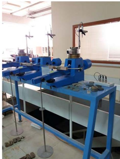
Figure 4-19 Consolidation test setup
