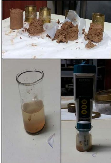
Figure 4-20 Pore water conductivity measurement by the EC probe
