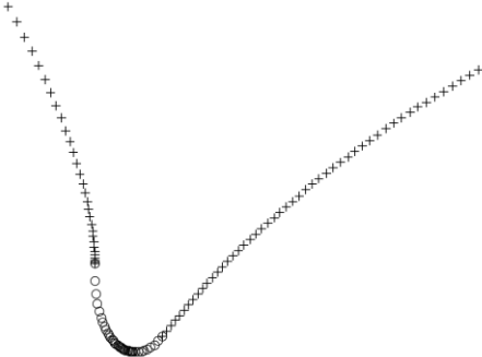
Fig. 2.22 External asymmetric spur gear tooth space profile
