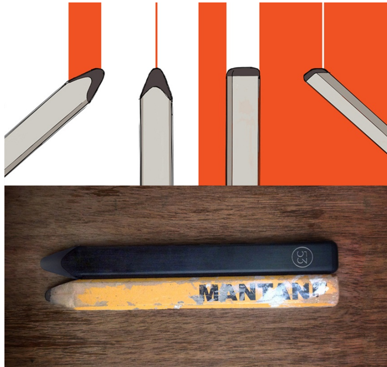
Figure 26: Above: 53 Pencil's pressure sensitivity, tilting recognition and eraser demonstrated. Below: the same tool versus a carpenter pencil (Collage by author)
