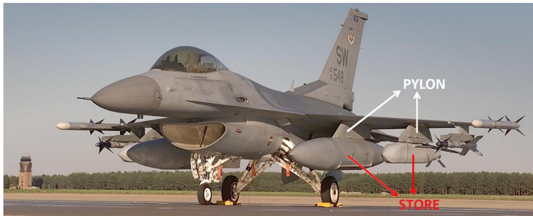
Figure 4. A F-16 jet fighter full of stores mounted under its wings via pylons
