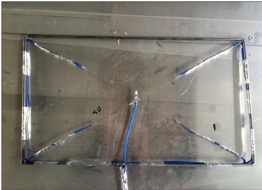
Figure 2.2 Planes with thermocouples attached
