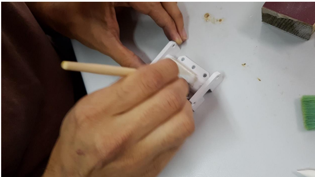
Figure 4.13: Painting process of test piece
