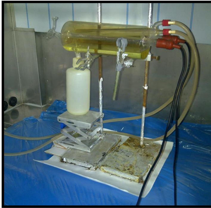
Figure 3.7 Sub-boiling distillation unit
