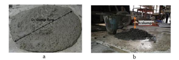
Figure 4.1: a) Slump and b) Slump flow of fresh concrete.
