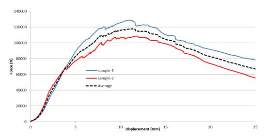
Figure 4.8: Force deflection graph of HPFC 24 square panel samples
