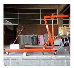
Figure 3.6: Engine crane
