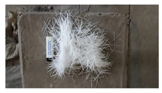
Figure 3.1: Polypropylene fiber used
