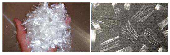
a) Monofilament Fibers
