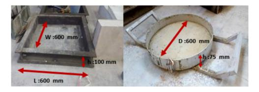
Figure 3.3: Square and round panel molds W: Width, L: Length, h: Height, D: Diameter.
