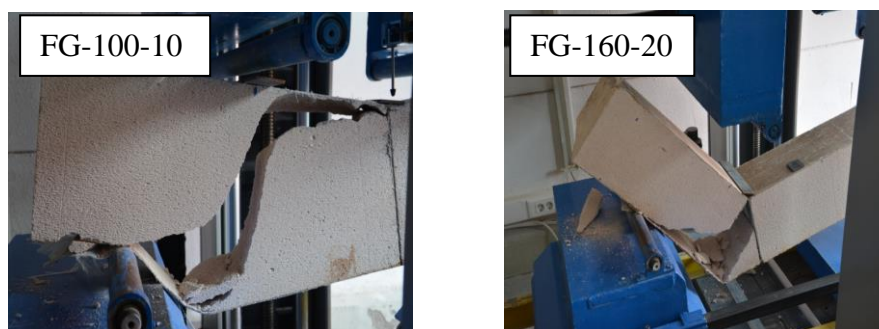
Figure 2.21: Failure modes of Group-C specimens
