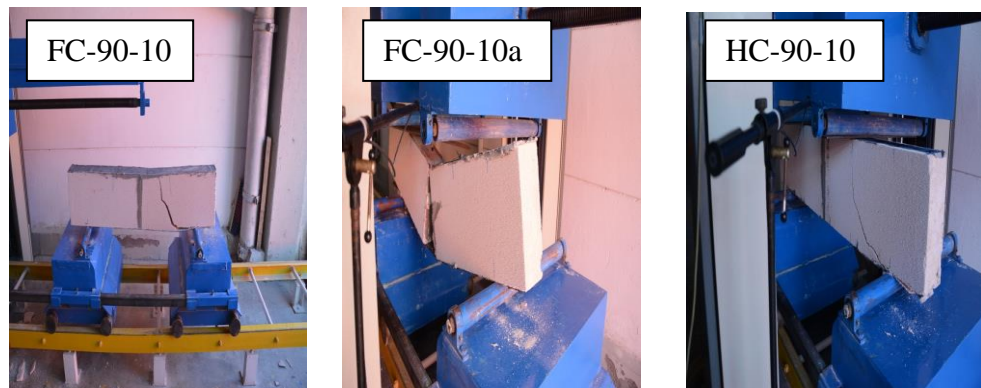
Figure 2.13: Failure modes of Group-B1 specimens
