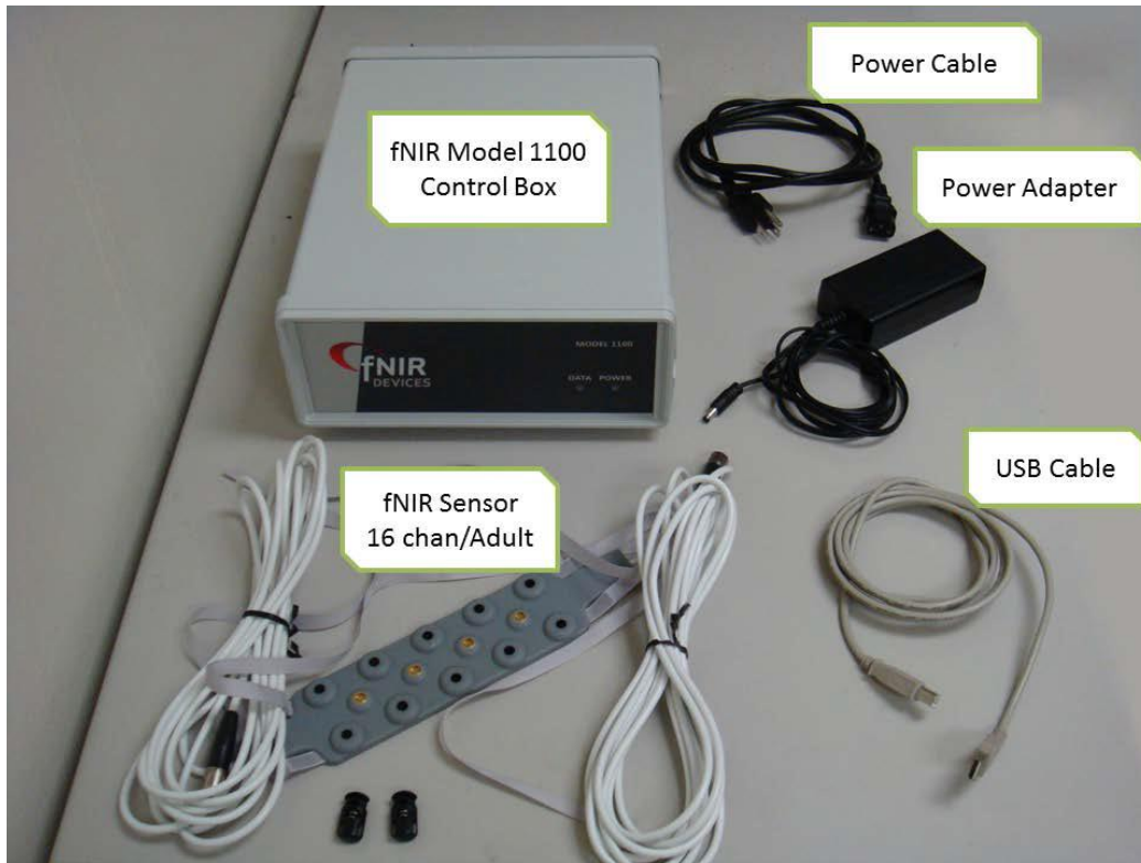
Figure 12: fNIR Model 1100 system
