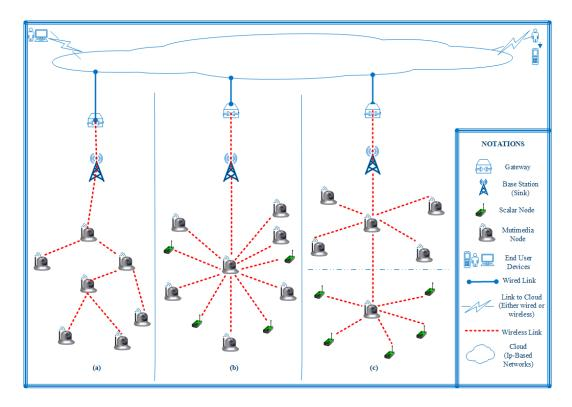
Figure 1.2: An exemplary schema of a WMSN: a) A homogenous single-tier network,b) A heterogeneous single-tier network, c) A heterogeneous multi-tier network.
