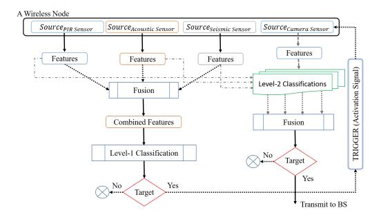
Figure 5.1: The research project system architecture.
