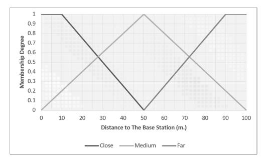
Figure 3.2: The fuzzified parameter Distance to The Base Station.
