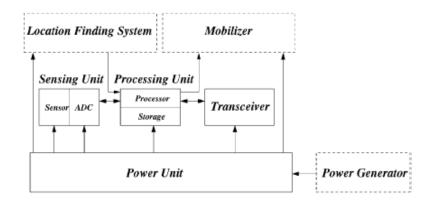
Figure 1.1: A reference component schema of a wireless sensor unit [1].
