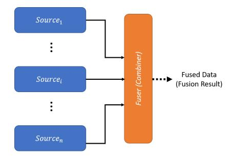
Figure 2.2: A flow of general data fusion procedure.
