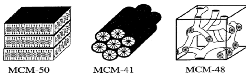
Figure 6 Schematic diagram of the M41S materials: MCM-50 (layered), MCM-41 (hexagonal) and MCM-48 (Cubic) mesoporous silica particle structures (Alothman, 2012).
