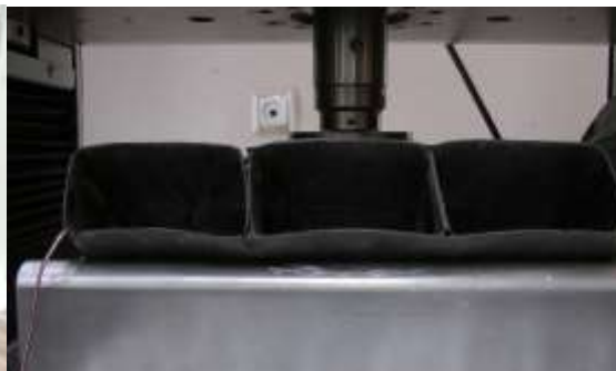
Figure 122. Ultimate skin failure
