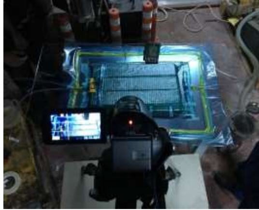
Figure 70. Photograph of vacuum bagged assembly during infusion
