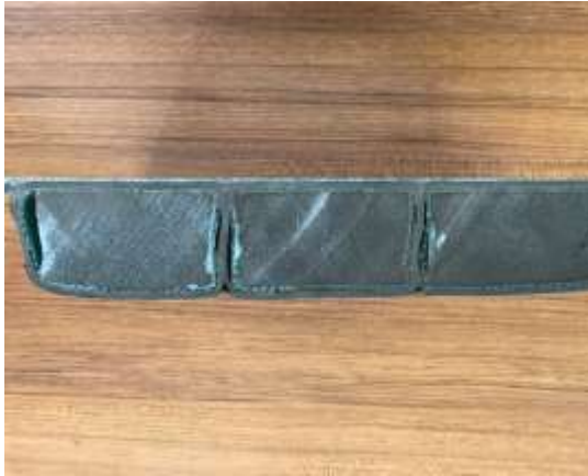
Figure 73. Photograph of Experiment No.2 before foam removal (Type 1, coated, 80°C-8h)
