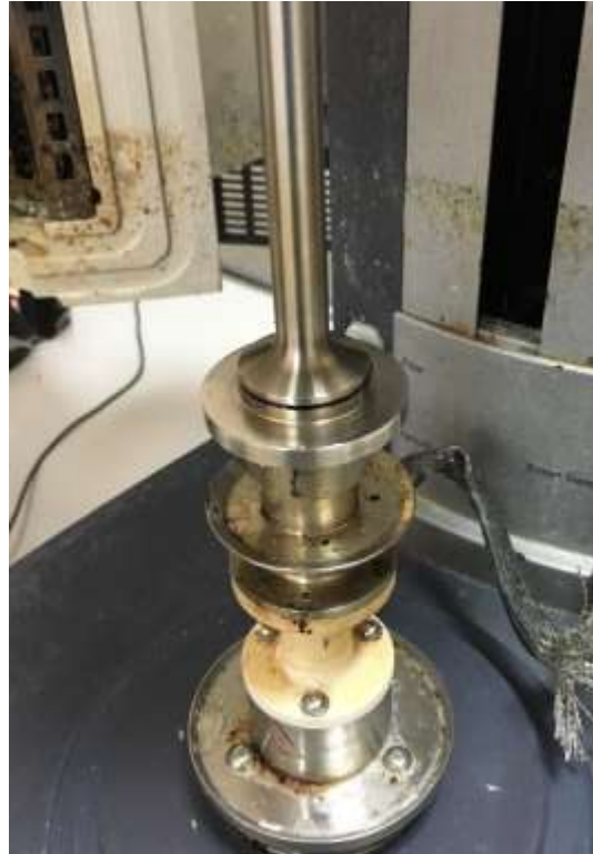
Figure 20. Rheometer parallel circular plates
