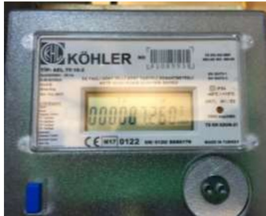
Figure 125. Photograph of electrical meter after the curing process
