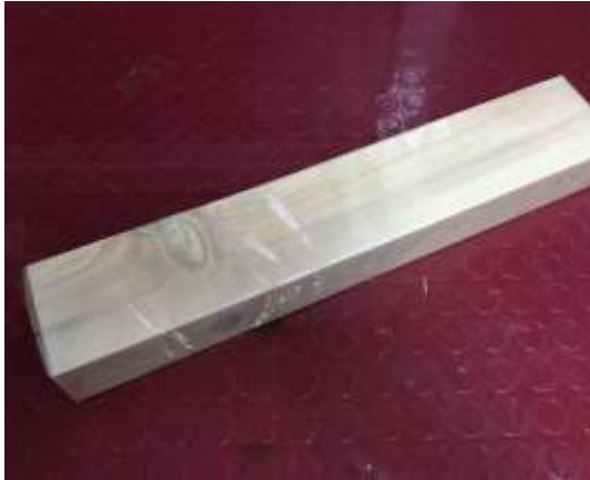
Figure 86. Curing tool for skin-web assembly
