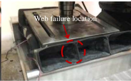
Figure 120. left web failure
