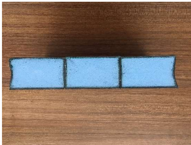
Figure 76. Photograph of Experiment No.3 before foam removal (Type 2, coated, 40°C-8h)
