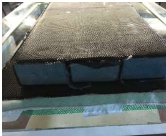
Figure 67. Placement of three mold pieces over the mold surface
