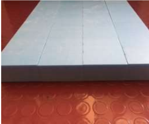
Figure 61. Foam molds coated with epoxy resin
