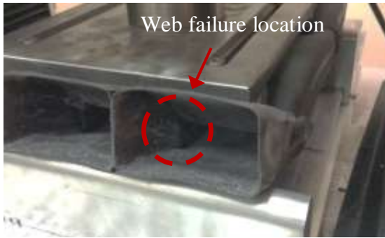
Figure 119. Right web failure
