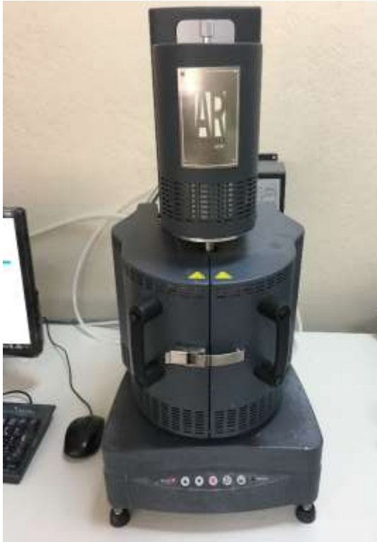
Figure 19. TA Instruments, AR2000 Rheometer
