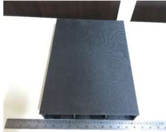
Figure 93. Bonded Three-cell Composite Box Beam
