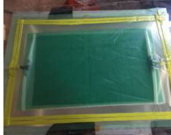
Figure 81. Sealing of whole assembly
