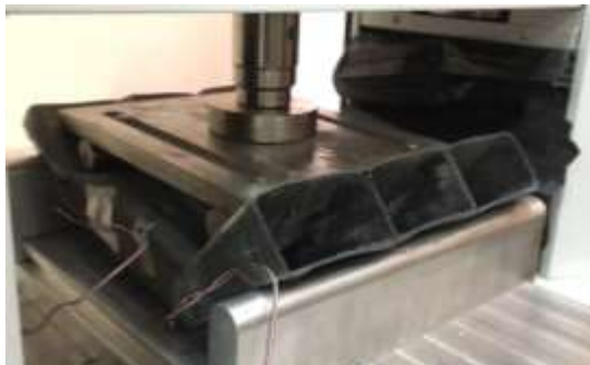
Figure 121. Ultimate skin failure
