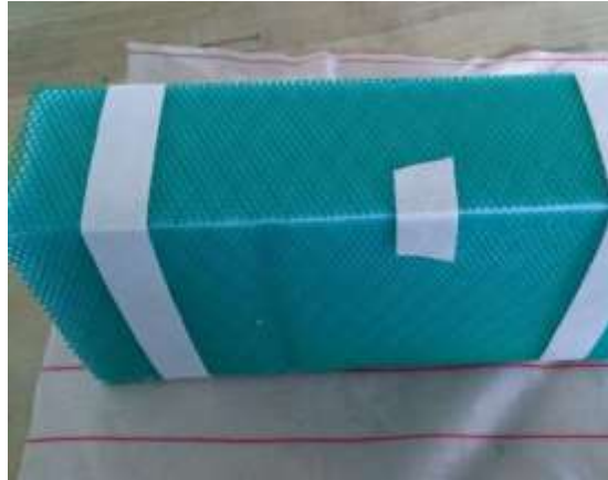
Figure 62. Epoxy coated molds wrapped with distribution media
