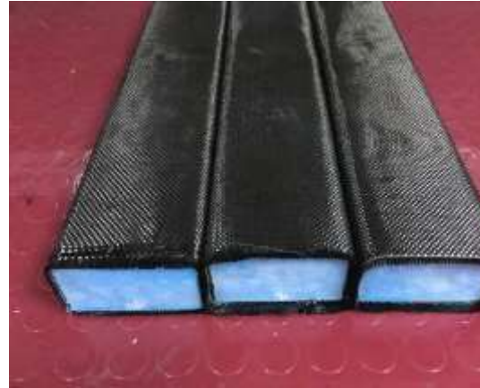
Figure 64. Carbon fiber fabrics are wrapped around the peel ply
