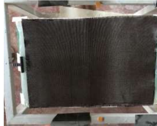
Figure 66. Placement of distribution media, peel ply and carbon fiber fabrics
