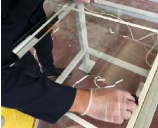
Figure 65. Application of mold release agent
