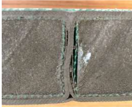
Figure 74. Fiber buckling caused by structurally unstable polystyrene foams
