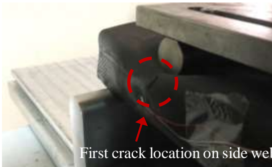
Figure 117. First crack in left-side web
