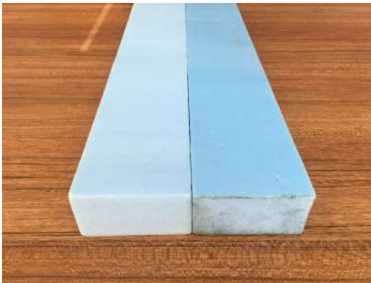
Figure 77. Photograph of Uncoated Foam (Left) and Coated Foam (Right)
