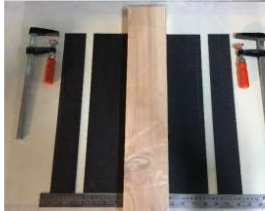
Figure 87. Pre-bonding set-up for the skin- web assembly
