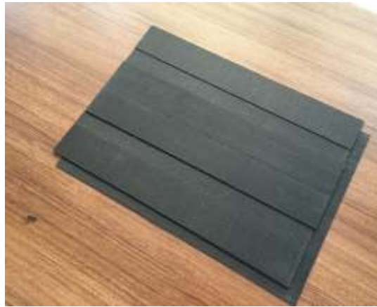
Figure 85. Photograph of shaped carbon fiber composite sub-parts
