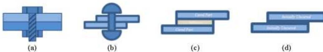
Figure 7. Joining Types of Composites: a) Bolted Joint b) Riveted Joint c) Secondary Bonding d) Co-curing
