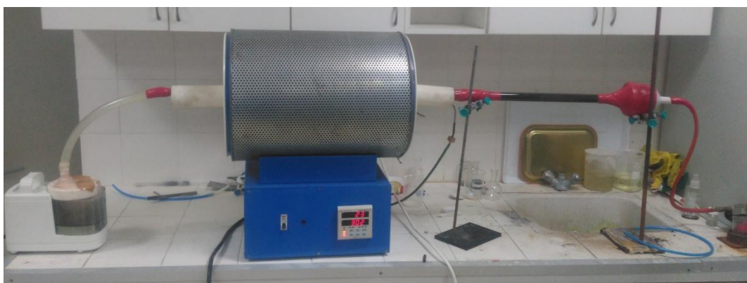
Figure 3.3 USP system used in nanoparticle synthesis in this work.
