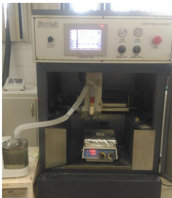
Figure 3.6 A photo of USP thin film deposition device used for thin film coatings in this work.
