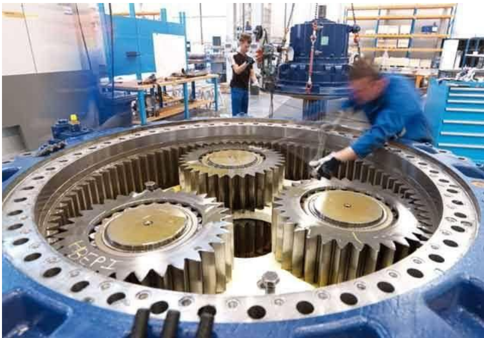
Figure 1-3 Planetary gearbox for a wind turbine [5]
