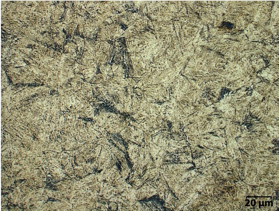
Figure 46 Optical micrograph of the tempered martensite (540°C/4h)
