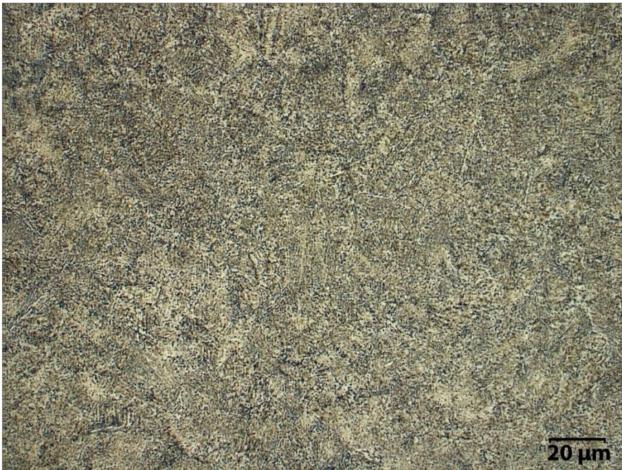
Figure 47 Optical micrograph of the tempered martensite (700°C/4h)
