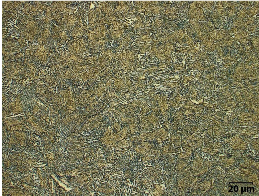
Figure 48 Optical micrograph of lower bainite (400°C/7h)
