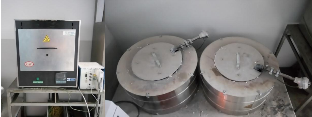
Figure 25 Conventional heat treatment furnace and salt baths with high-temperature range (from left to right)
