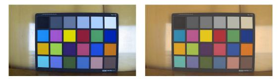
Figure 3.34: The Original Image and the Color Corrected Image for Camera-3
