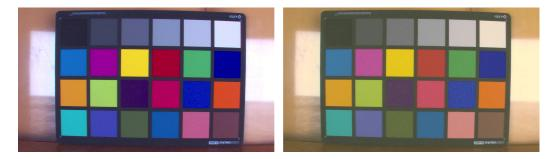
Figure 3.36: The Original Image and the Color Corrected Image for Camera-5
