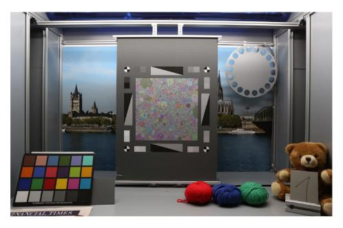
Figure 6.11: The Test Setup Proposed by Image-Engineering GmbH [42]
