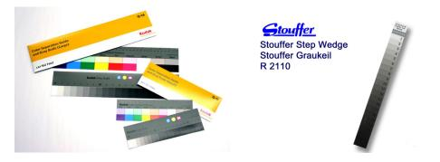
Figure 2.4: Kodak (left) and Stouffer (right) Gray Ramp Test Charts [5] and [6]
