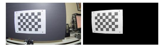
Figure 6.16: A frame (left) and Detected Test Chart (right)
