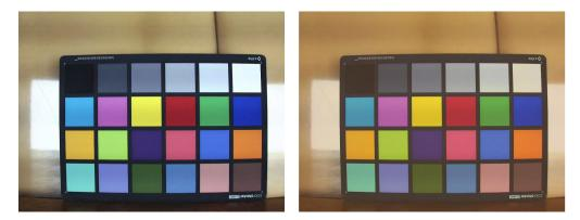
Figure 3.35: The Original Image and the Color Corrected Image for Camera-4
