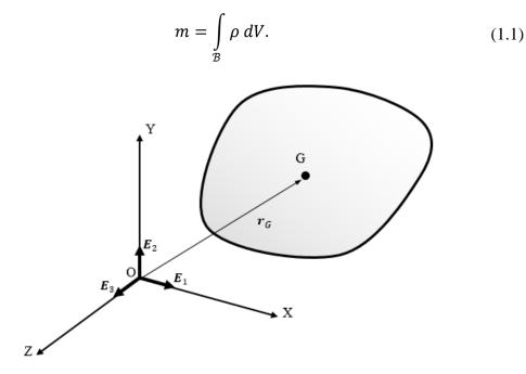
Figure 1. Center of gravity position of the given solid body is defined as  $r_G = x_G E_1 + y_G E_2 + z_G E_3.$
