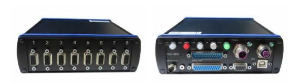
Figure B-3. Front and back sides of the amplifier
