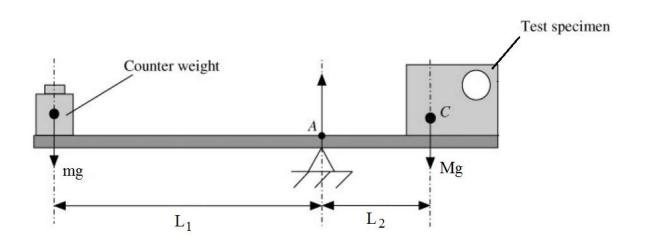
**Figure 16.** Moment balance about point A is used to find the distance between center of gravity position along vertical axis and point A, L<sub>2</sub>. [66]
