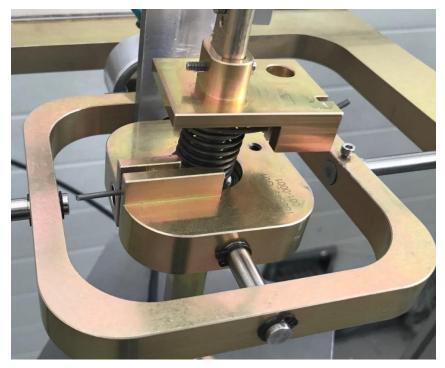
Figure 31. Torsional spring between frame 1 and extension link
