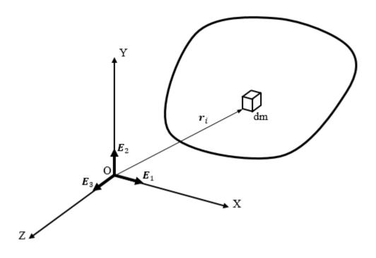
Figure 10. Differential element of mass dm relative to reference coordinate frame is shown.
