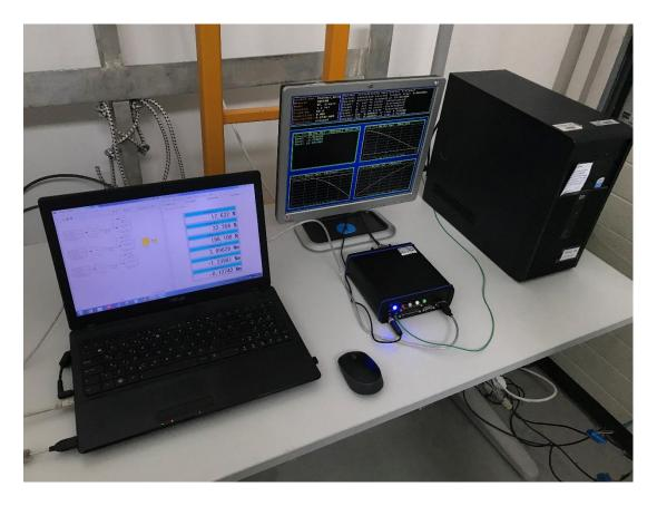
Figure 34. Data acquisition systems for load sensor and encoders
