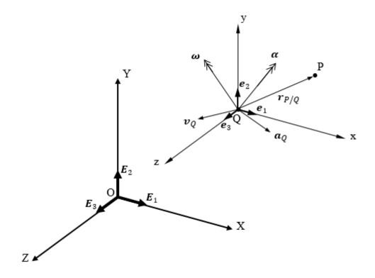
**Figure 7.** Position of point P with respect to translating and rotating coordinate system located at point Q. Translational and rotational motion of this local frame is defined relative to fixed reference coordinate system at point O.
