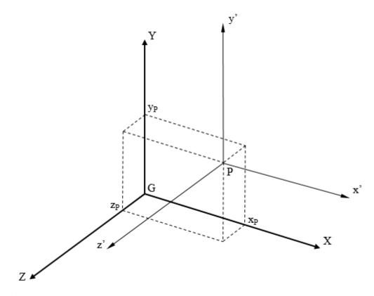
**Figure 12.** Inertia parameters with respect to center of gravity G and arbitrary point P can be correlated by using parallel distances between their axes.
