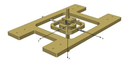
Figure 28. Nested frames and the reference coordinate axes are shown.
