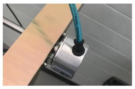
Figure 32. Encoder and connection to the frame is shown.
