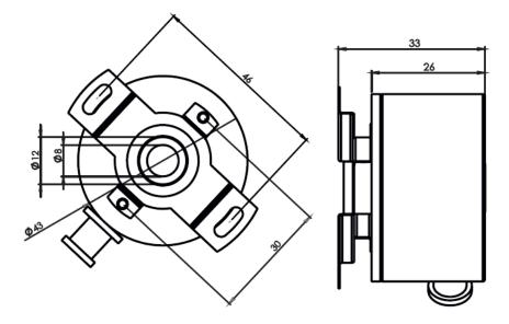
Figure A-2. Dimensions of the rotary encoder
