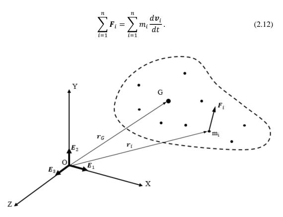
Figure 5. System of particles whose center of mass is located at G and force acting on one particle are demonstrated.
