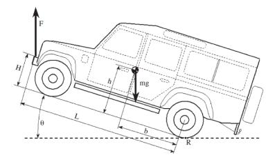
Figure 15. The specimen can rotate about point R. The distance, b, is calculated using moment balance about point R. [10]
