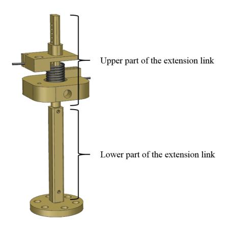
Figure 30. Extension link and connected parts are shown.
