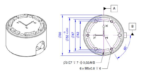
Figure B-2. Dimensions of the load sensor
