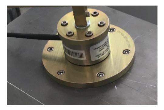
Figure 33. 6-axis load sensor and its connection interfaces
