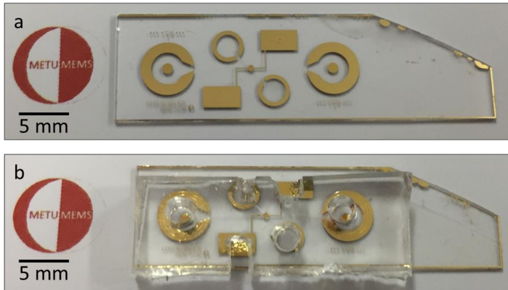
Figure 3.23. a) The fabricated second-generation electrostatic microvalve on the glass wafer and b) the plasma bonded die that includes both microvalve and PDMS microchannel.
