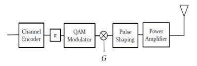
Figure 2.1: Transmitter Side
