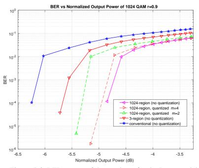
Figure 5.6: BER curves of the receivers for the Rapp model
