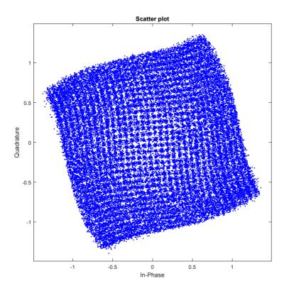
Figure 1.2: 1024 QAM constellation points passed through a power amplifier with the Saleh model
