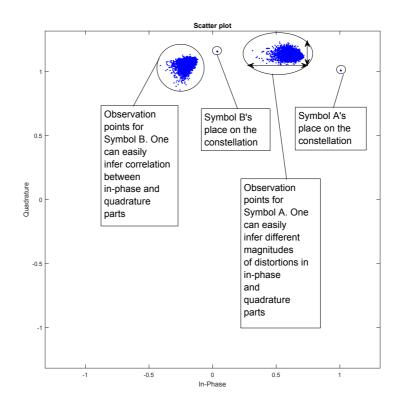
Figure 3.1: Two specific outermost constellation points' observation symbols in the receiver side
