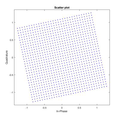
Figure 3.2: Rotation of the 1024QAM constellation with the complex  $\alpha$  or the rotation matrix
