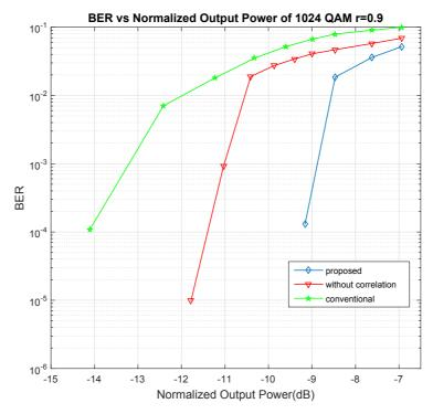
Figure 5.5: BER curves of the receivers with rate 0.9
