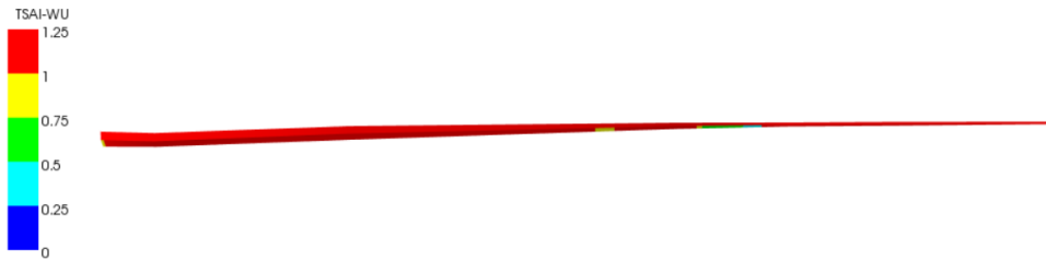
Figure 5.19. Contour plots of Tsai-Wu failure reserve factors in the internal flange at flapwise loading.
