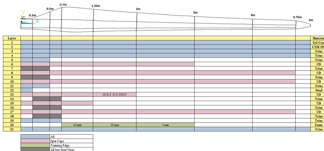
Figure 3.10. Lamination plan of the pressure and suction sides of blade.
