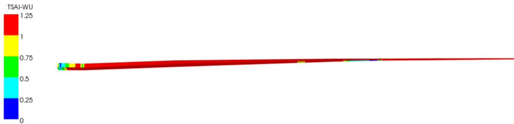
Figure 4.28. Contour plots of Tsai-Wu failure reserve factors in the internal flange at flapwise and edgewise loading.
