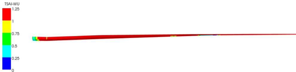
Figure 4.17. Contour plots of Tsai-Wu failure reserve factors in the internal flange at flapwise loading.
