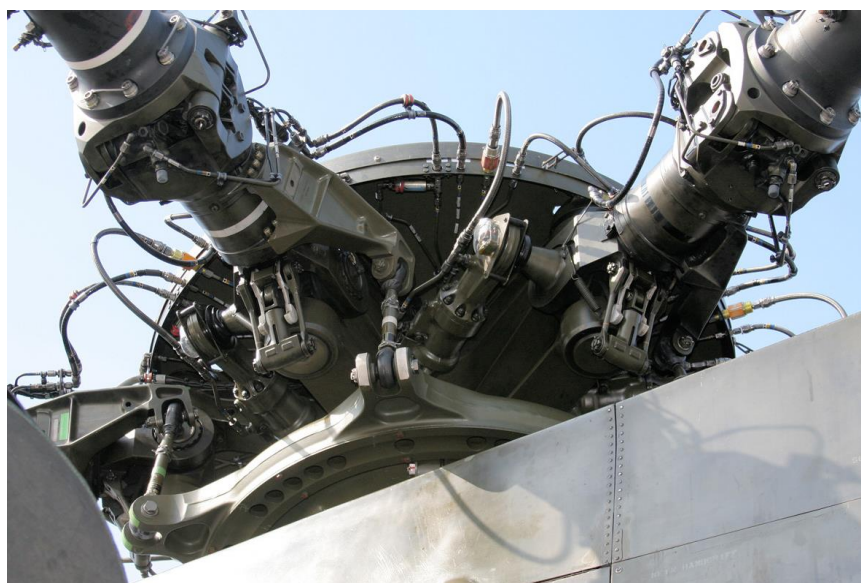
Figure 6 Fully Articulated Main Rotor - Sikorsky CH53G [37]
