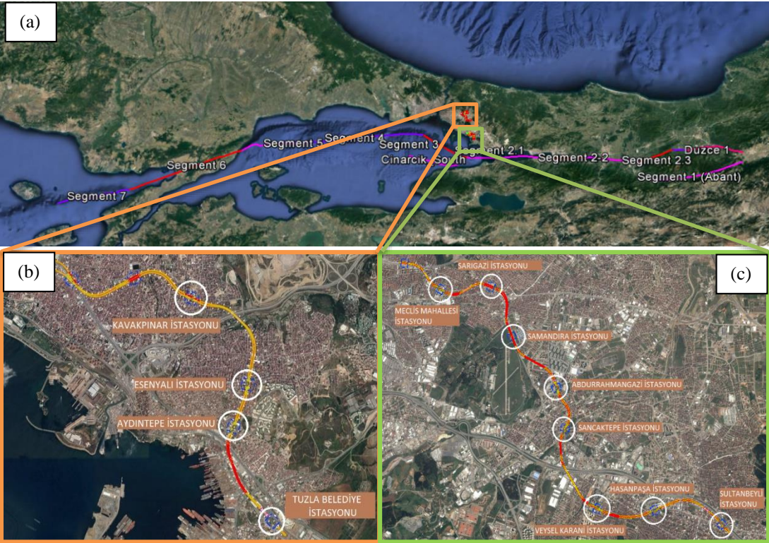
Figure 2.6 (a) Fault system and approximate locations of analyzed metro stations (b) KPT Metro Line and (c) CSS Metro Line
