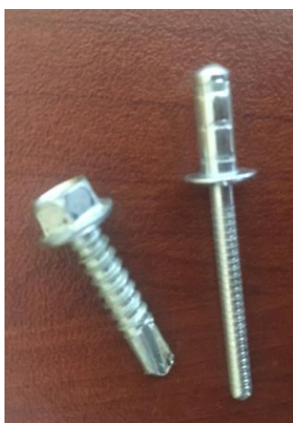
Figure 14. Screw and rivet used in truss specimens
