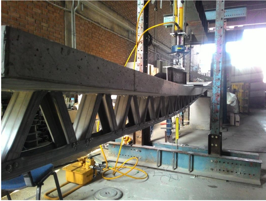
Figure 24. Deformed shape of specimen WB_Slab
