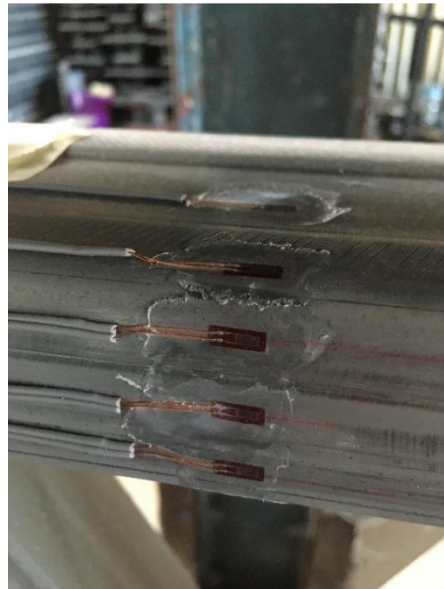
Figure 22. Strain gages attached on CFS member
