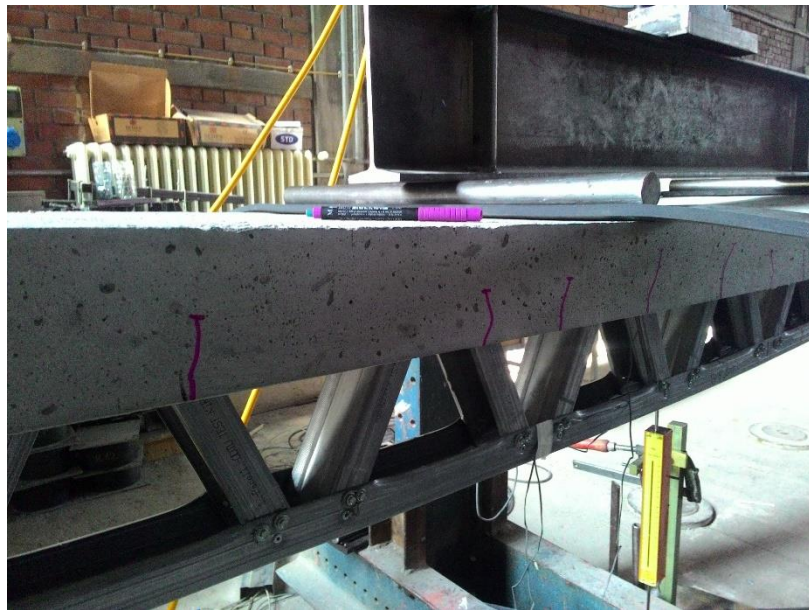
Figure 25. Concrete cracking in specimen WB_Slab
