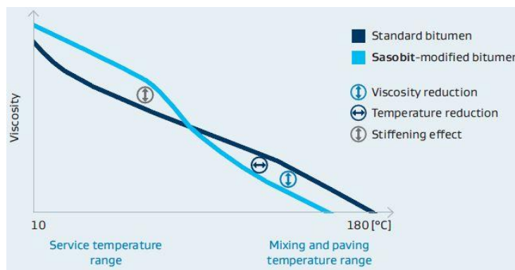
Figure 2.5 Sasobit viscosity modification (SasolPerformanceChemicals, ProductInformation_en)
