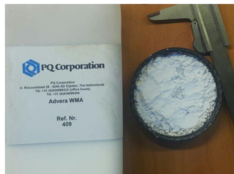
Figure 2.2 WMA foaming additive (ADVERA)
